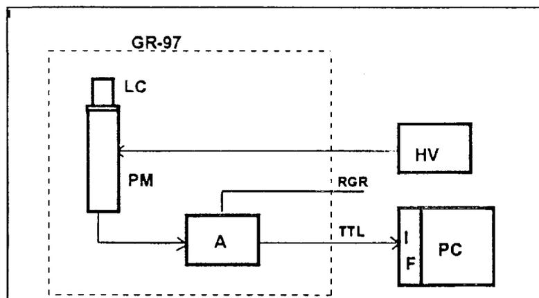
Fig. 2. Block diagram of the GR-97 measuring head for determining radon concentration: LC - Lucas cell KS-10 or KS-11, PM - photomultiplier tube EMI-966B, HV - high voltage power supply, A - low noise pulse amplifier followed by a pulse discriminator, IF - computer interface, PC - personal computer, RGR - analog pulse from amplifier output, TTL - TTL pulse from discriminator output.
