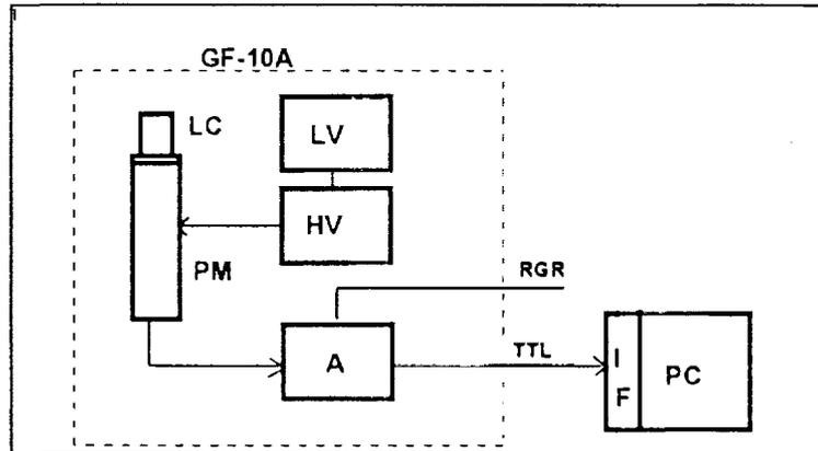
Fig. 1. Block diagram of the GF-10A measuring head for determining radon concentration: LC - Lucas cell KS-10 or KS-11, PM - photomultiplier tube FVS-300, HV - high voltage power supply, A - low noise pulse amplifier followed by a pulse discriminator, LV - low voltage (+5 V) power supply for HV, IF - computer interface, PC - personal computer, RGR - analog pulse from amplifier output, TTL - TTL pulse from discriminator output.
