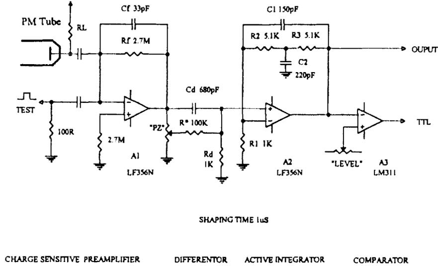
Fig. 3. Functional diagram of low noise pulse amplifier.
