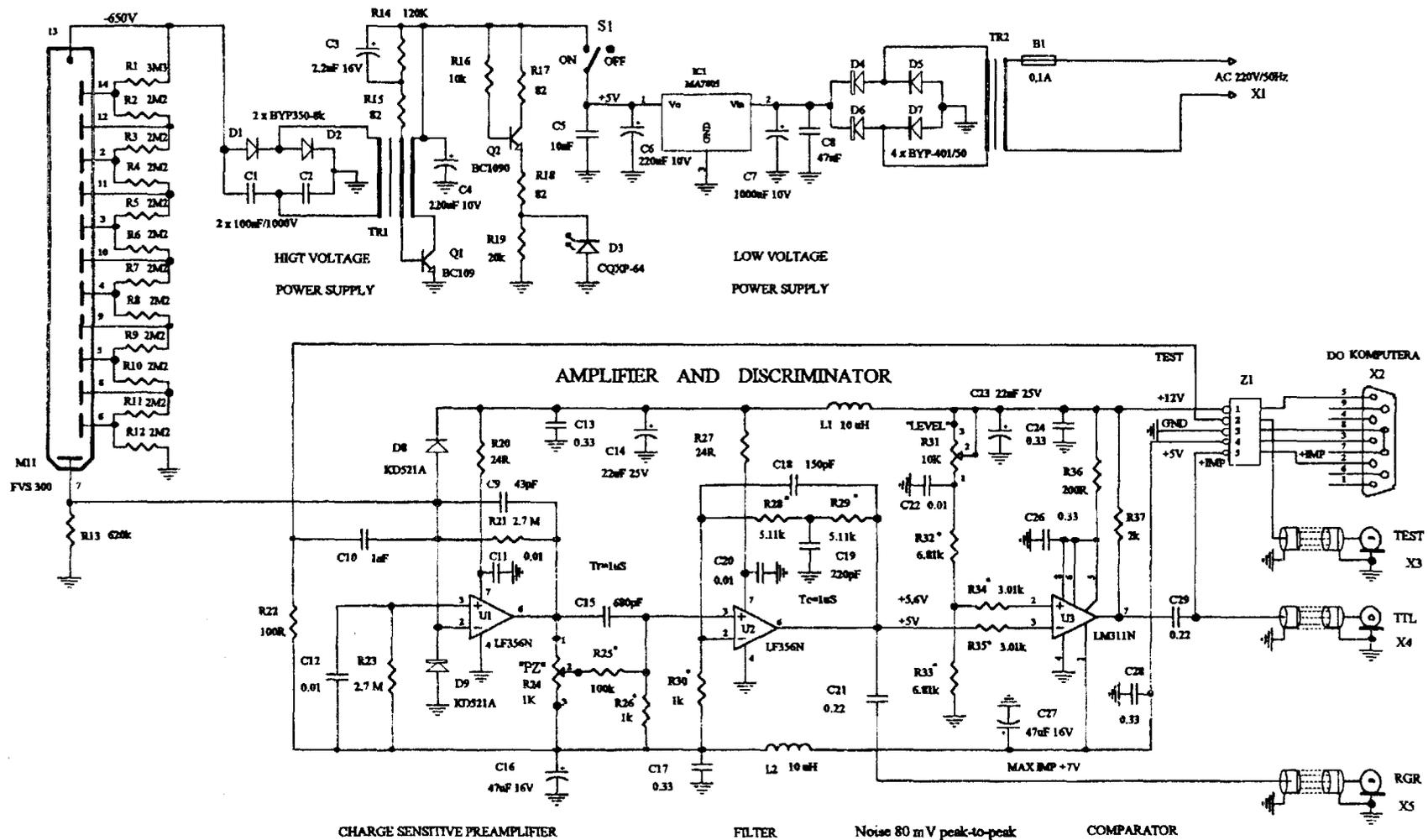
Fig. 4. Measuring head GF-10A
