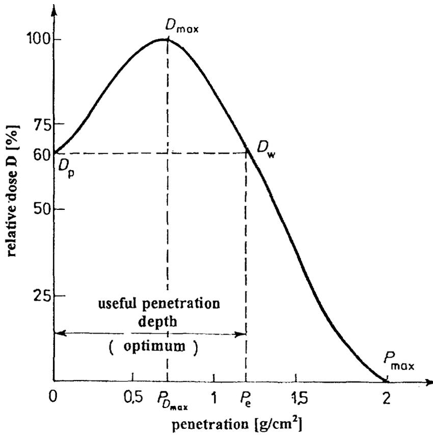
Fig. 8. Absorbed dose vs. material thickness.
