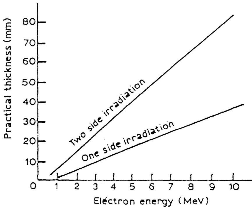
Fig.10. Practical thickness vs. electron energy. (Bulk density = 1).
