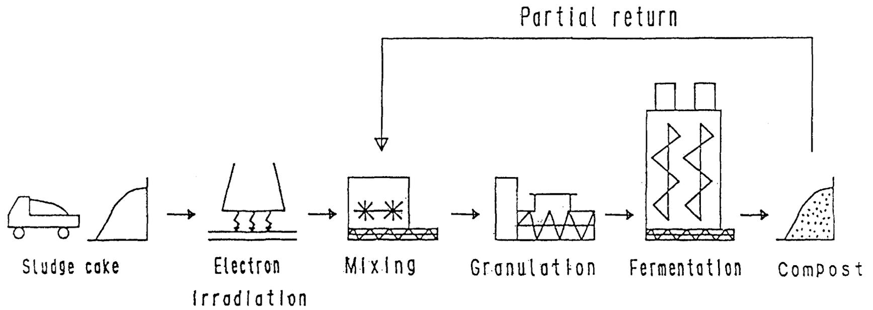
Fig.20. Flowsheet of sludge irradiation and composting [15].
