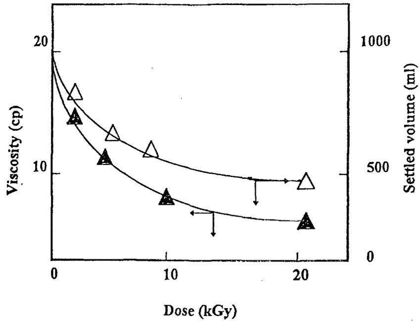
Fig. 17. Sludge settling parameters after irradiation [20].
