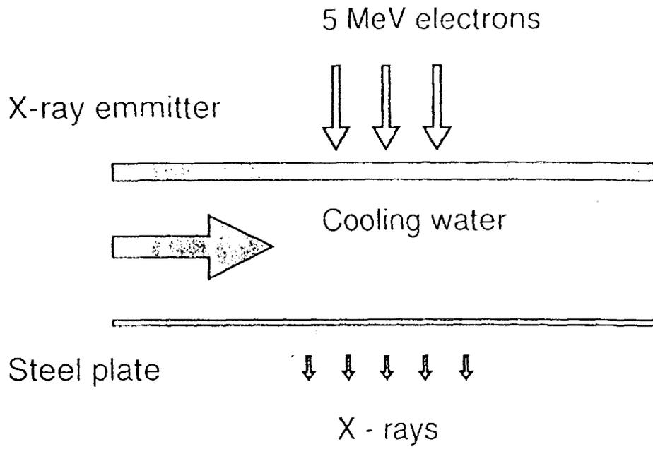
Fig.11. Structure of  $e^-/X$  converter.
