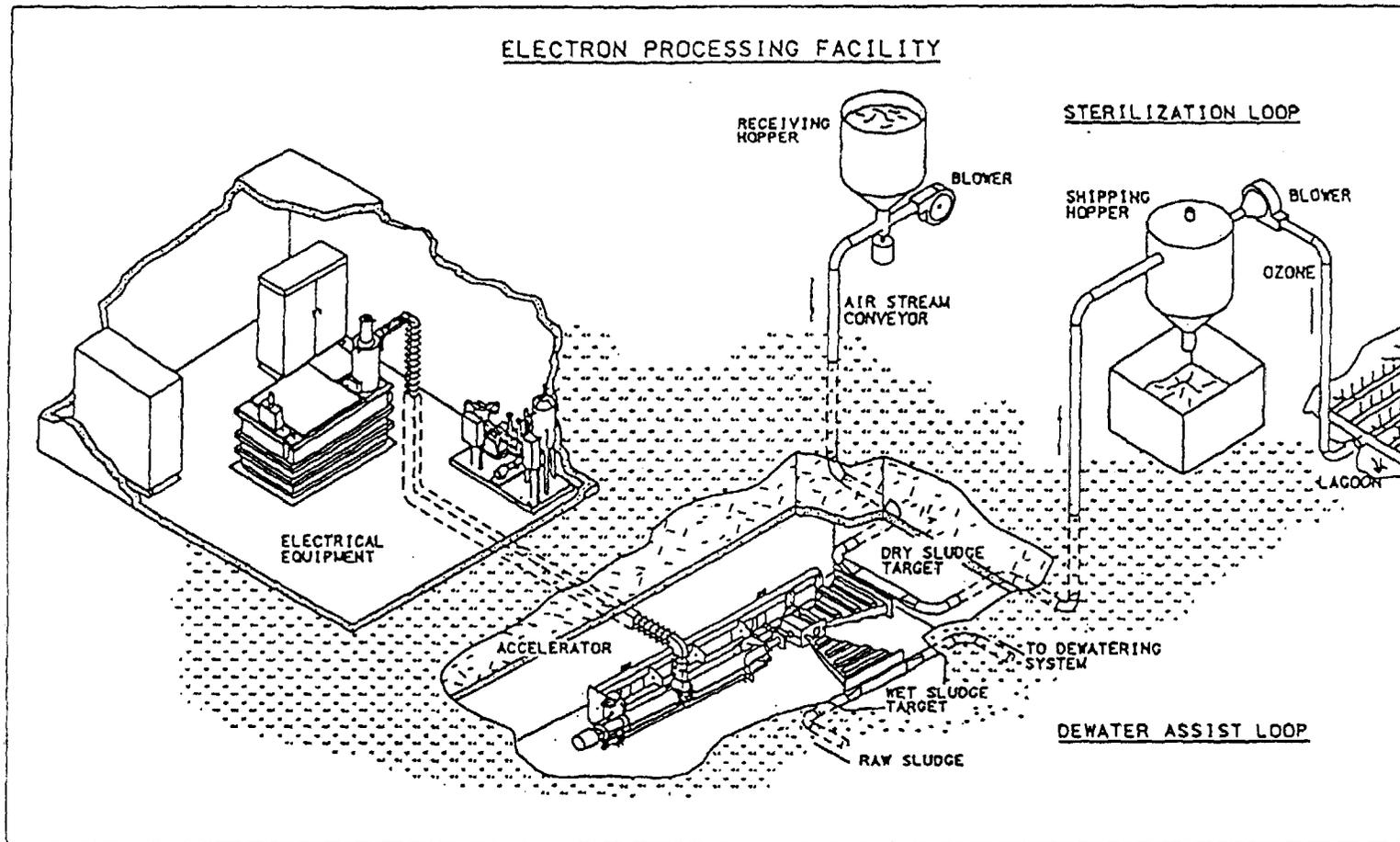
Fig. 16. Design concept of electron beam plant [19].
