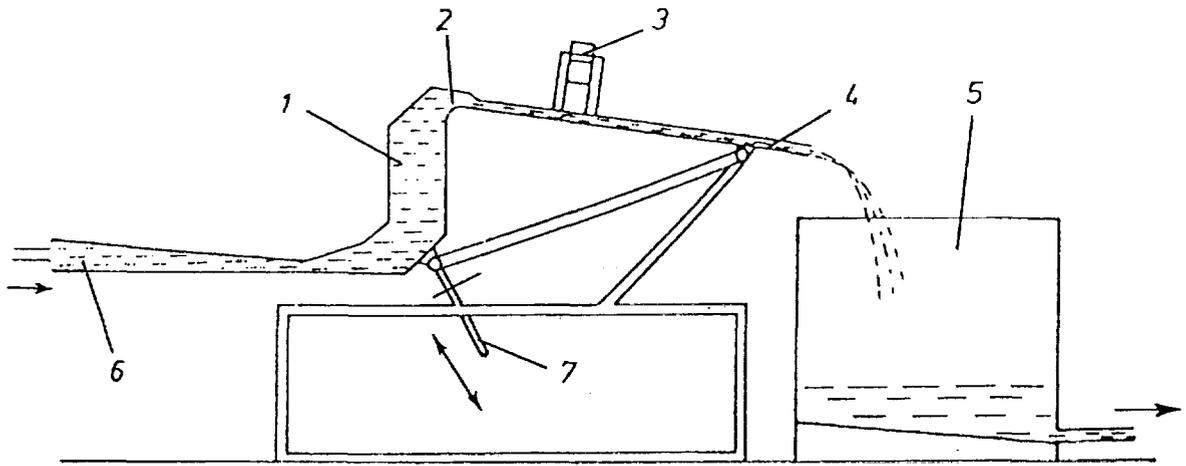
Fig. 19. Sludge irradiation system.
