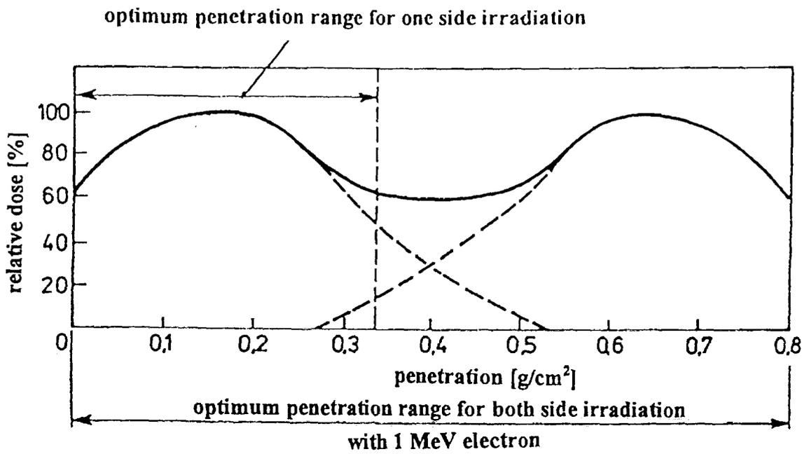
Fig.9. Two side material irradiation.
