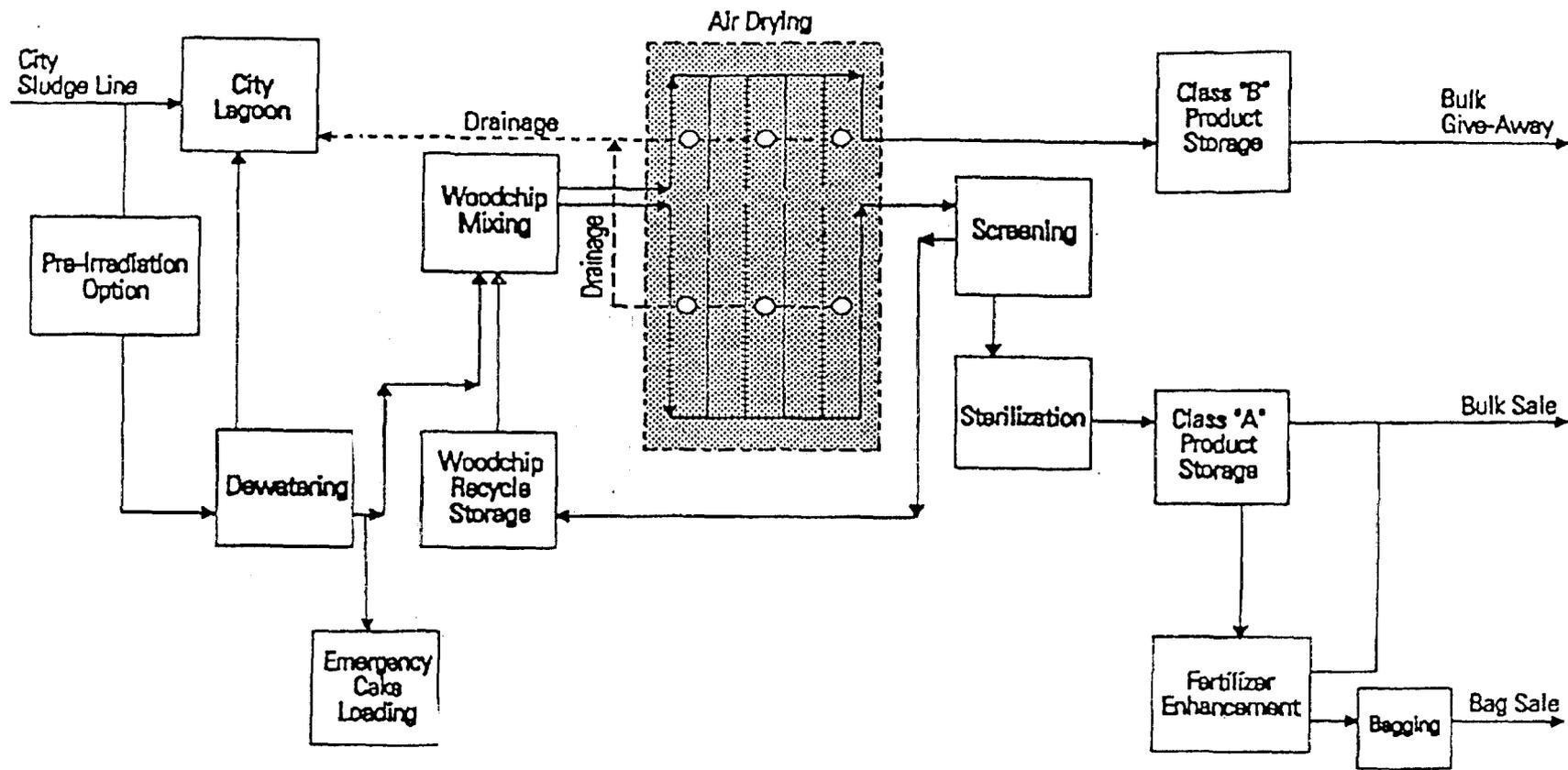
Fig. 15. Flowsheet of sludge treatment facility [19].
