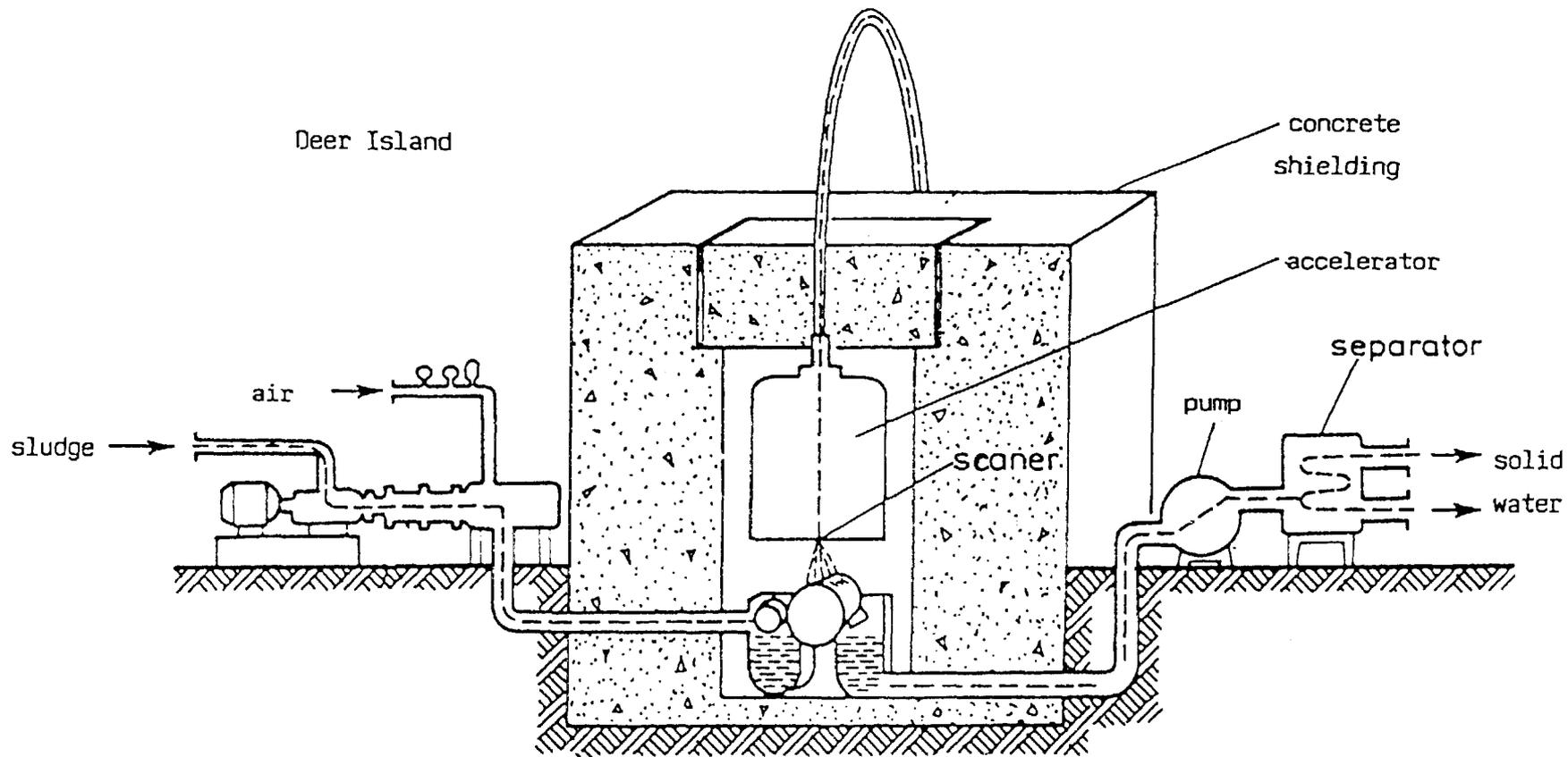
Fig.18. Sludge irradiation facility at Deer Island wastewater treatment plant.
