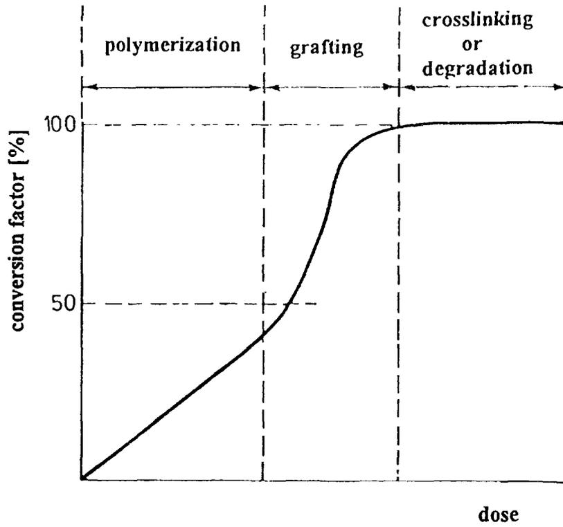
Fig. 7. Dose ranges for polymer processing.
