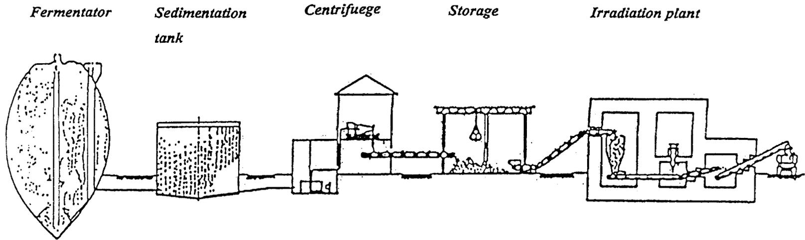
Fig. 13. Flowsheet of sludge disinfection plant [17].
