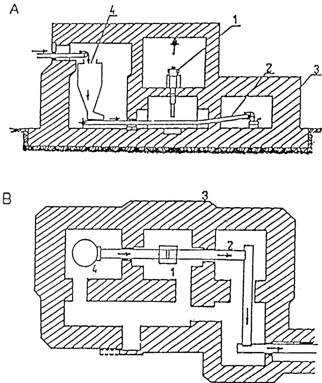
Fig. 14. Sludge irradiation facility [18]: 1 - accelerator, 2 - conveyer, 3 - shielding, 4 - tank.
