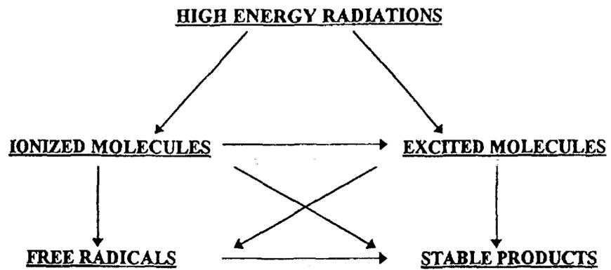
Fig.5. Radiation induced processes [6].
