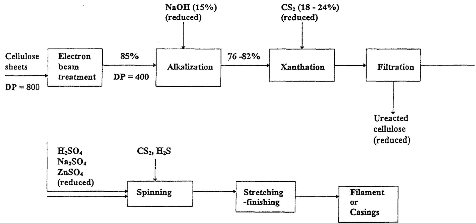
Fig.28. Viscose production process—electron beam cellulose pulp treatment
