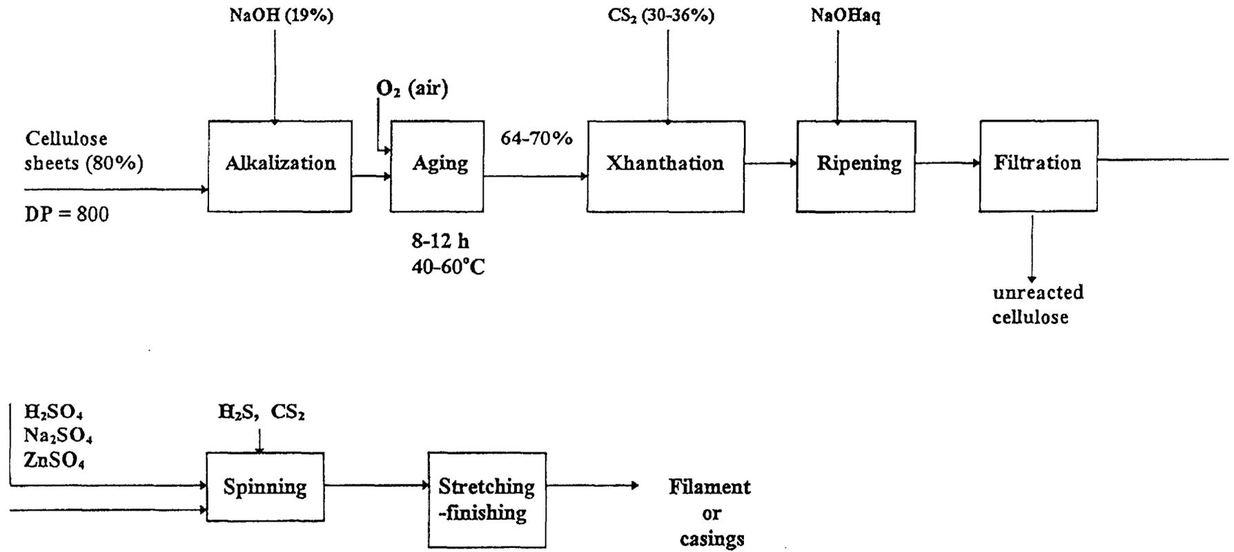
Fig.25. Viscose manufacturing process - conventional.
