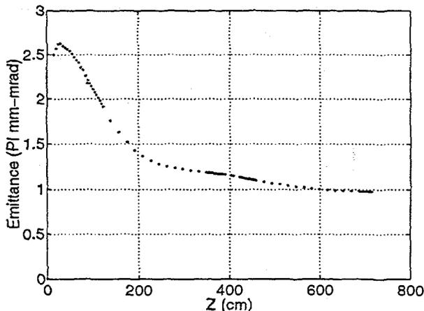
Figure 1. Parmela Simulations of Emittance Compensation with Acceleration
