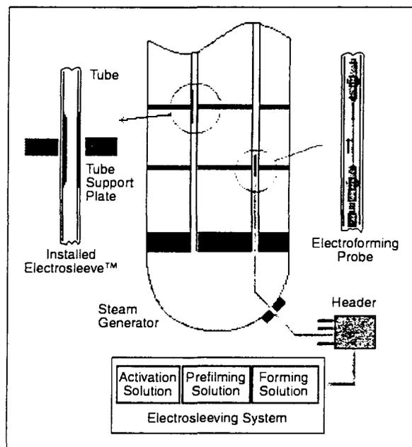
Figure 6: Simplified schematic of Electrosleeve delivery system.
