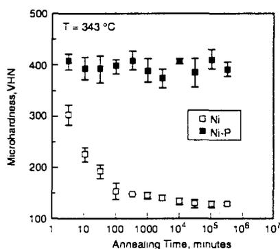
Figure 2: Vickers hardness vs. annealing time at 343 °C for nanocrystalline (1) Ni and (2) Ni-1500 ppm P.
