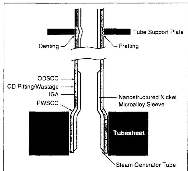
Figure 8: Electrosleeve repair of various SG degradation modes.
