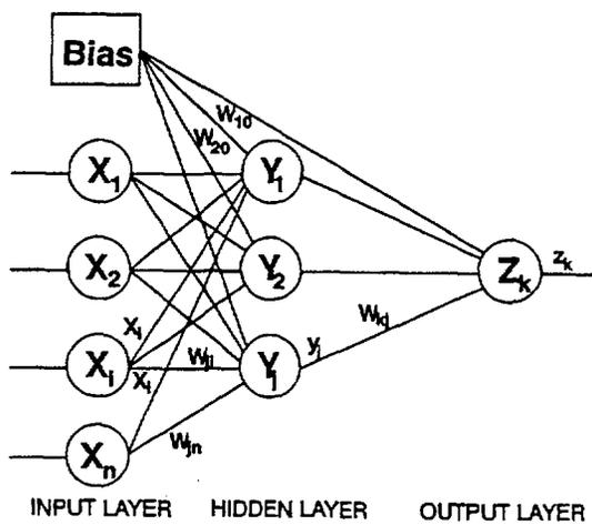
FIGURE 1. ARCHITECTURE OF A BACK PROPAGATION ARTIFICIAL NEURAL NETWORK. DESCRIPTION OF INPUT VARIABLES IN TABLE 1 AND CONNECTION WEIGHTS IN TABLE 4.
