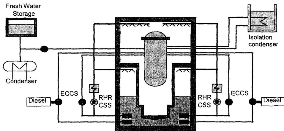
FIG. 6. Decay heat removal and coolant make-up systems.
