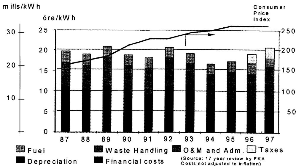
FIG. 2. Generation costs for the three BWR 75s at Forsmark
