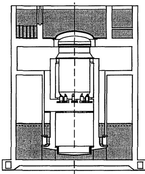
FIG. 5. Containment design for the BWR 90+
