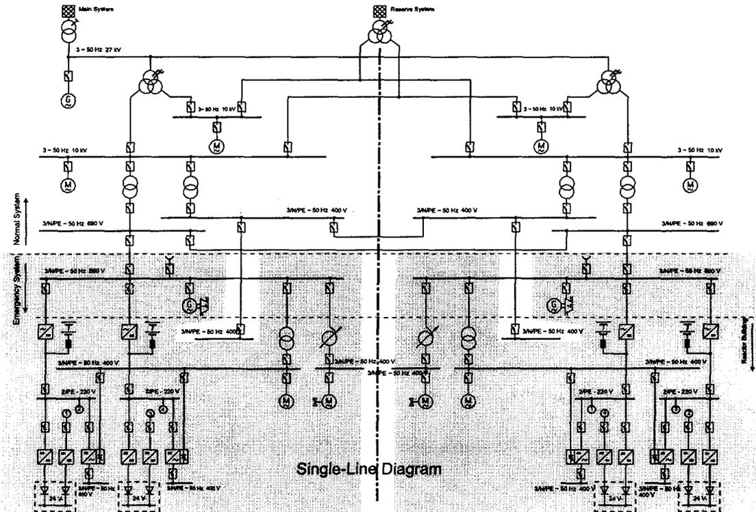
FIG. 15: Electric Power Supply Systems (Single Line Diagram)
