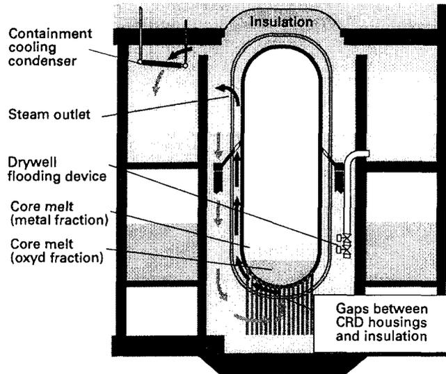
FIG. 13 Cooling of RPV Exterior in the Event of Core Melt
