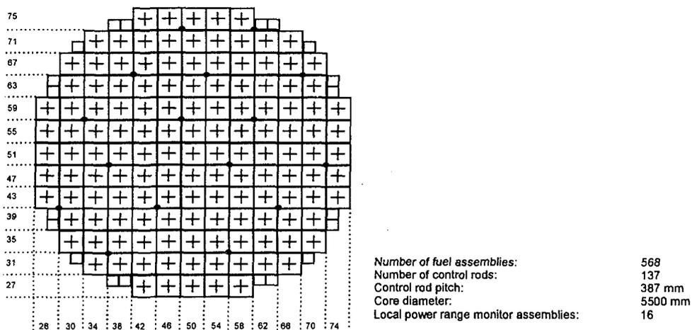
FIG. 1: Arrangement of SWR 1000 Reactor Core
