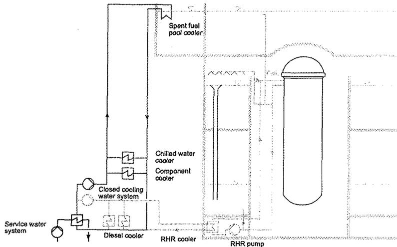
FIG. 12: Active Core Flooding and Residual Heat Removal Systems
