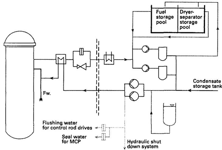
FIG. 14: Reactor Water and Fuel Pool Cleanup System
