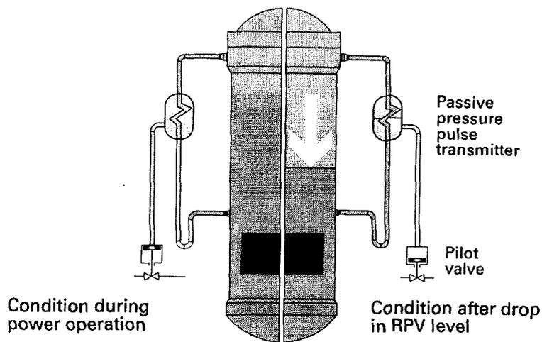
FIG. 10: Passive Pressure Pulse Transmitter
