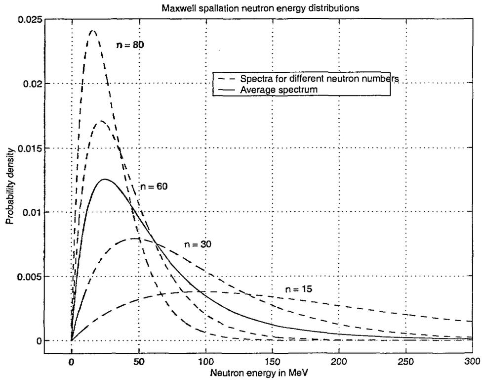
FIGURE 9. Some number dependent spectra and the average spectrum of spallation neutrons with Maxwell energy distribution.
