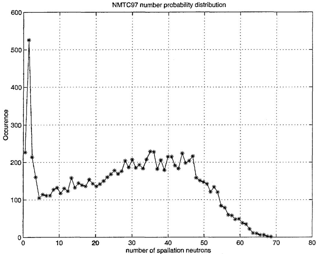
**FIGURE 3.** Number distribution of spallation neutrons calculated in a *NMTC/JAERI97* simulation where the proton energy was 3000 MeV.
