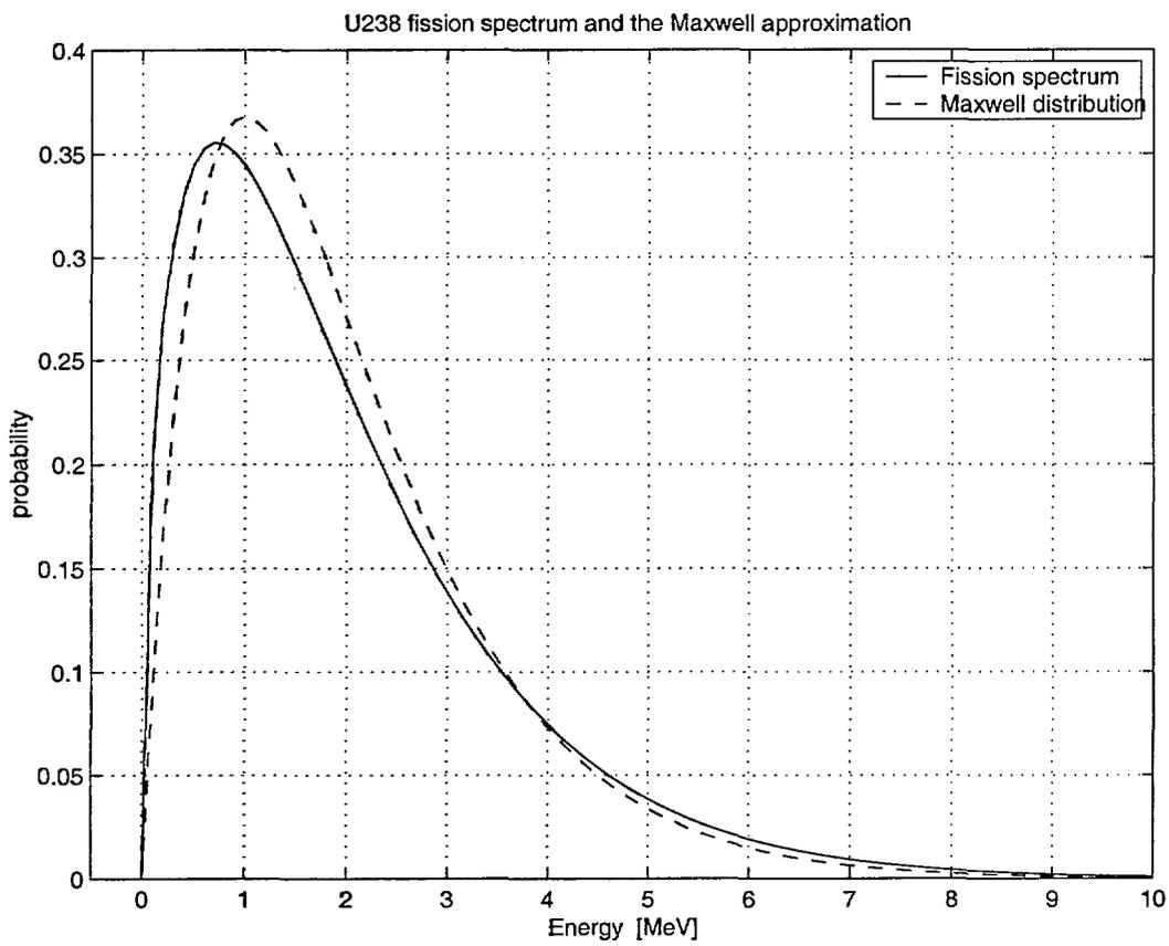
FIGURE 8. The energy distribution of neutrons generated in thermal fission of  $^{235}\text{U}$  and a Maxwell distribution that approximates the fission spectrum.
