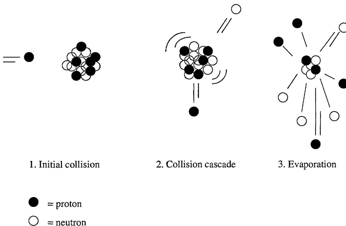
**FIGURE 1. The spallation process.**
