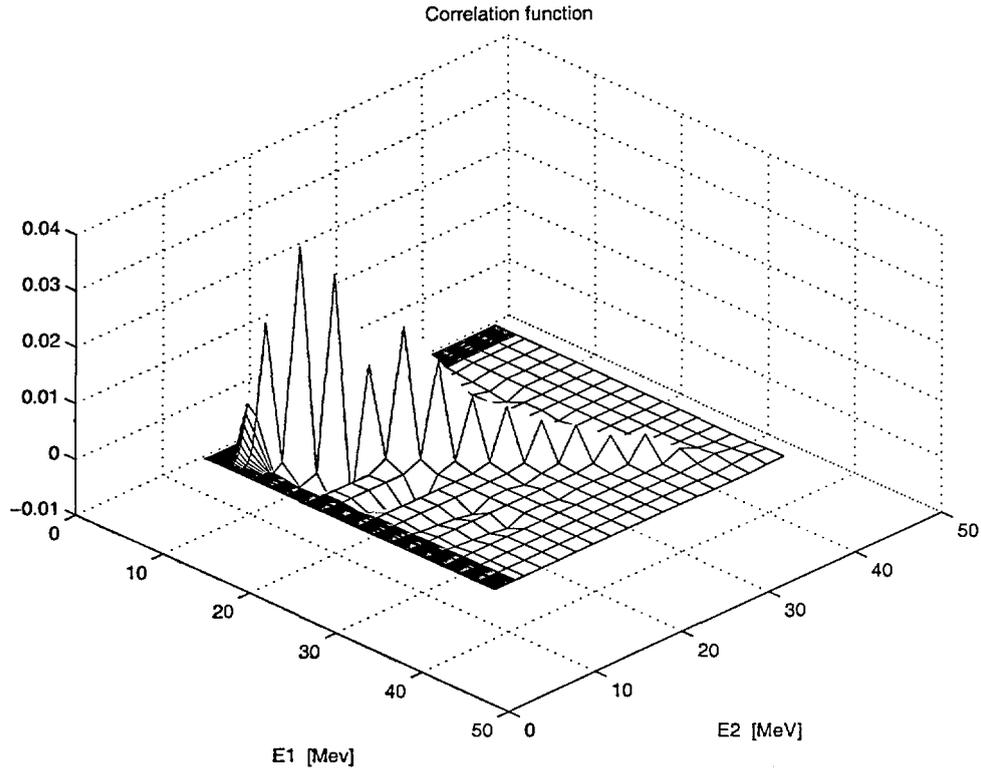
**FIGURE 7.** Two-dimensional correlation function of a Gaussian spectrum model where a standard deviation of  $\sigma = 0.6$  MeV was used.
