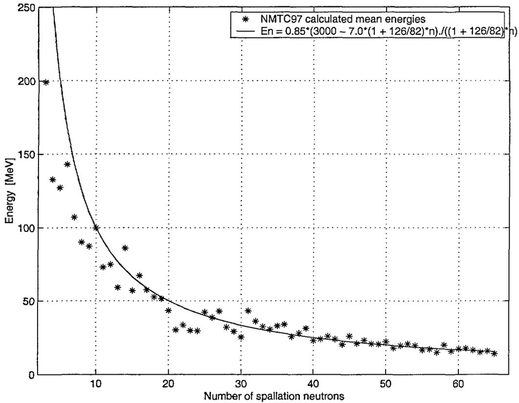
FIGURE 5. Average energies for different groups of spallation neutrons, calculated with *NMTC/JAERI97* and with (eq. 3.1).
