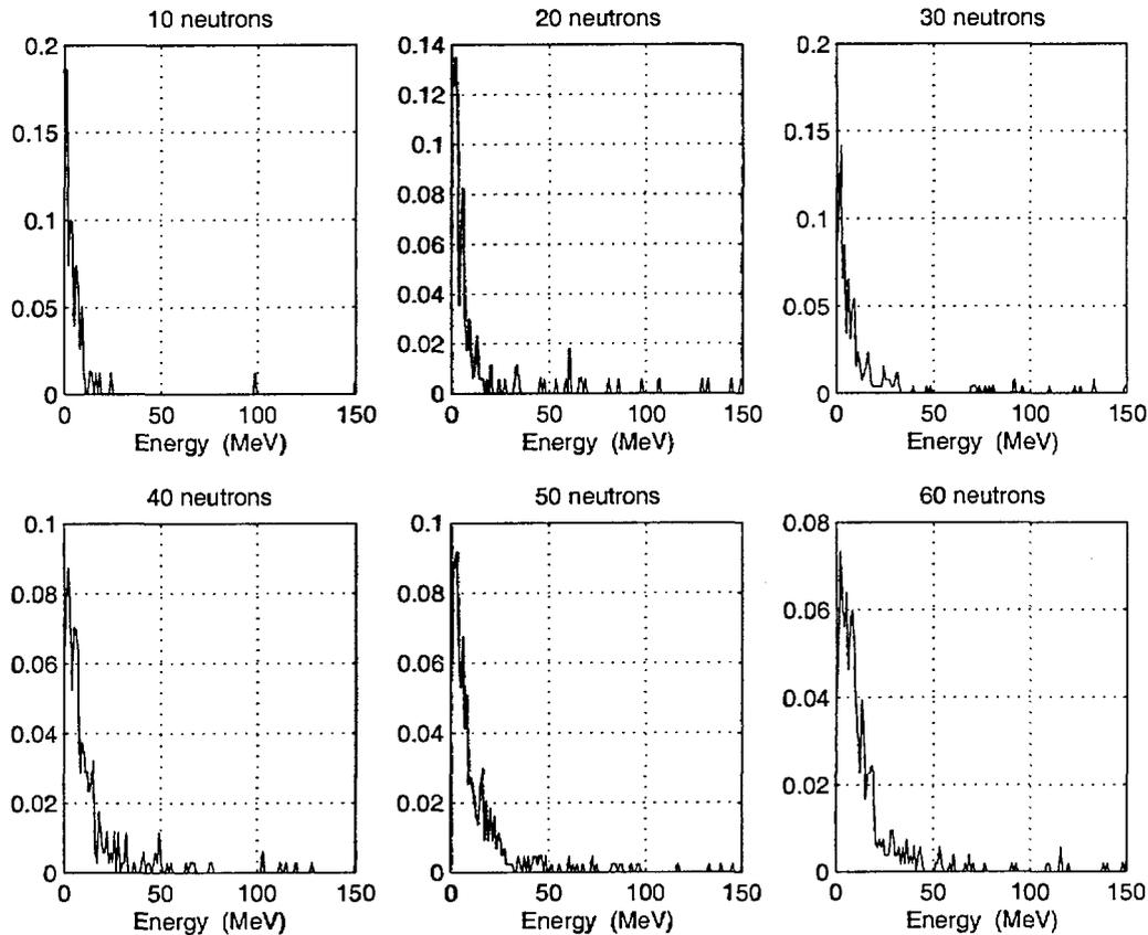
**FIGURE 4.** Energy distributions for various groups of spallation neutrons, calculated in a *NMTC/JAERI97* simulation where the proton energy was 3000 MeV.
