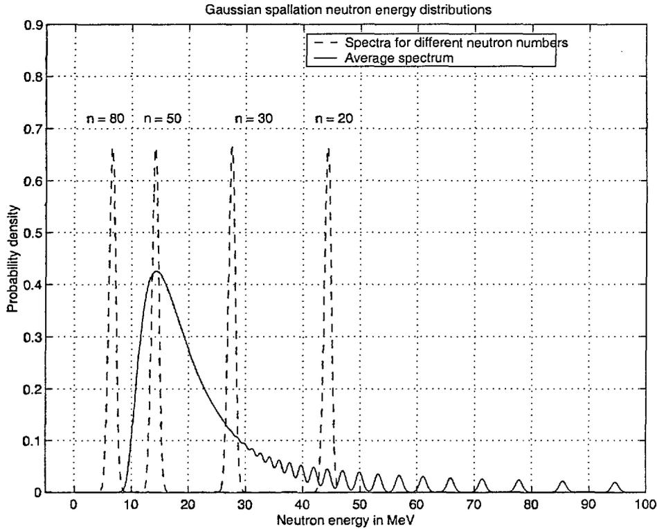
**FIGURE 6.** Some number dependent spectra and the average spectrum of spallation neutrons with Gaussian energy distribution. A standard deviation of  $\sigma = 0.6$  MeV was used.
