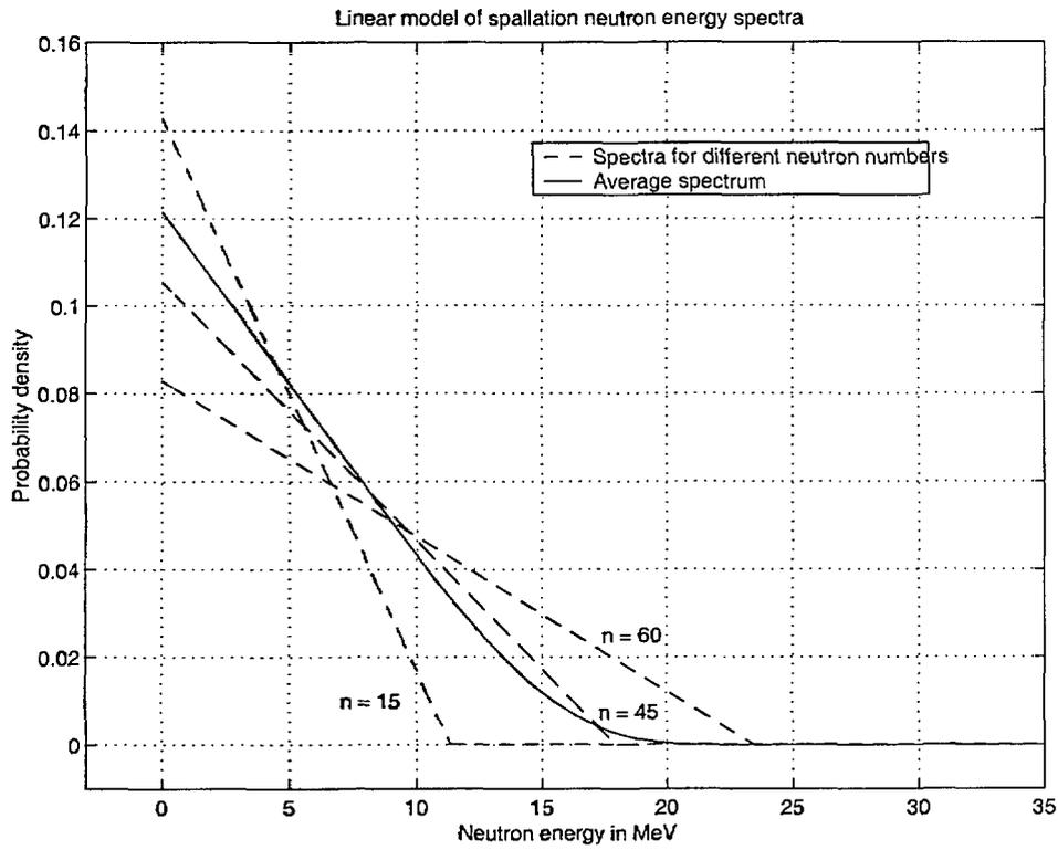
**FIGURE 11. Some number dependent spectra and the average spectrum of spallation neutrons with a piece-wise linear energy distribution, modelling spectra that were calculated by NMTC/JAERI97 for a case where the proton energy was 3000 MeV.**
