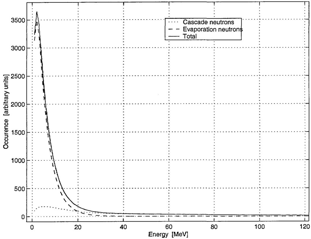
FIGURE 2. Energy distribution of spallation neutrons ejected through collision cascades and evaporation.
