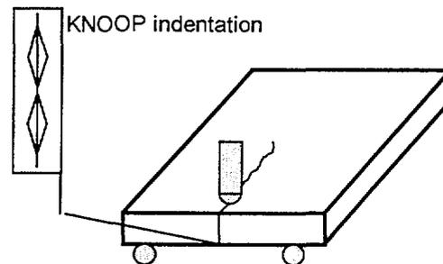
FIG. 3. Double torsion test
