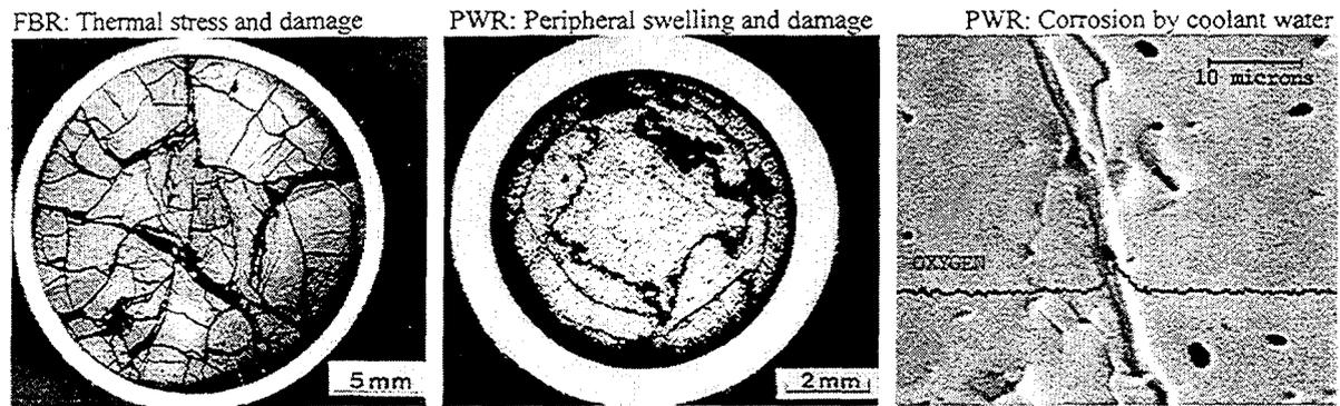
FIG. 1. Damage modes of pellets during irradiation
