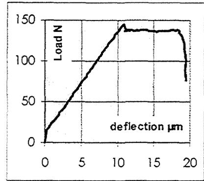
FIG. 5. Brittle homogeneous material
