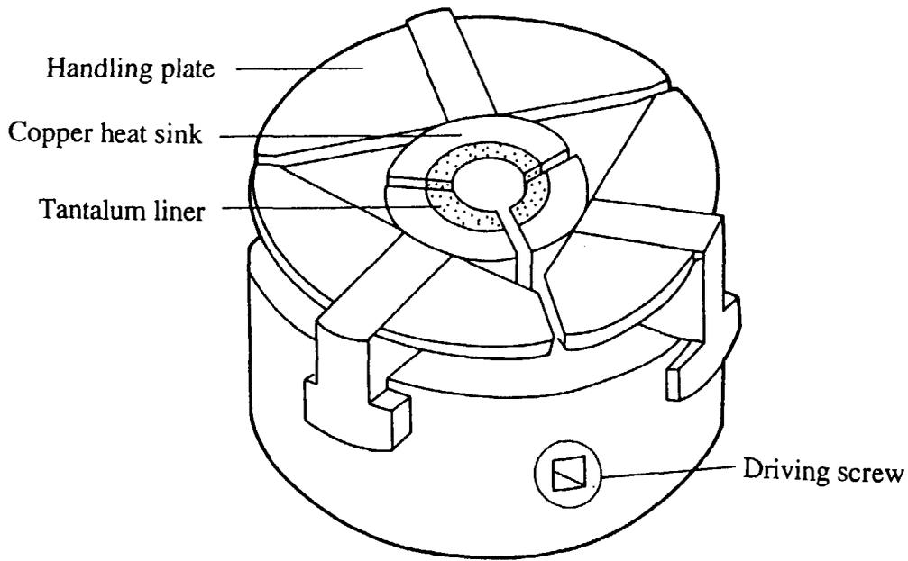
Fig. 1 Structure of the capsule chuck in an electron beam welder
