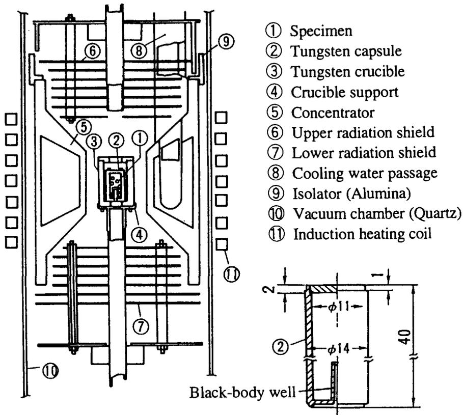
Fig. 3 A schematic drawing of the induction furnace unit and a tungsten capsule
