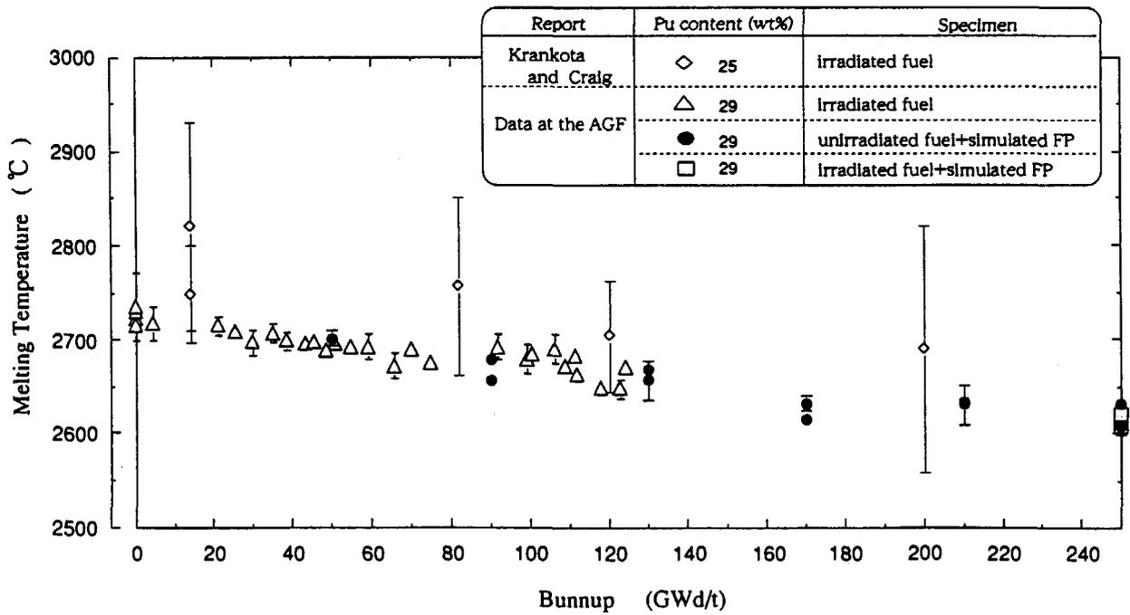
Fig. 4 Melting temperature of MOX fuels as a function of burnup
