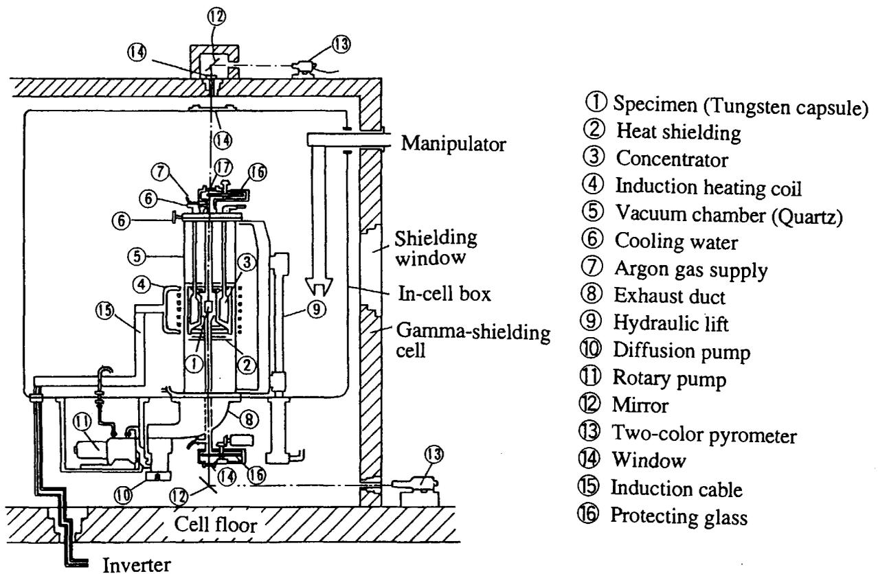
Fig. 2 A schematic drawing of the melting temperature measurement apparatus
