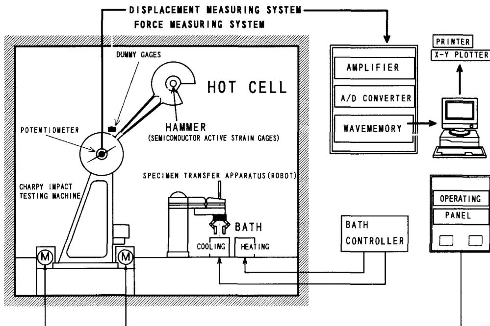
Fig.1 Block diagram of instrumented Charpy impact testing machine
