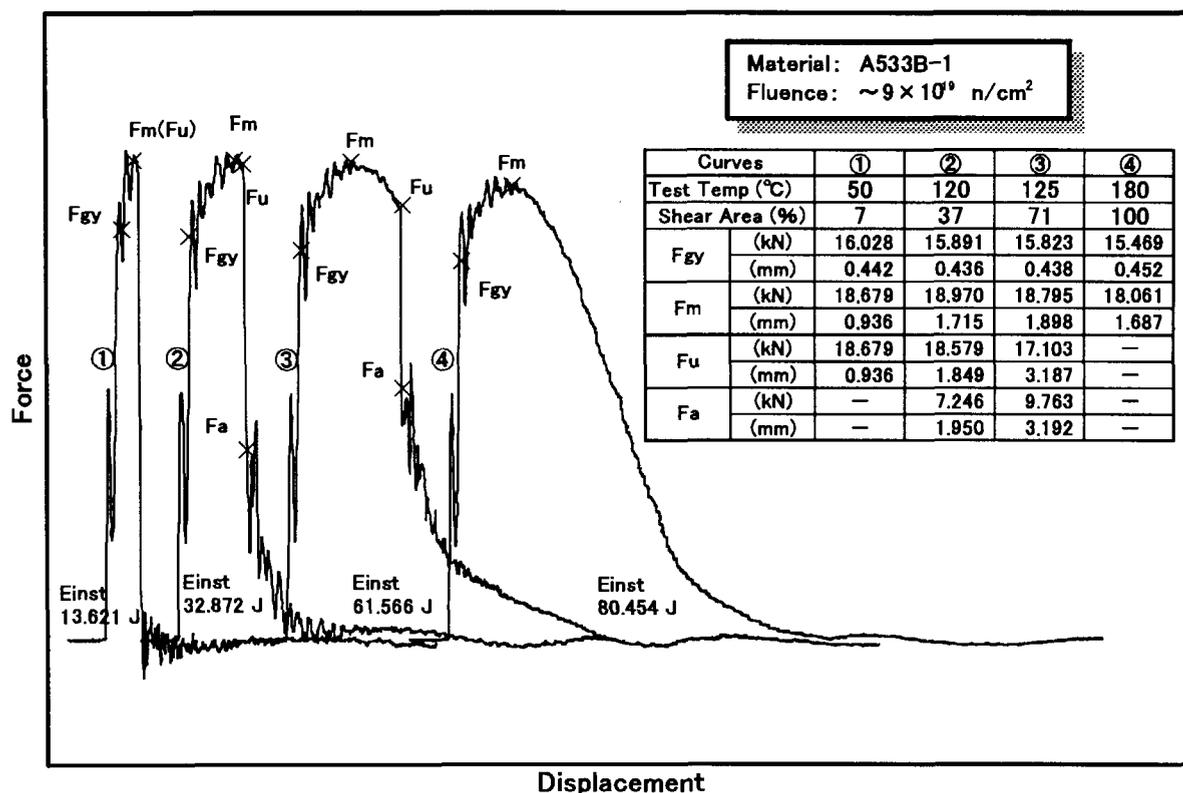
Fig.4 An example of PIE data obtained from remodeled Charpy impact testing machine
