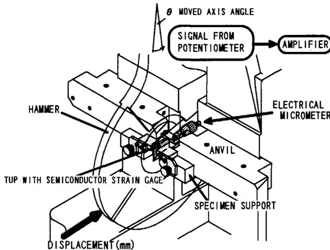
Fig. 3 Displacement calibrator
