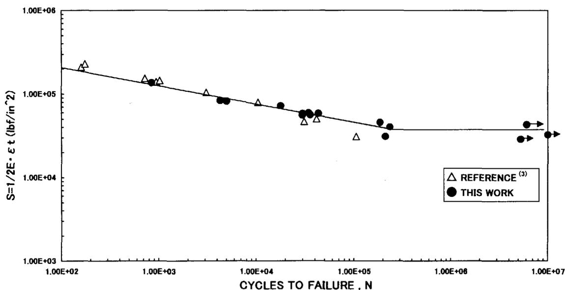
Fig.7 Fatigue data on unirradiated Zry-2 (at room temp.)
