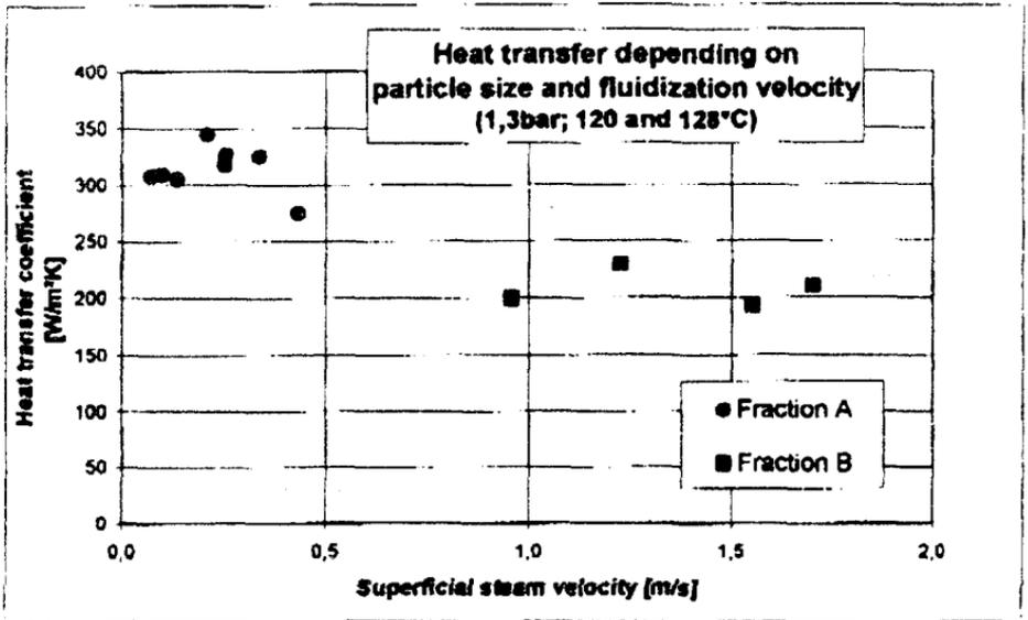
Figure 3: Heat transfer coefficients depending on particle size
