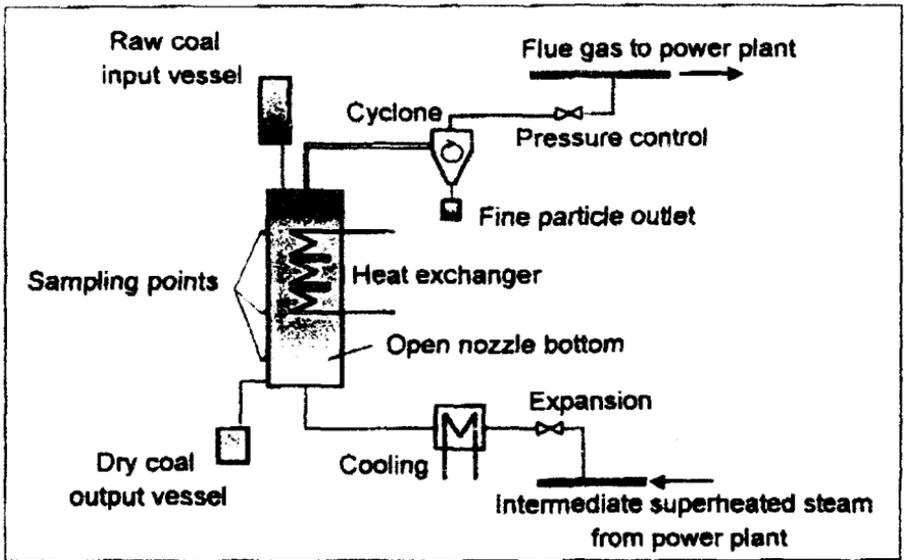
Figure 1: Flow scheme of the test dryer
