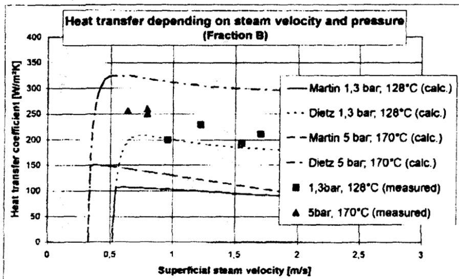
Figure 6: Heat transfer coefficient depending on pressure
