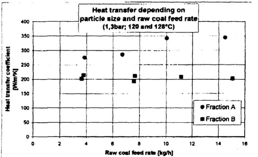
Figure 5: Heat transfer coefficient depending on raw coal feed rate
