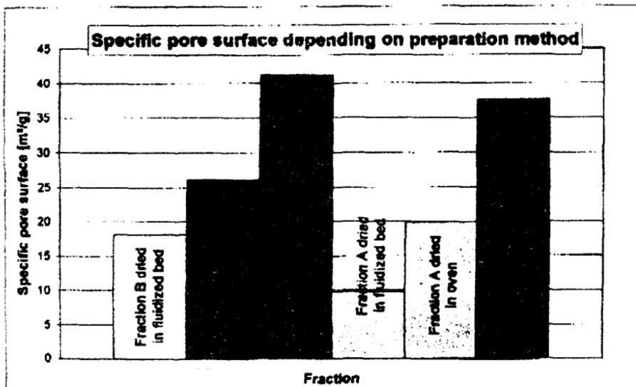
Figure 8: Pore surfaces depending on different preparation methods
