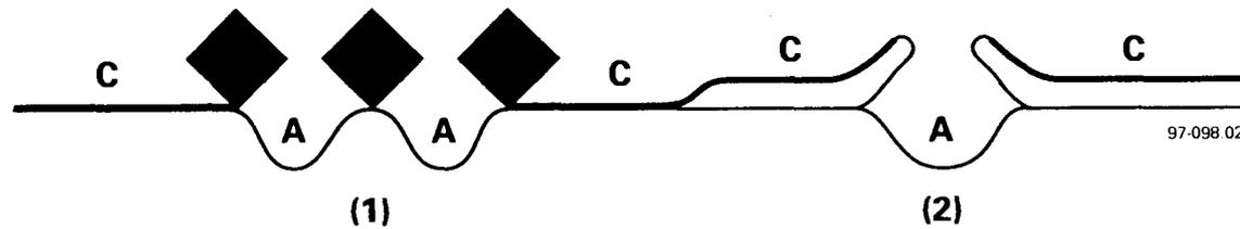
FIGURE 2: Schematic Illustrating the Possible Formation of Localized Corrosion Cells in the Event of Surface Wetting. Anodic sites (A) will tend to form in areas to which the supply of O is restricted, such as (1) underneath precipitated deposits or (2) within the pores and cracks in partially spalled corrosion products. Anodic dissolution at these sites is supported by O<sub>2</sub> reduction on exposed cathodic sites (C).
