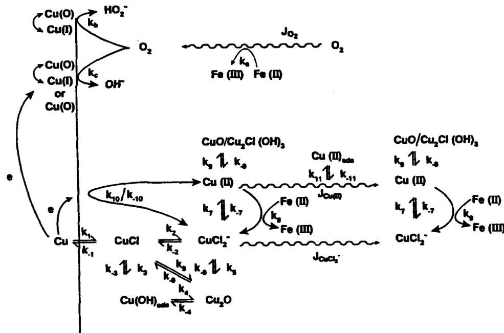
FIGURE 4: Reaction Mechanism Used to Model Aqueous Corrosion in Saturated and Unsaturated Disposal Vaults (King and Kolář 1995)
