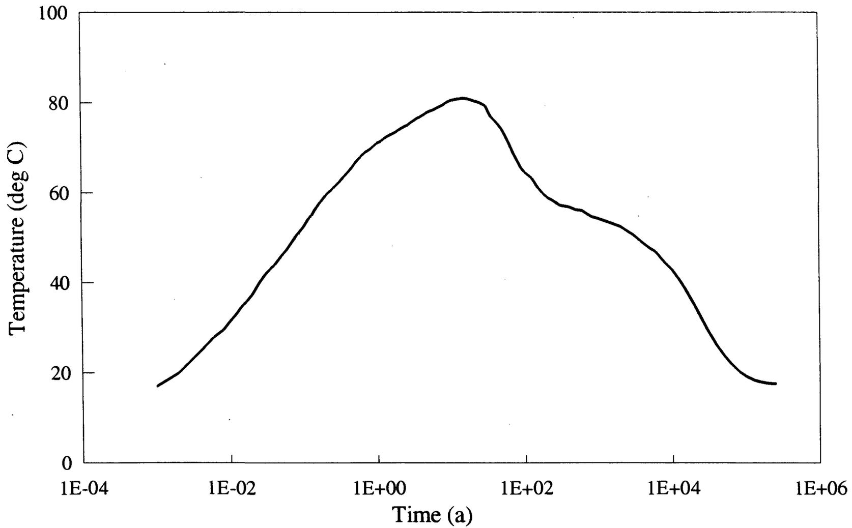
FIGURE 3: Predicted Variation of the Container Surface Temperature with Time for the In-room Disposal Configuration (Baumgartner et al. 1995)
