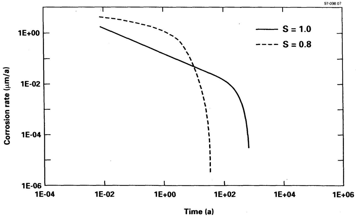
FIGURE 7: Predicted Corrosion Rate of Copper Container at 25°C in a Saturated Disposal Vault ( $S = 1.0$ ) and for a Container Covered by a Thin Liquid Film ( $S = 0.8$ ). Degree of saturation ( $S$ ) = 0.8 (broken curve) and 1.0 (solid curve).
