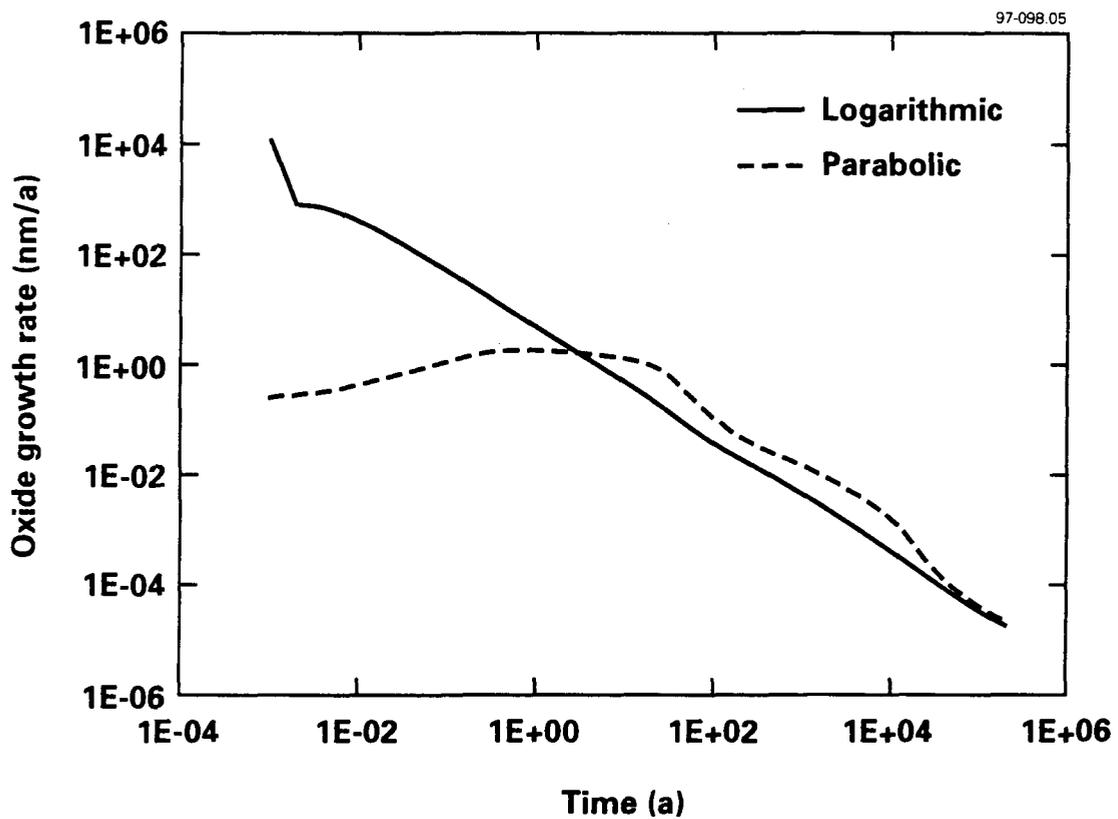
FIGURE 5: Predicted Oxide Growth Rate on Dry Container Surface for Logarithmic and Parabolic Kinetics. Logarithmic (Roy and Sircar 1981) solid curve, parabolic (Pinnel et al. 1979) broken curve.
