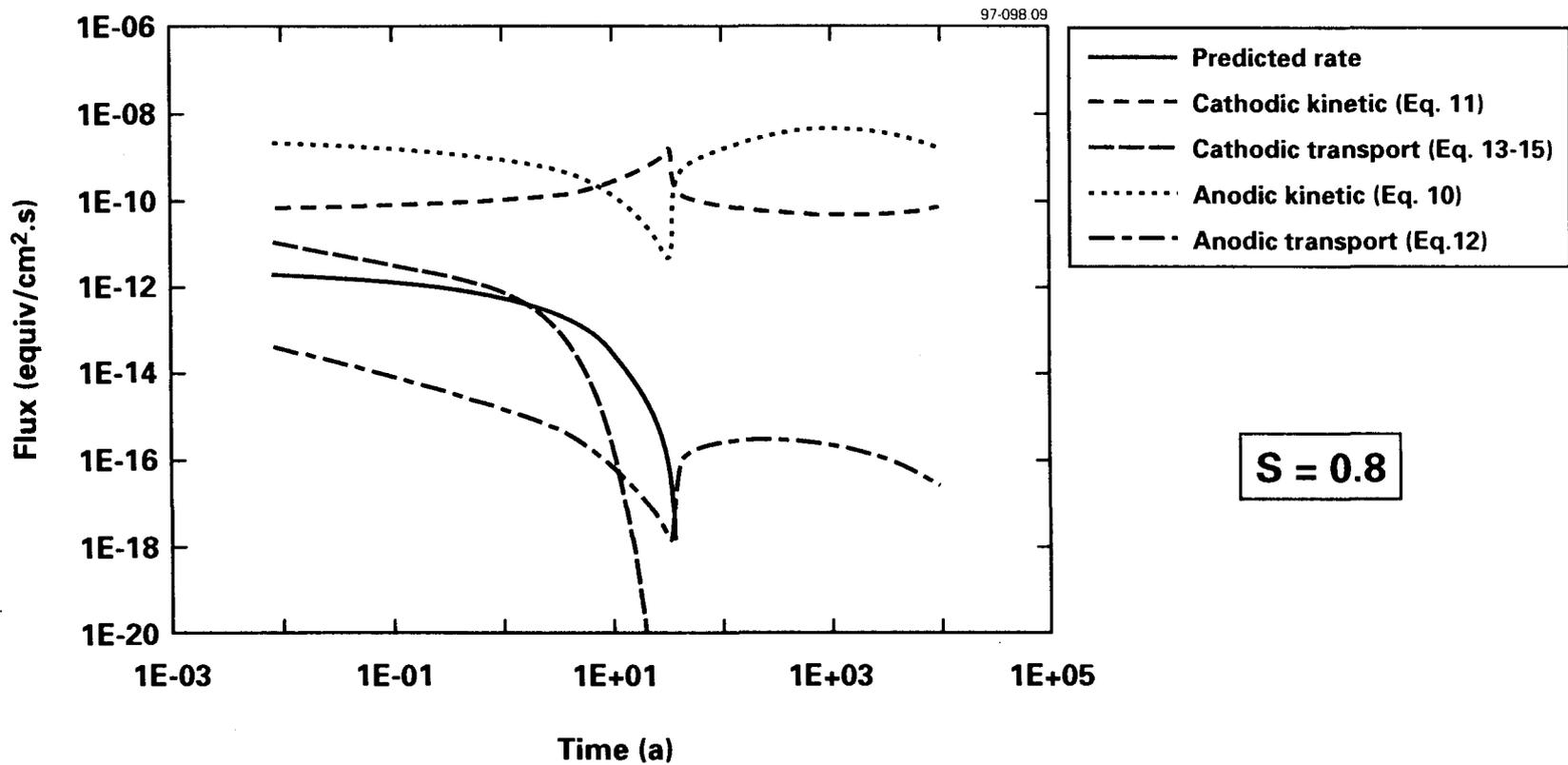
FIGURE 9: Comparison of Predicted Corrosion Rate and Rates of Four Possible Rate-determining Steps for the Uniform Corrosion of Copper Containers in an Unsaturated Disposal Vault ( $S = 0.8$ ).
