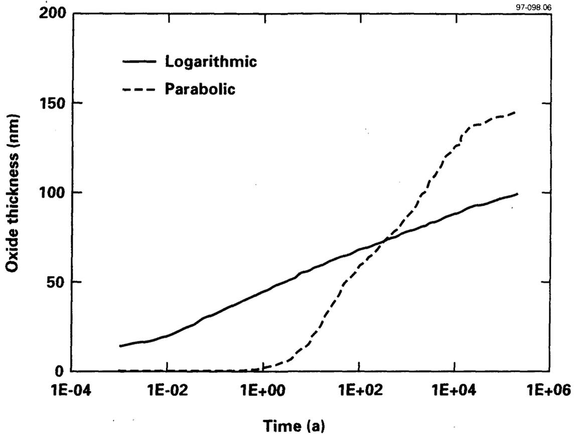
FIGURE 6: Predicted Oxide Thickness as a Function of Time for Logarithmic and Parabolic Kinetics. Logarithmic (Roy and Sircar 1981) solid curve, parabolic (Pinnel et al. 1979) broken curve.
