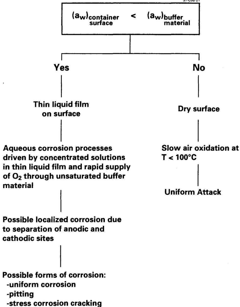
FIGURE 1: Schematic Illustrating the Corrosion Consequences of Surface Wetting
