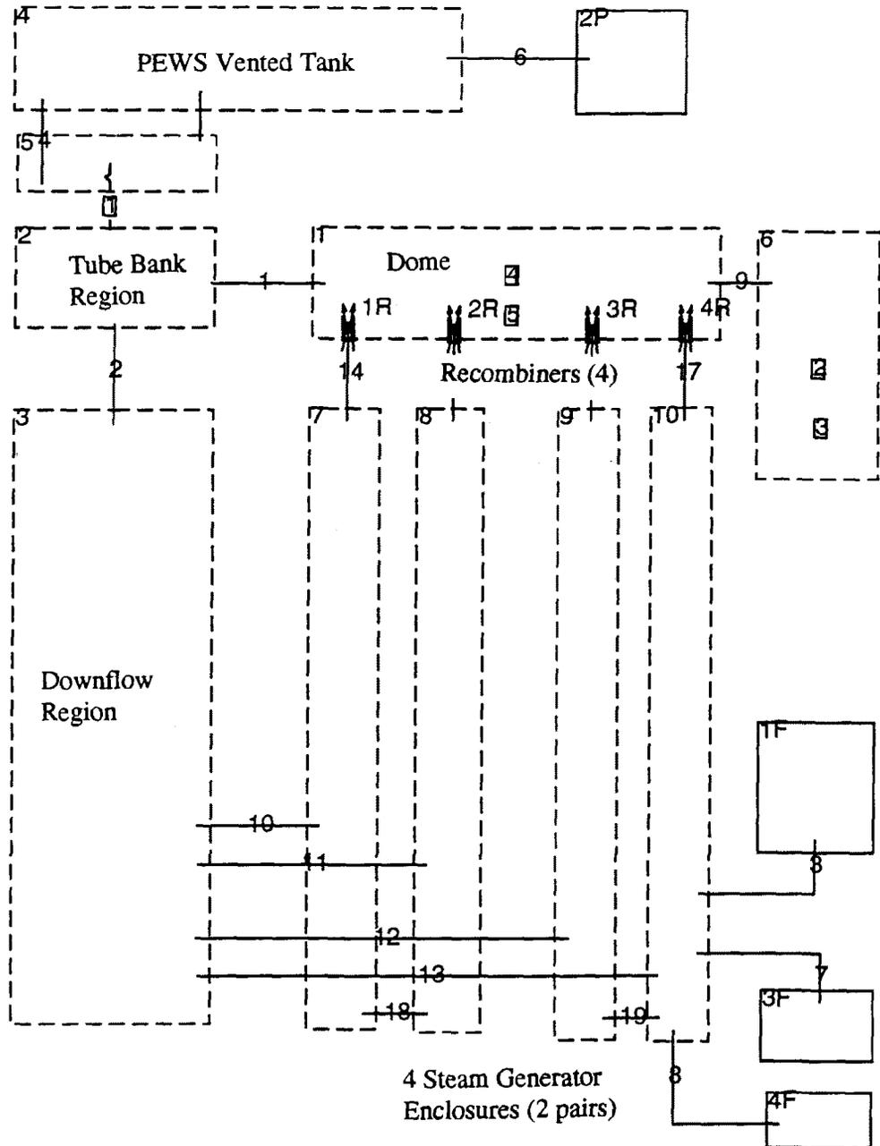
Figure 2. GOTHIC Model of Passive CANDU Containment
