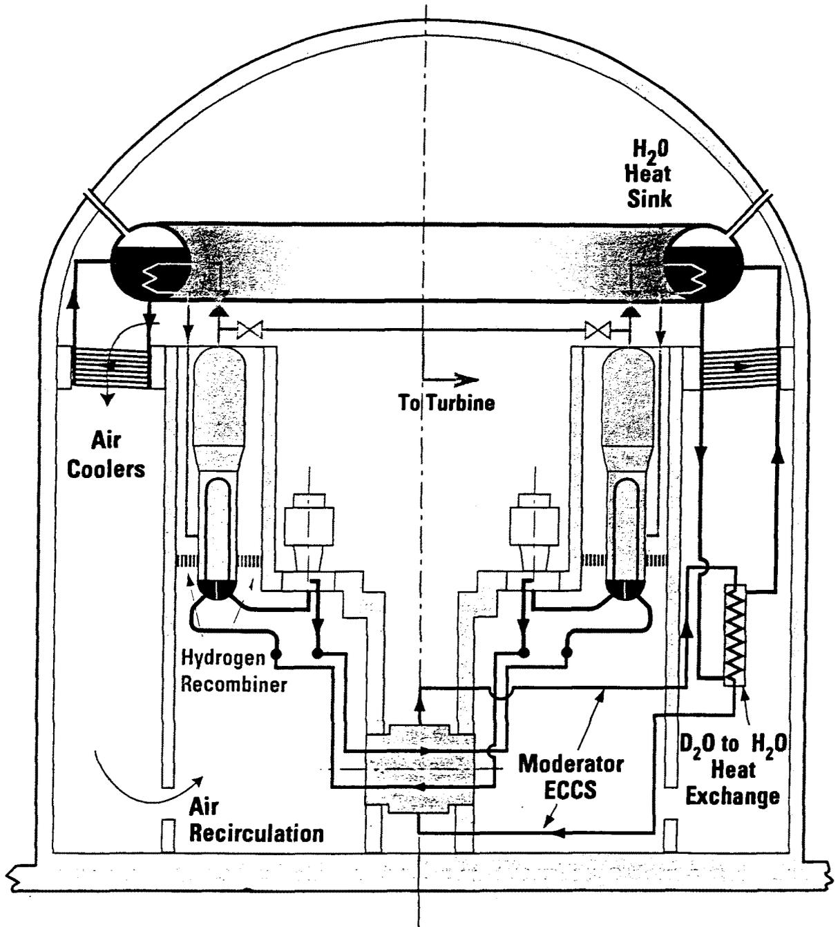
Figure 1. CANDU Containment with Passive Emergency Water System
