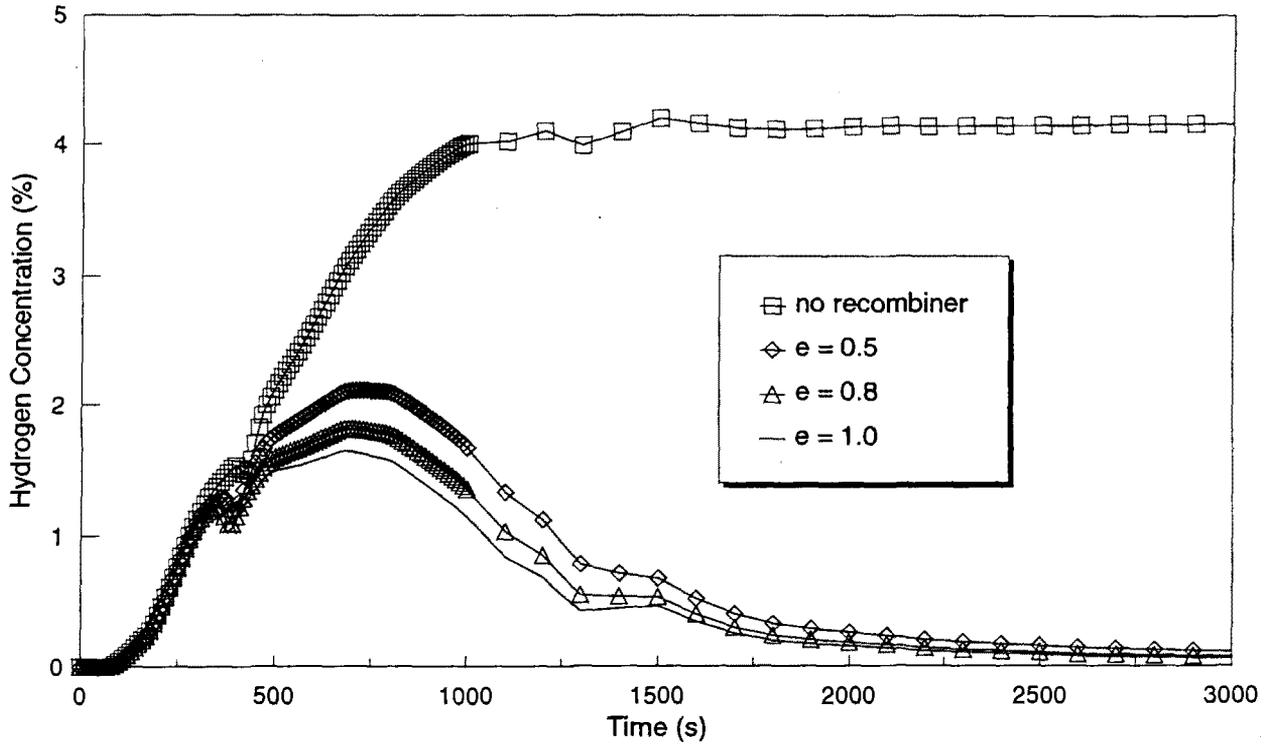
**Figure 5. Fuelling Machine Vault Hydrogen Concentration with Various Recombiner Efficiencies**
