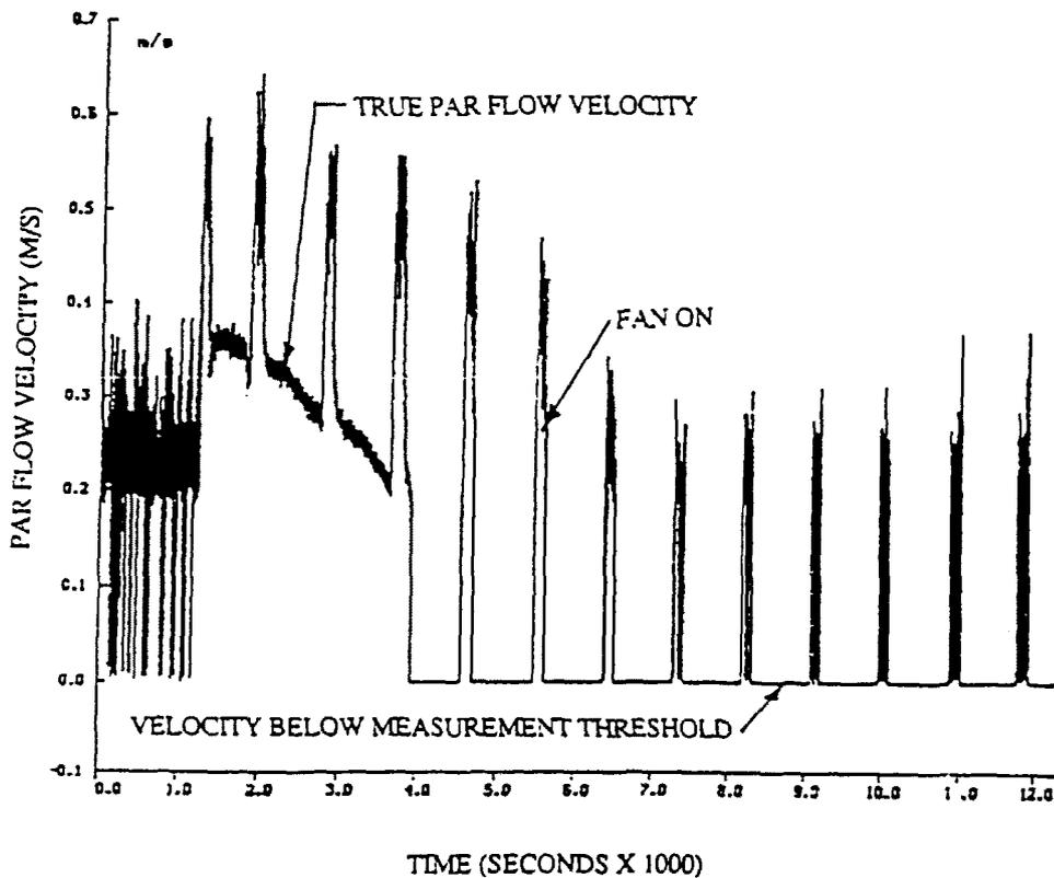
Figure 7 PAR Flow Velocity History (Test S5)
