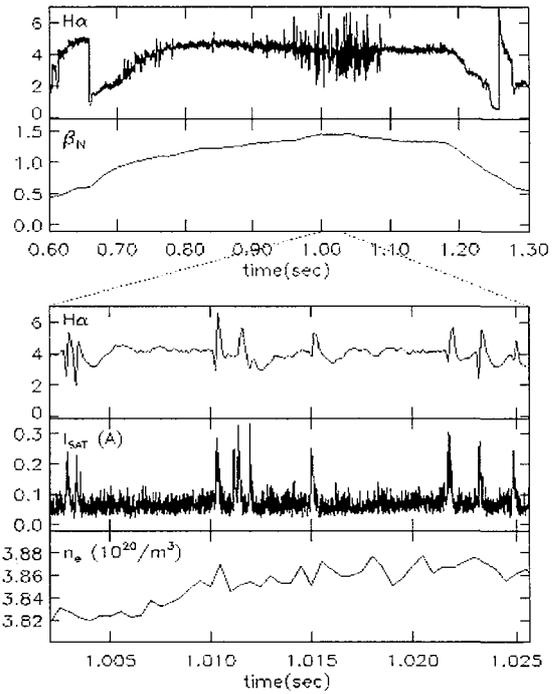
Fig 2. As  $\beta_N$  rises above 1.2-1.3 small ELMs appear on top of the EDA. Also shown on an expanded time scale is  $H\alpha$ , the ion saturation current from a divertor probe and the line averaged density. While some plasma exhaust is clearly visible on the probes, there is no measurable loss of particles from the plasma.
