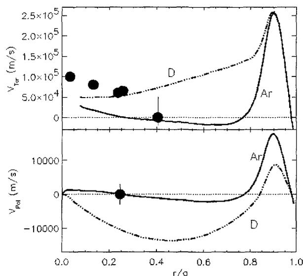
Fig. 6. Calculated toroidal (top) rotation velocity profiles for argon ions (solid) and deuterons (dash-dot-dot-dot) and poloidal rotation velocity profiles (bottom) for an ELM-free ICRF H-mode discharge. The filled circles show the measured argon toroidal and poloidal rotation velocities
