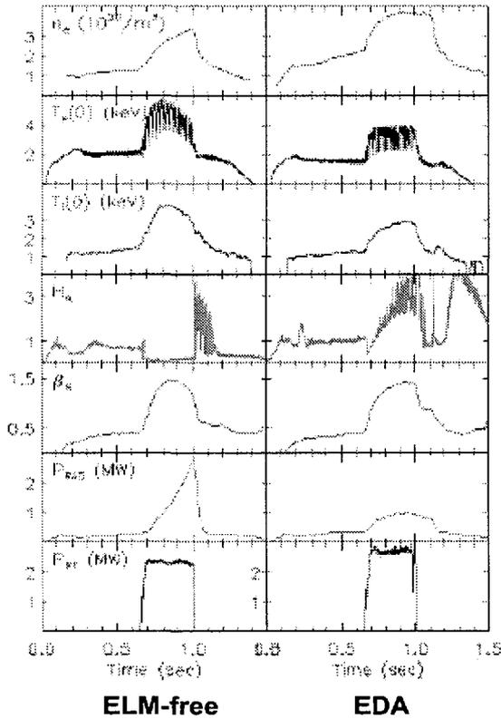
Fig 1. Characteristic traces from ELM-free and EDA H-modes. Note the difference in the  $H\alpha$  and  $P_{RAD}$  signals. The controlling difference between these shots is the target density, which is higher for EDA.
