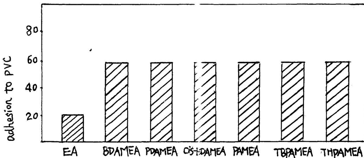
Figure 1 Adhesion to PVC of the cured films.
