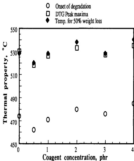
Fig.1: Thermal stabilities of EPDM formulations containing 45 phr of HAF-carbon black, different concentrations of coagent type SR-633, 1 phr of antioxidant and irradiated to 150 kGy.
