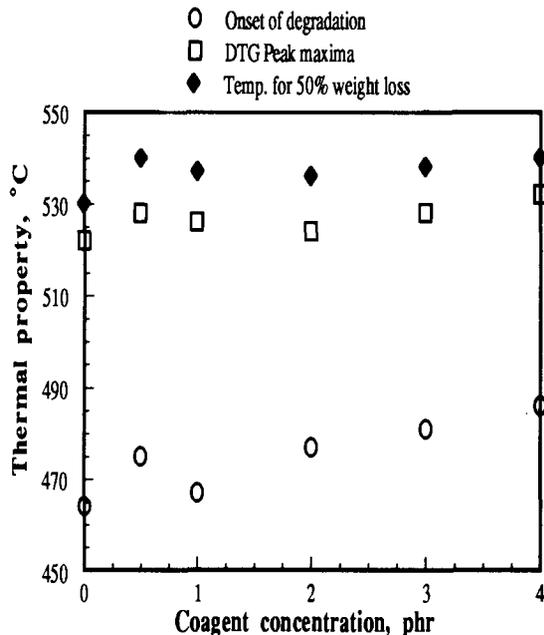
Fig.2: Thermal stabilities of EPDM formulations containing 45 phr of silica, variable concentrations of coagent type SR-633 and irradiated to 150 kGy.
