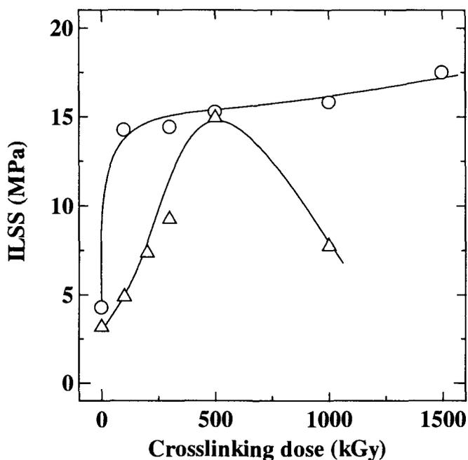
Figure 3 Relationship between the interlaminar shear strength (ILSS) of crosslinked PTFE composite and crosslinking dose. ○:  $V_f$  54.3% and , △:  $V_f$  64.0%.
