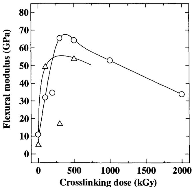
Figure 2 Relationship between flexural modulus of crosslinked PTFE composite and crosslinking dose. ○:  $V_f$  54.3% and , △:  $V_f$  64.0%.
