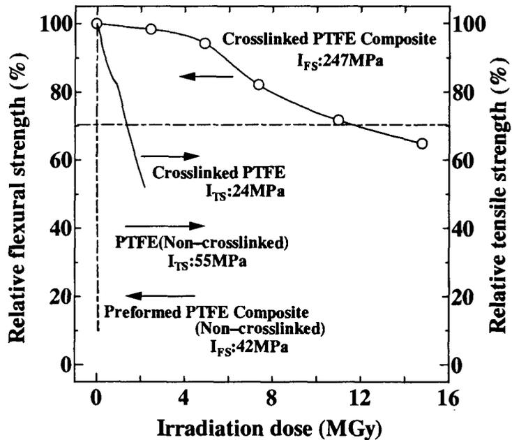
Figure 4 Relative radiation resistance of crosslinked PTFE composite (300kGy for crosslinking) as a function of irradiation dose.
