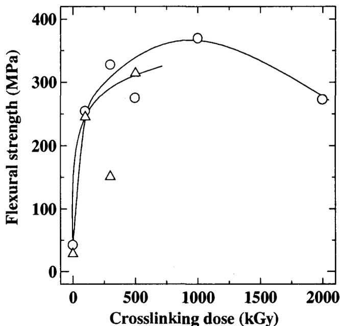
Figure 1 Relationship between flexural strength of crosslinked PTFE composite and crosslinking dose.  $\circ$ :  $V_f$  54.3% and  $\triangle$ :  $V_f$  64.0%.
