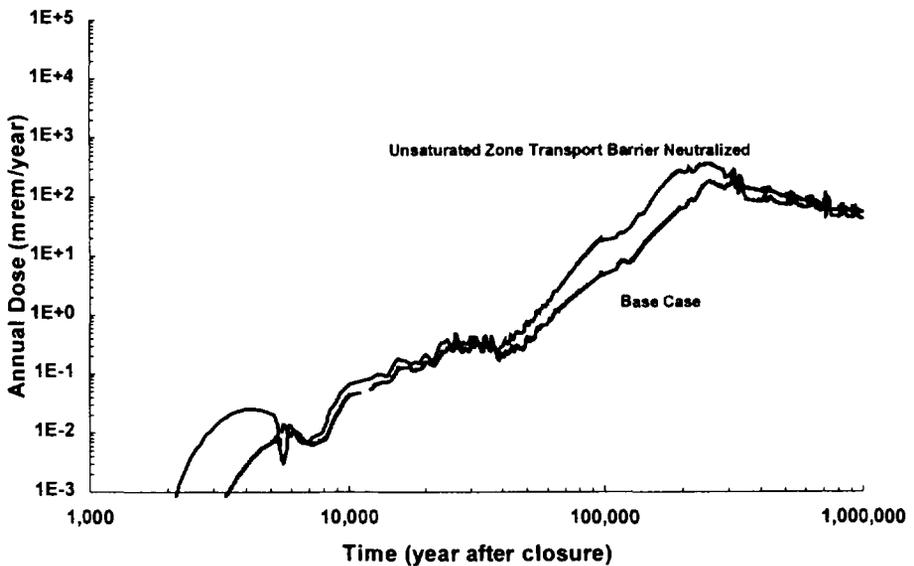
Figure 1. Neutralization of Unsaturated Zone (UZ) of VA Reference System
