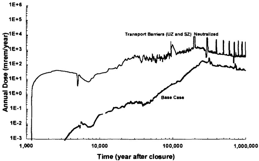
Figure 3. Neutralization of both the Unsaturated Zone (UZ) and the Saturated Zone (SZ) of the VA Reference System
