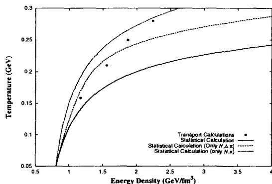
FIG. 6. Caloric curve for nuclear matter. Dotted points are the results of transport calculation, while lines denote the results of statistical calculation for gases with several sets of component. Baryon density is  $\rho_b=0.77/\text{fm}^3$ .
