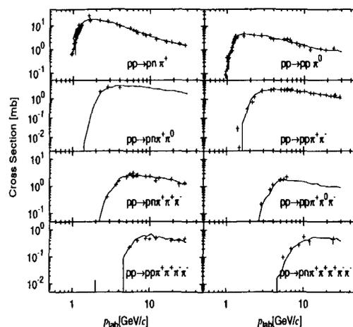
FIG. 2. Inelastic cross sections of  $p-p$  collision. The solid lines denote the results of our calculation, while crosses denote experimental data taken from Ref. [14]
