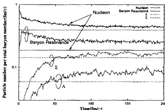
FIG. 7. Time evolution of particle abundance of nucleon(solid line), baryonic resonance(dashed line),  $\Lambda$ (dotted line) and  $\Sigma$ (dashed-dotted line) at  $\rho_b = 0.77 \text{ GeV}/\text{fm}^3$  and  $e=1.87\text{GeV}/\text{fm}^3$ . Straight lines show the results of a statistical model.
