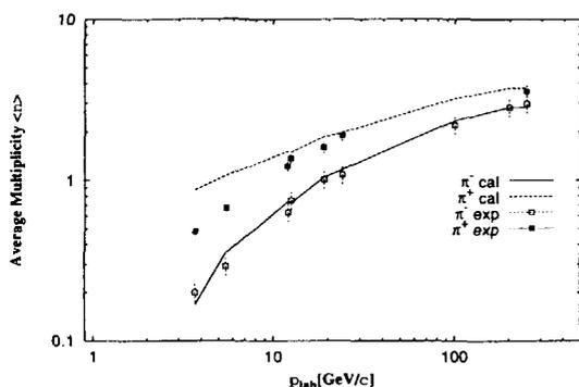
FIG. 1. Average multiplicity of charged pions in  $p-p$  inelastic scattering calculated in our model for  $\pi^-$  (solid) and  $\pi^+$  (dashed). Experimental data for  $\pi^-$  (open squares with dashed error bars) and  $\pi^+$  (solid squares with dotted error bars) are taken from Ref. [13].
