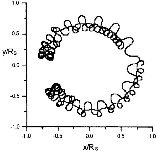
Fig. 3. Fragment of proton trajectory in Hill's vortex FRC ( $B_0=1$  T,  $\varepsilon_{\perp}=10$  keV).
