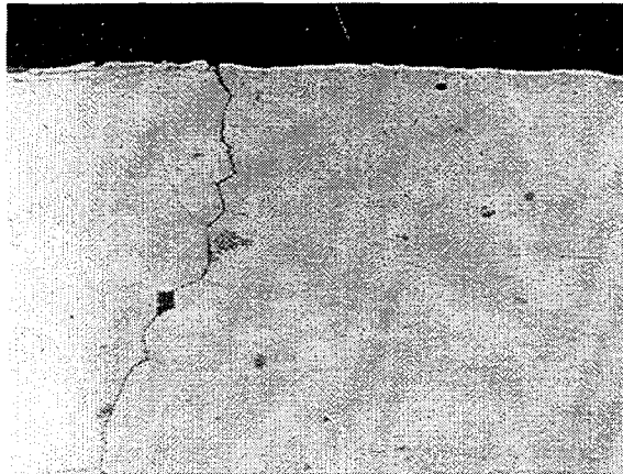
Figure 8: Metallographic Cross Section of Alloy 600 Steam Generator Tubing with an OD Crack and Adjacent Grain Boundary Definition, 500X magnification
