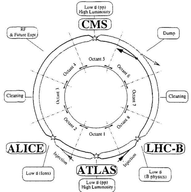
Figure 2: A schematic layout showing the assignment of the eight long straight sections of the LHC to experiments and utilities
