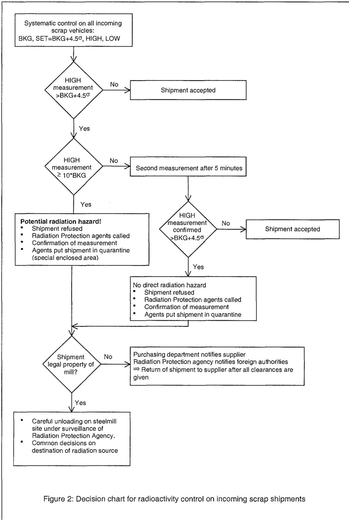
Figure 2: Decision chart for radioactivity control on incoming scrap shipments
