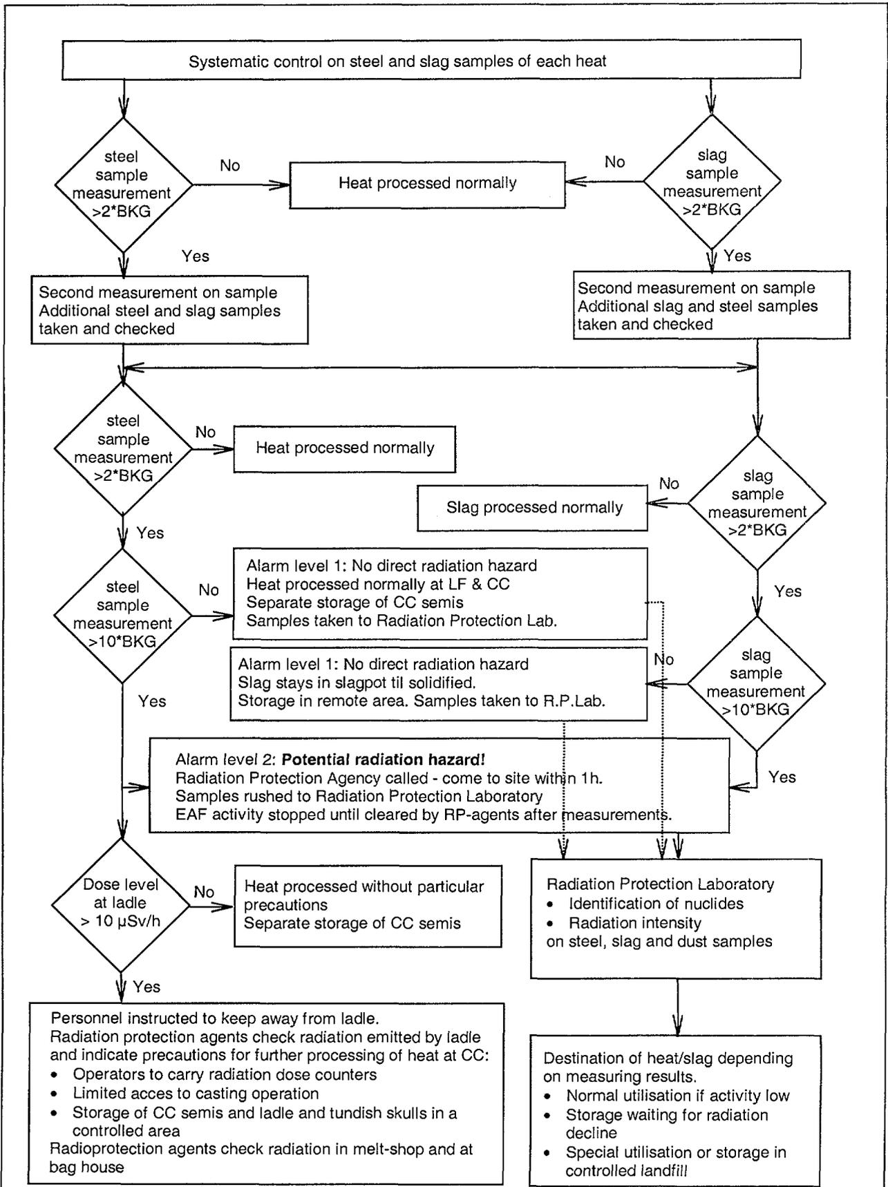
Figure 4: Decision chart for in-plant radioactivity controls
