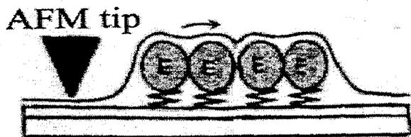
Figure 2 Idealized illustration of contact AFM tip and GOx enzyme covalently attached onto the SAM.
