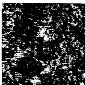
Surfaces of different samples of fabricated enzyme electrode made using different concentrations of GOx were studied by tapping mode AFM in air. A typical image is presented in Figure 3 which shows the presence of array of pentagonal to hexagonal clusters with size of about 50nm in diameter.
