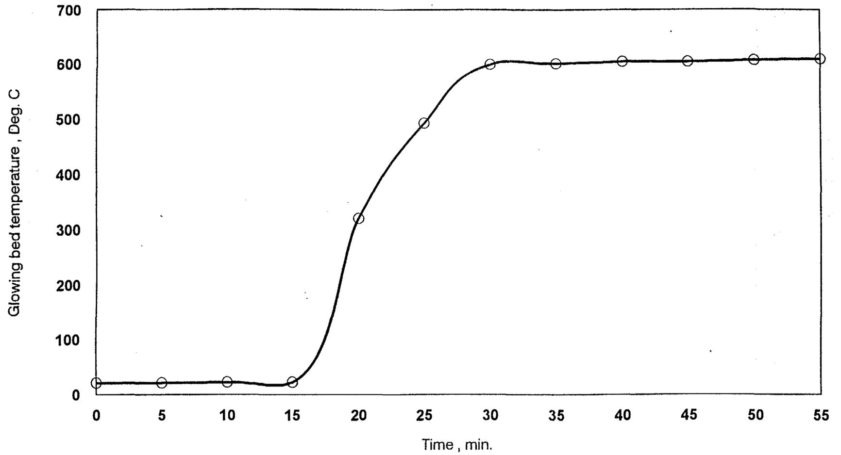
Fig. 3 . Glowing bed temperature versus time at start-up
