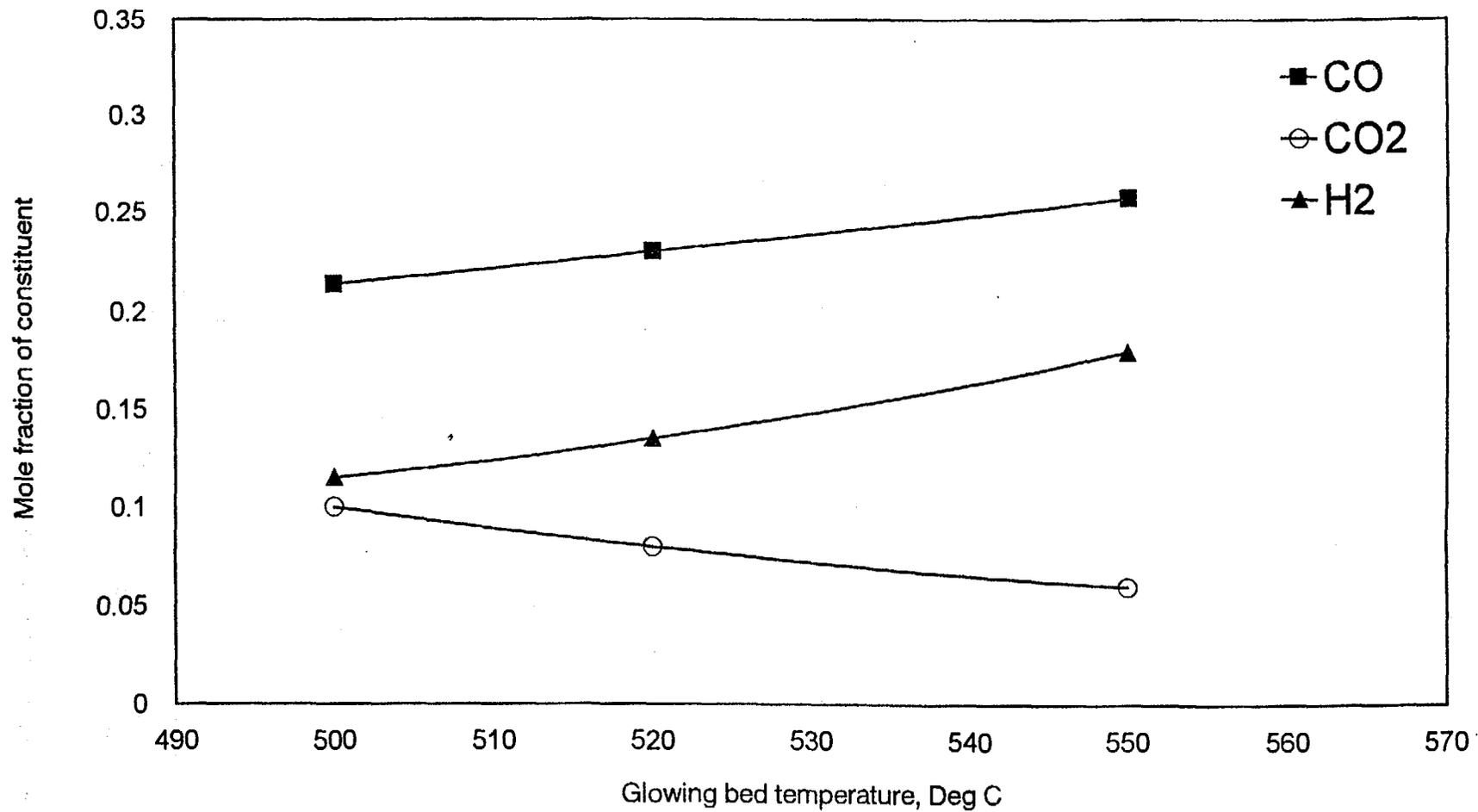
Fig. 5 Influence of glowing bed temp. on CO, H2 and CO2 in gas reactor effluent
