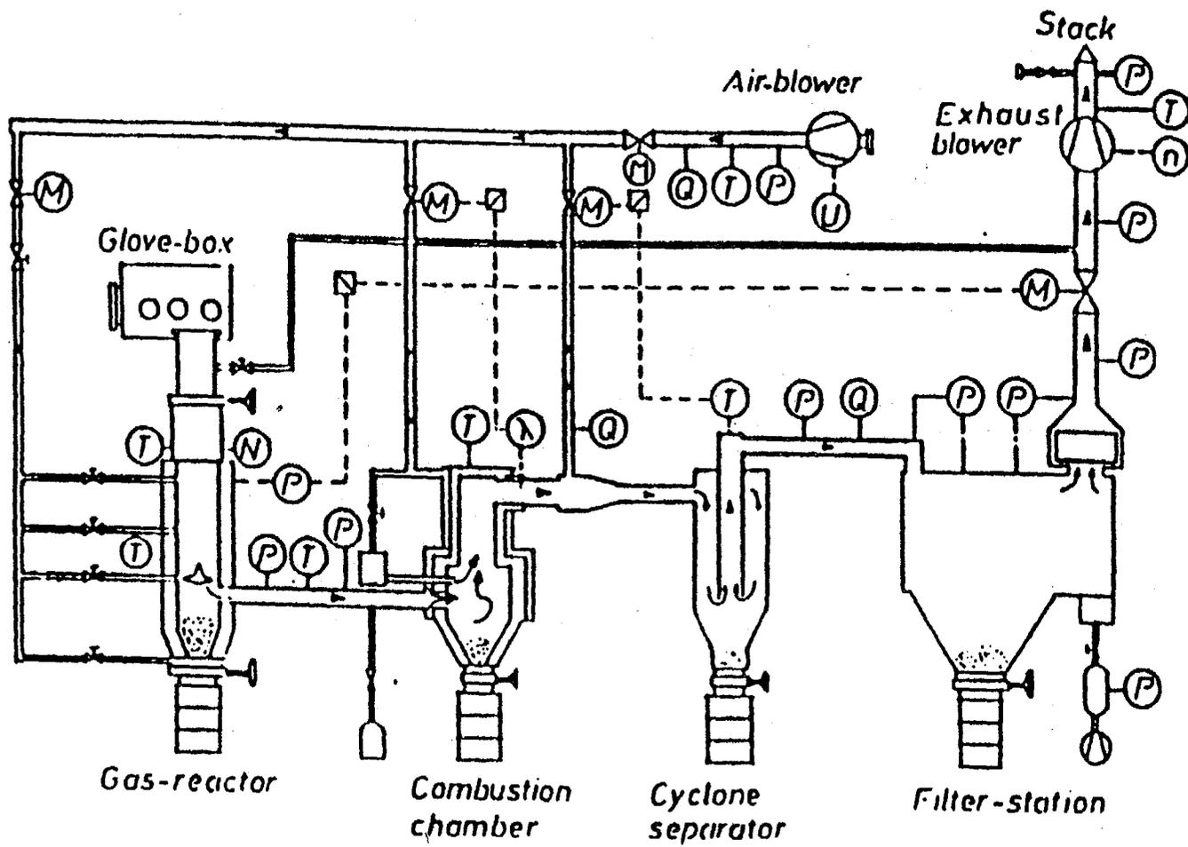
Figure(1). Schematic LAWI flow sheet.
