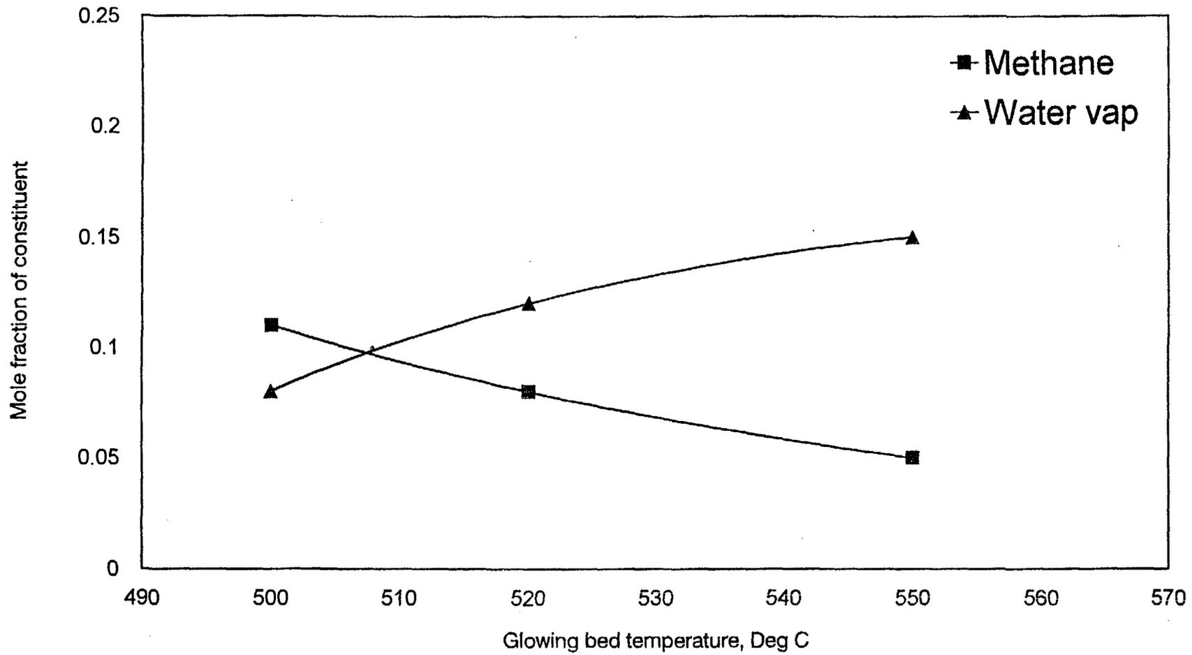
Fig. 6 Influence of glowing bed temp. on methane and water vap. and methane in gas reactor effluent .
