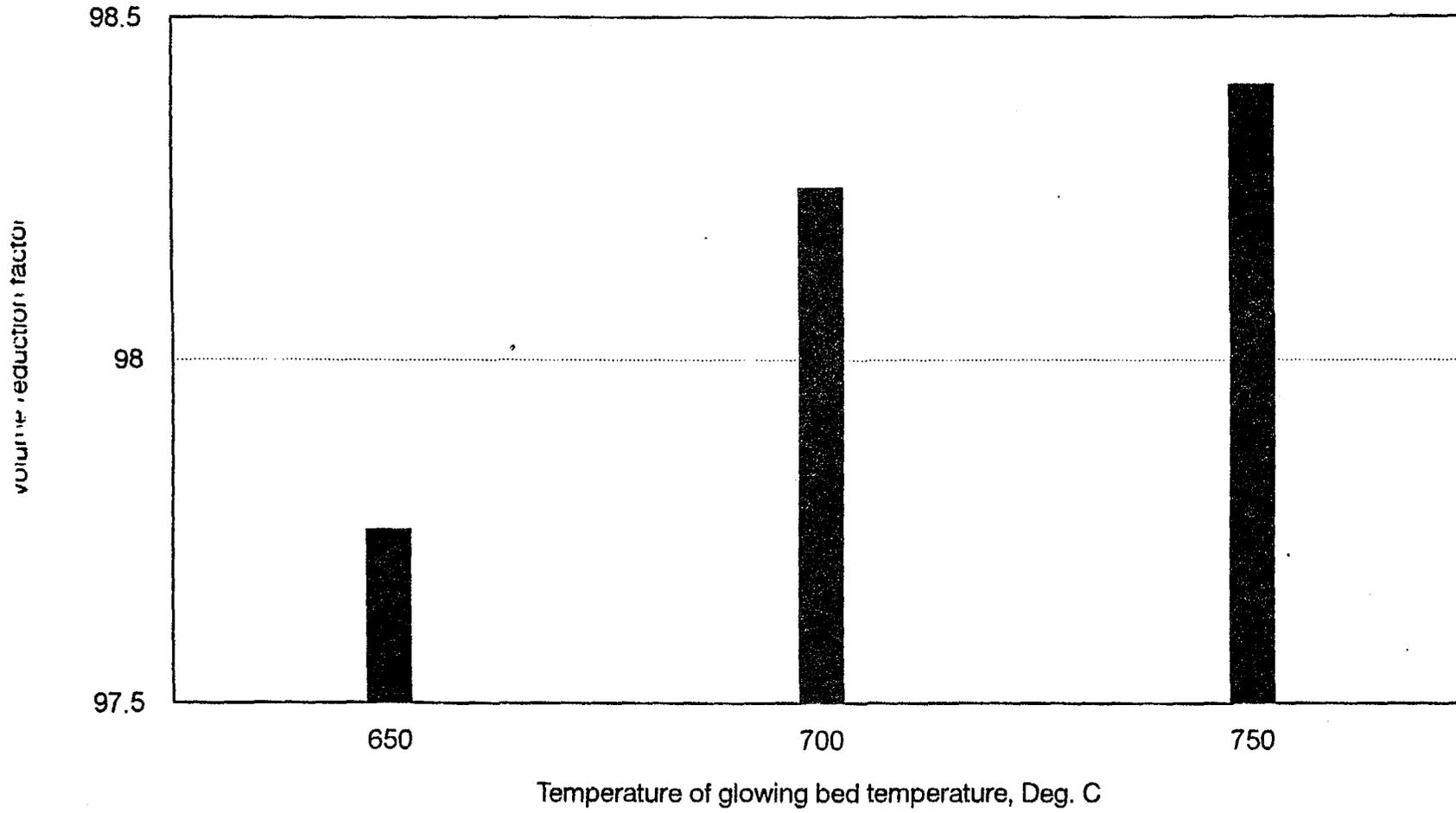
Fig. 7 Volume reduction by incineration
