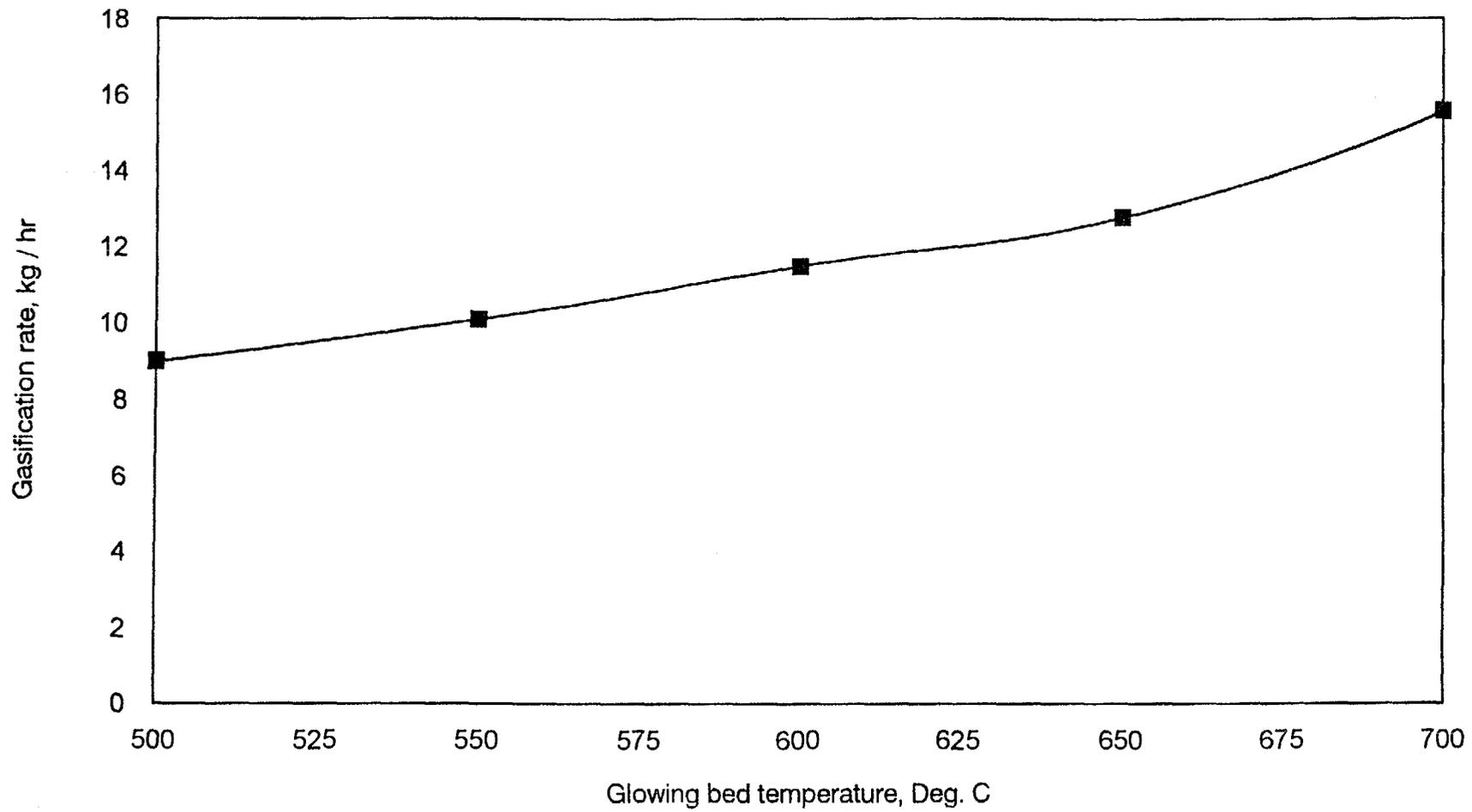
Fig. 4. Influence of glowing bed temperature on gasification rate
