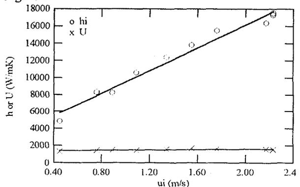
Figure 3. The effect of hot water velocity on heat transfer coefficients.
