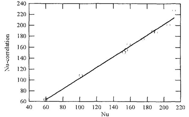
Figure 7. Comparison of Nu numbers obtained from the measurements and calculated from equation (11).
