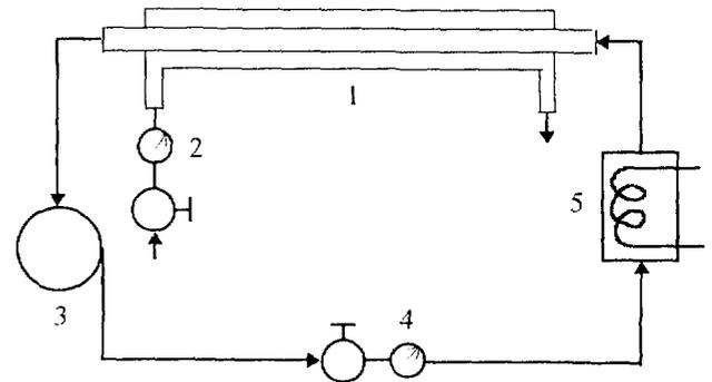
Figure 1. Schematic diagram of experimental apparatus. 1-Heat exchanger, 2-Cold water flow meter 3-Pump, 4-Hot water flow meter, 5-Heater.
