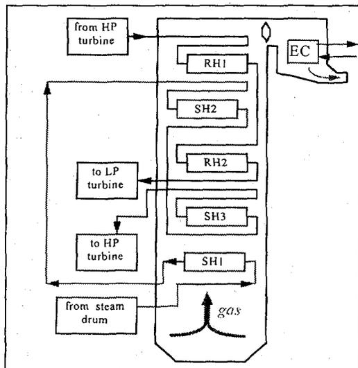
Fig. 1: Scheme of the boiler
