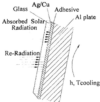
Fig 4 – Thermo-Mechanical model of a panel.
