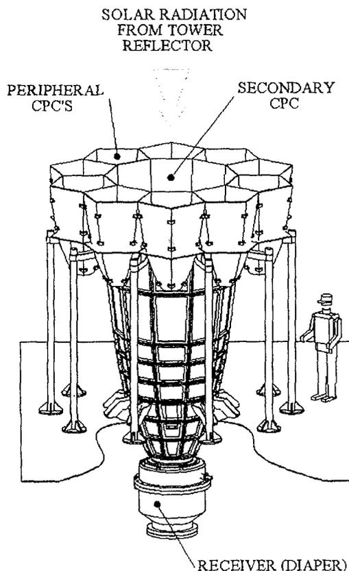
Fig.1 - CPC's/Receiver arrangement (Heliostats, Tower Reflector and Turbine are not shown).
