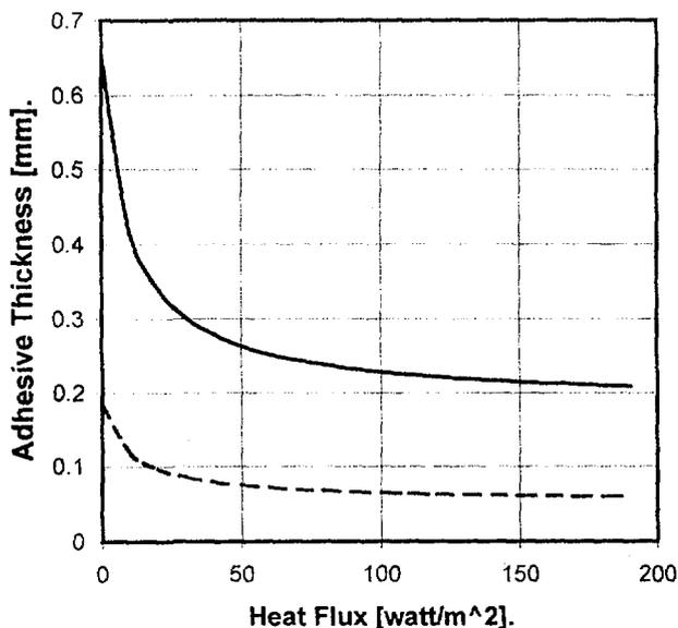
Fig. 5 – Adhesive thickness for the VERTEC glass -----, and for the BOROFLOAT glass —, at zero stress conditions.
