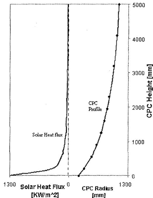
Fig 3 - CPC profile and the solar heat flux distribution
