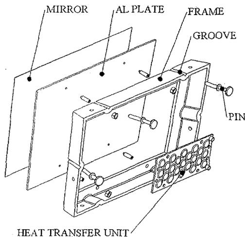
Fig. 2 - CPC's Module – Exploded Rear View.
