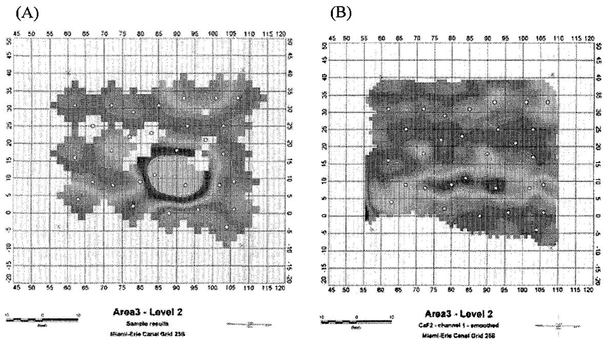
FIG. 9. Contoured  $^{238}\text{Pu}$  data from A) 30 hand collected samples and B) 21,916 in situ measurements.
