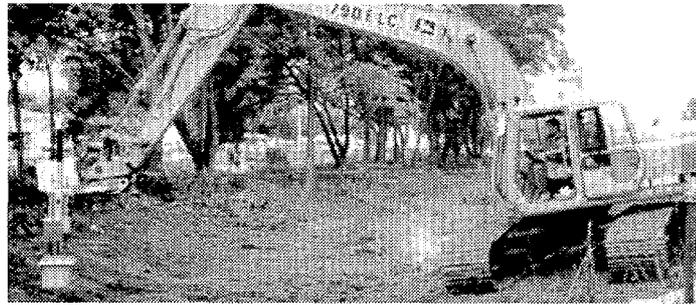
*FIG. 4. INEEL excavator mounted system (EMS) in situ characterization at DOE Mound.*
