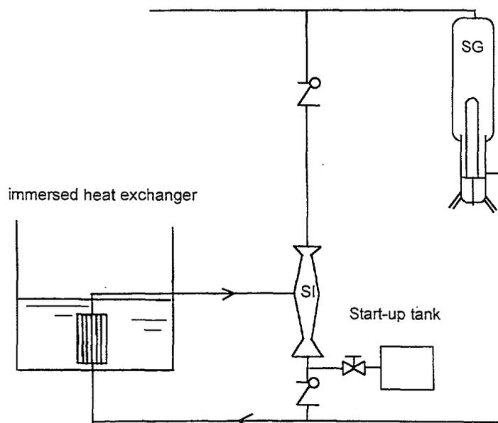
FIG. 1. Recirculation configuration [7].
