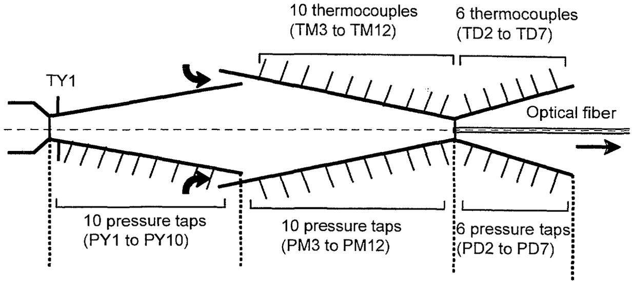
FIG. 5. Instrumentation.
