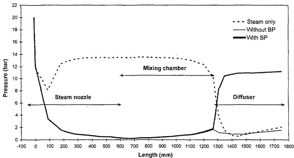
FIG. 6. Pressure profiles for a 2 MPa test.
