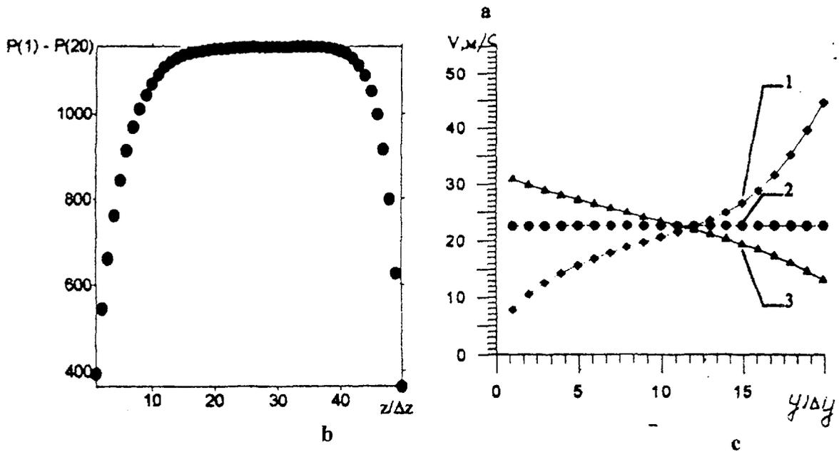
Fig. 2. The flow through the porous structure ( $\alpha=10^\circ$ ,  $h=3$  m,  $k_{\eta\eta}=3.8$ ,  $k_{\xi\xi}=62$ ,  $u_0=22.6$  m/c/c): a) longitudinal velocity component distribution in the channel; b) transversal pressure drop distribution along the channel; c) longitudinal velocity distribution through the height of the channel in the entrance (1), the exit (3) and in the centre (2) of the porous insert.
