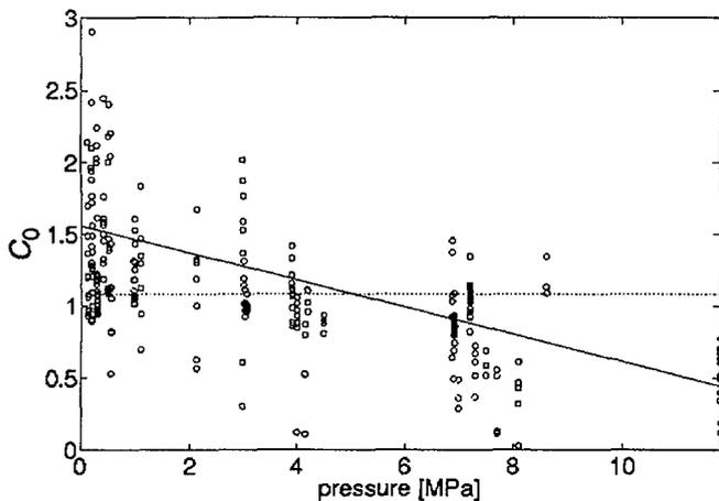
Fig. 2: Effect of system pressure on  $C_0$  with  $v_{gj}$  as parameter.
