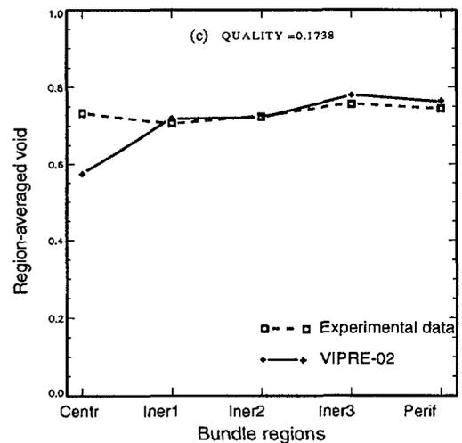
Fig. 15: Region-averaged void for the standard 8x8 assembly: BWR nominal conditions.
