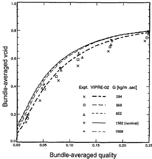
Fig. 16: Bundle-averaged void versus quality: mass flux parameter.
