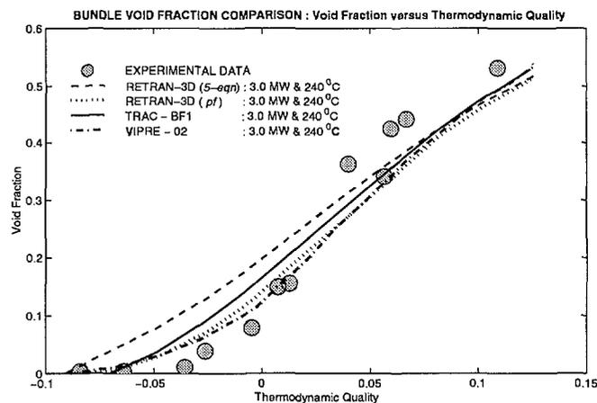
Fig. 10: Rod Bundle A comparison, pressure 12.3 Mpa.
