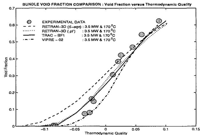
Fig. 9: Rod Bundle B comparison, pressure 7.4Mpa.
