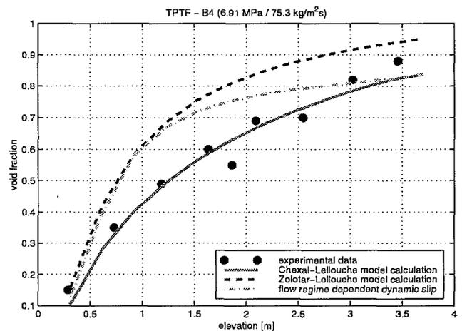
Fig. 5: Prediction of a TPTF experiment using the 4-equation model option.
