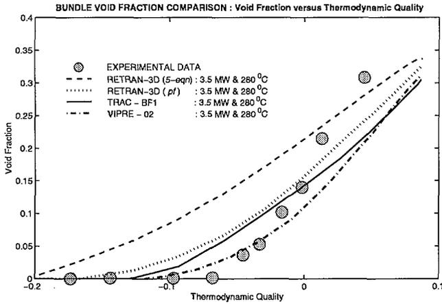
Fig. 11: Rod Bundle B comparison, pressure 166 bar.
