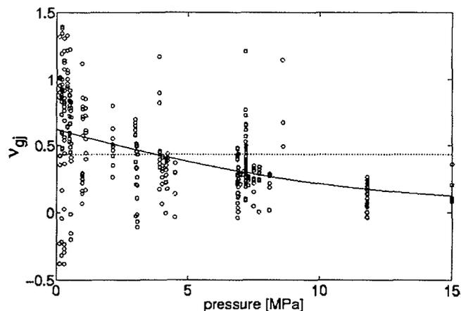
Fig. 3: Effect of system pressure on  $v_{gj}$  with  $C_0$  as parameter.
