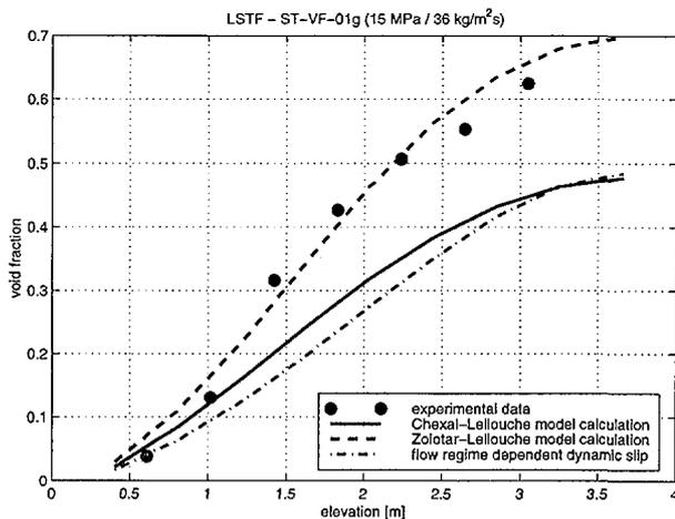
Fig. 7: Prediction of an LSTF experiment using the 4-eq. model option.
