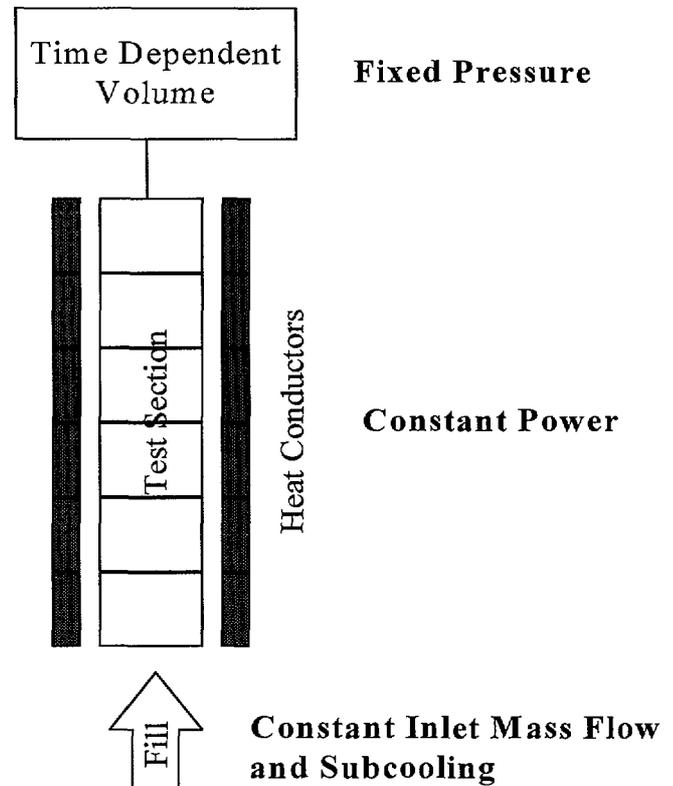
Fig. 4: RETRAN nodalization diagram.
