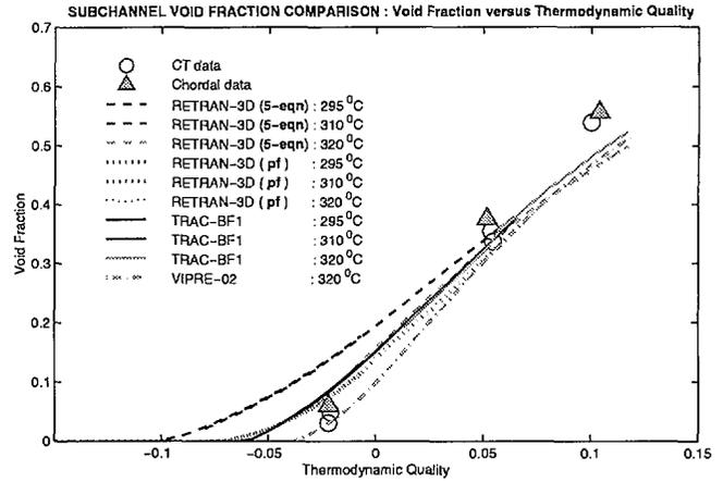
Fig. 12: Subchannel comparison, pressure 123 bar.
