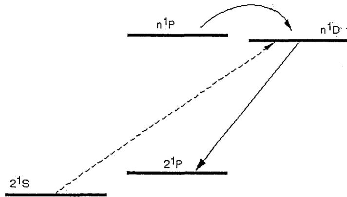
Figure 1 Energy levels and transitions of the helium atom used for the measurement of electric fields by LIF
