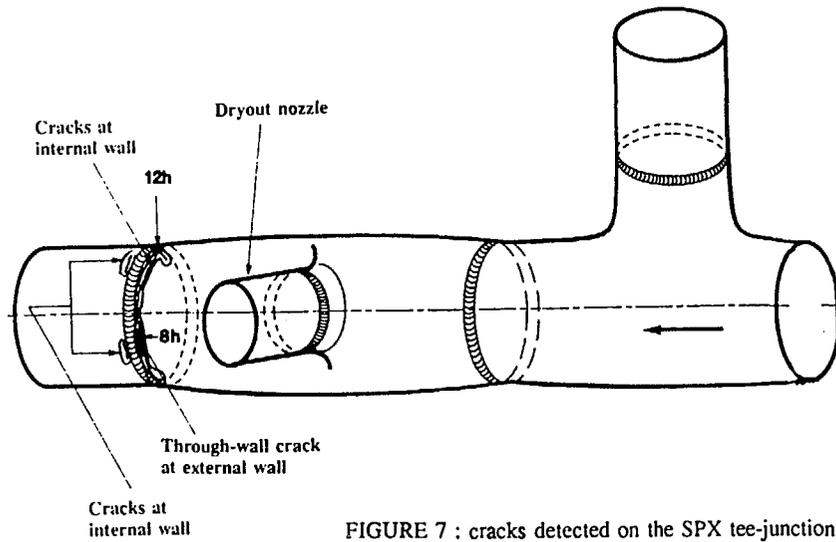
FIGURE 7 : cracks detected on the SPX tee-junction
