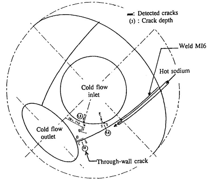
**FIGURE 2 : detected cracks on the PHENIX expansion tank**
