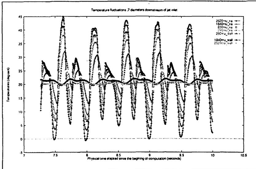
Figure 2 : Temperature fluctuations .07 meters downstream of hot jet
