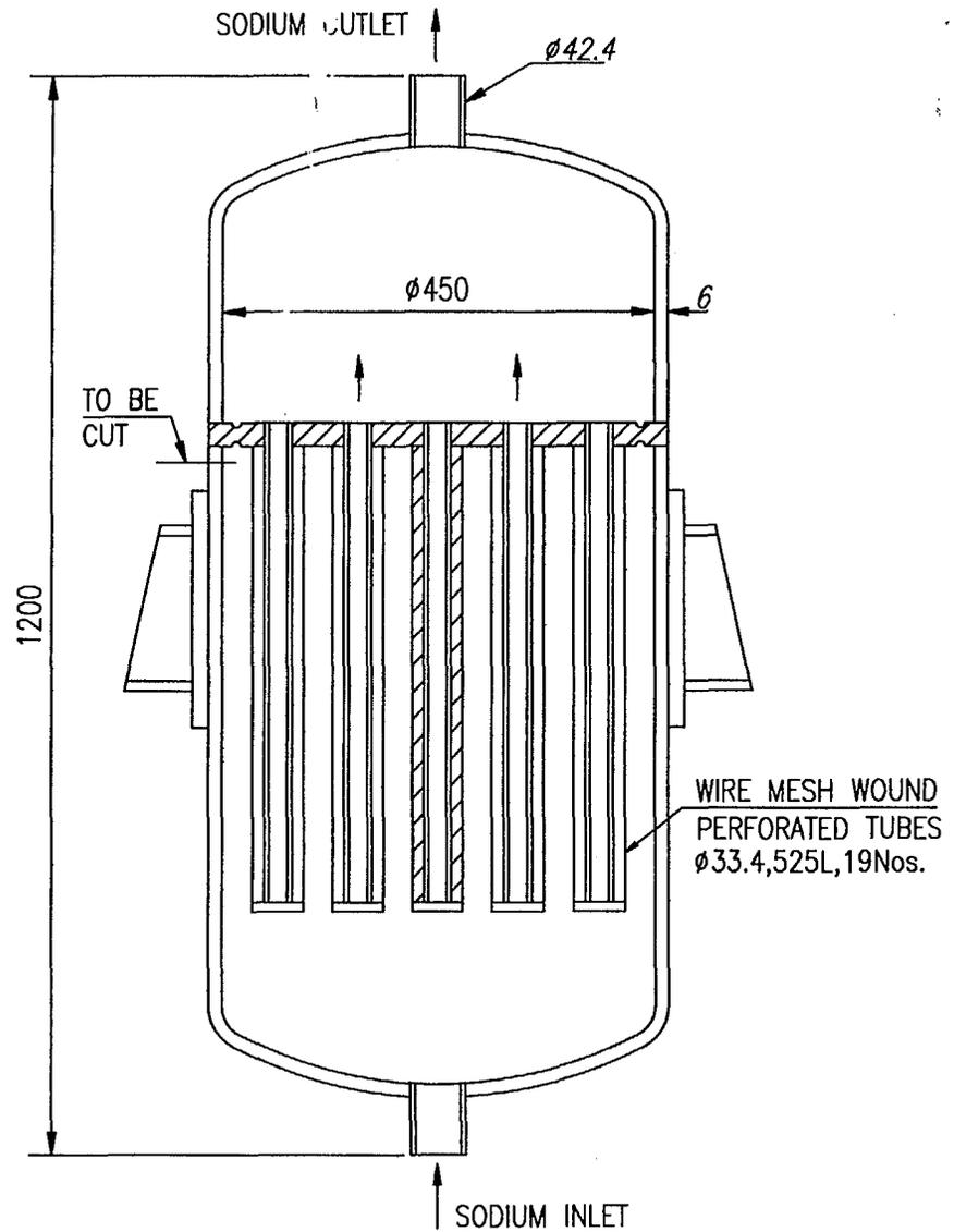
Fig. 2 COARSE FILTER
