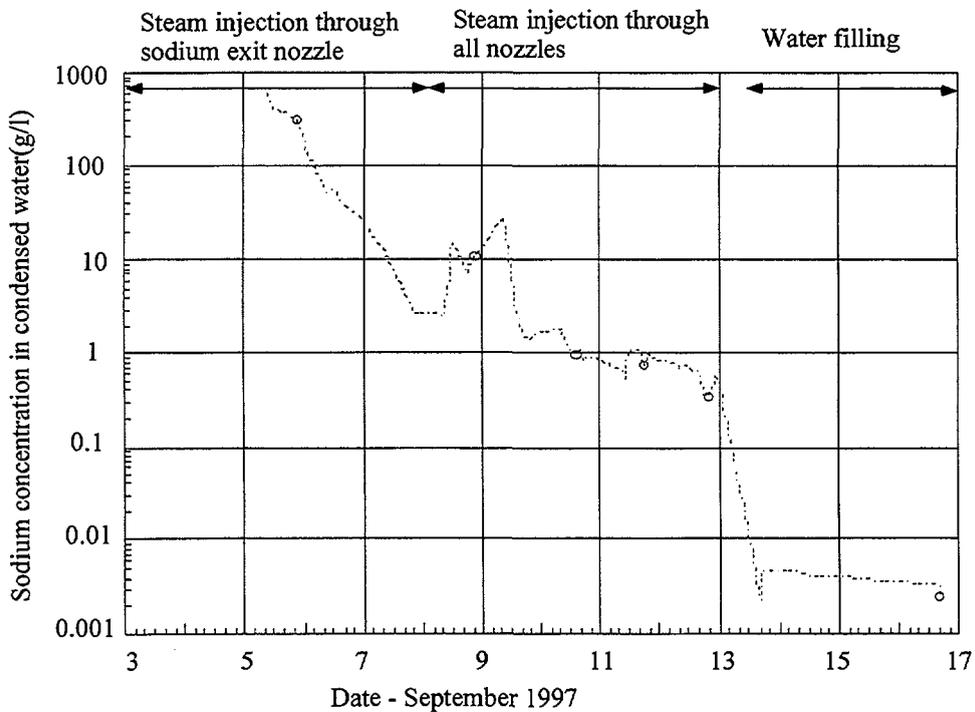
Figure 9 Sodium concentration in condensed water
