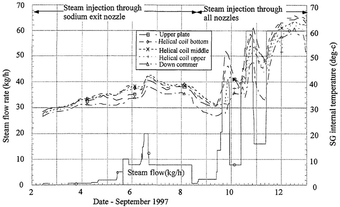
Figure 8 SG temperature during steam injection
