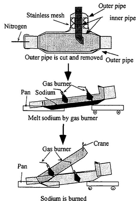
Figure 5 Shape and dismantling process of mixing tee
