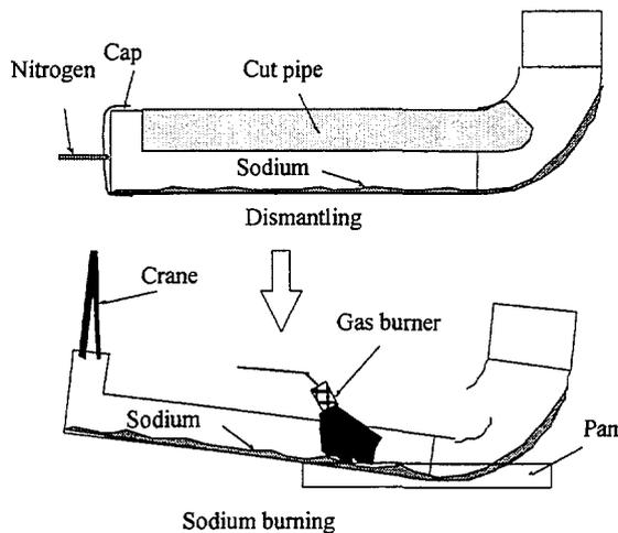
Figure 4 Sodium removal process of piping
