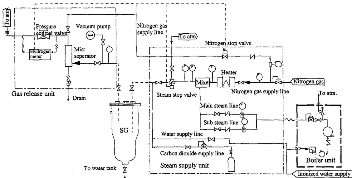
Figure 6 P & I drawing of the SG cleaning system
