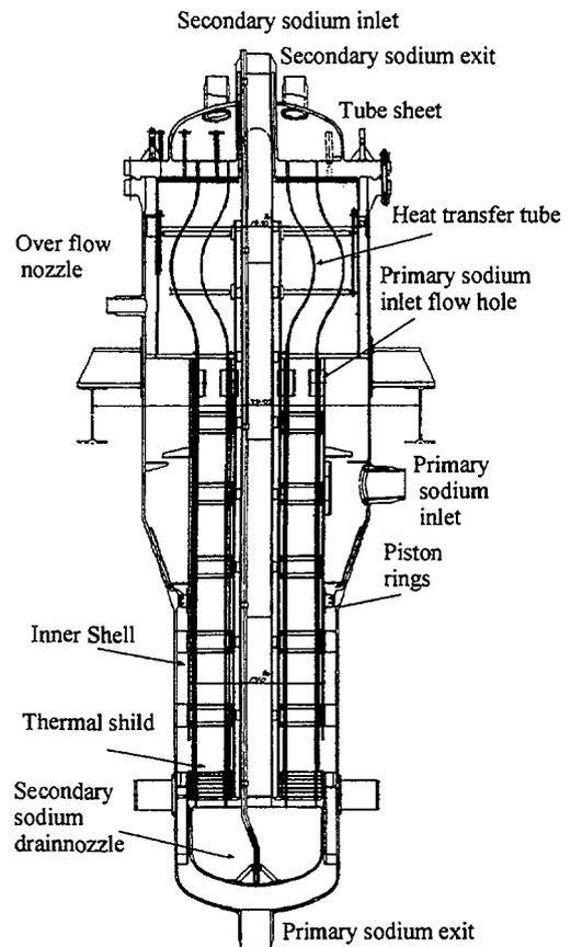
Figure 3 50MW IHX Structure
