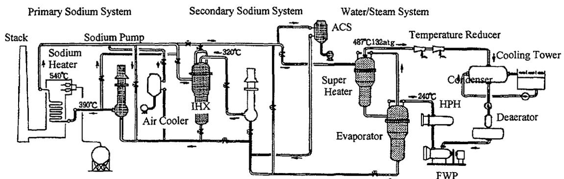
Figure 1 Schematic Diagram of 50MWSGTF
