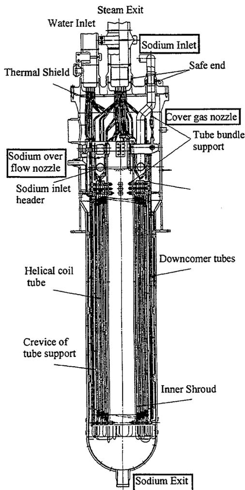
Figure 2 Structure of #2 50MW Steam Generator
