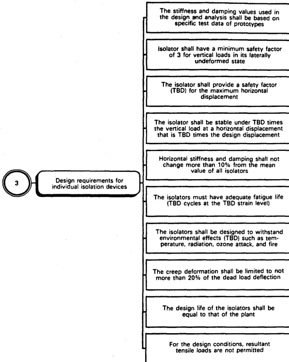
Fig. 4. Design guidelines for nuclear reactors isolated by HDLRBs: qualification of seismic isolation bearings; acceptance testing of isolation devices; seismic isolation reliability; seismic safety margin assessment; seismic monitoring.
