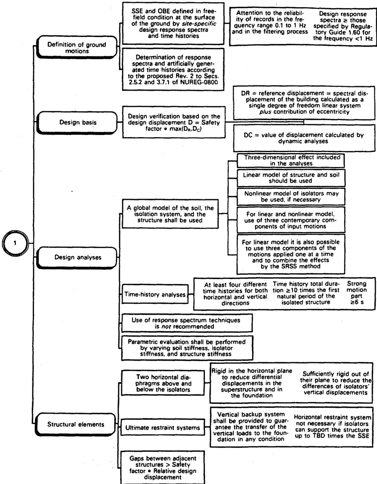
Fig. 2. Design guidelines for nuclear reactors isolated by HDLRBs: design and performance requirements for overall seismic isolation systems; design requirements and analysis methods for isolated structures, systems and components; design requirements and analysis methods for interface components.
