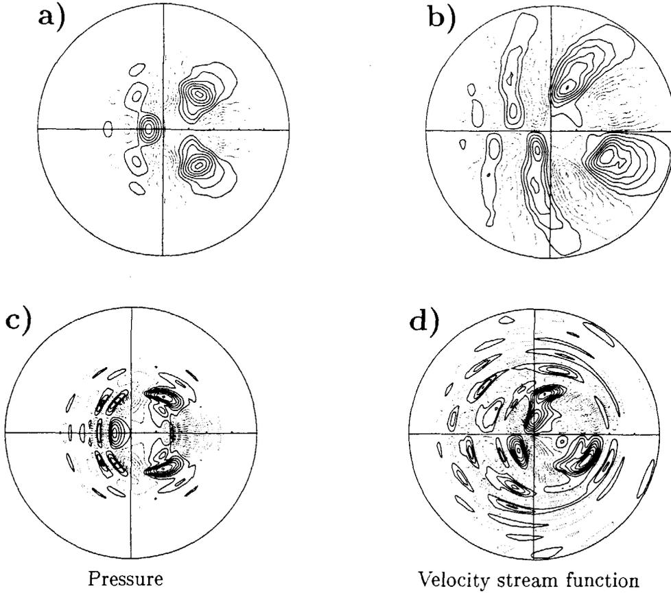
Figure 1. a) and b) Contours for resistive MHD 3/2 mode in a torus with strong  $\kappa_{\parallel}$  and density evolution,  $\gamma = 0.01$ . The case with  $\kappa_{\parallel} \simeq 0$  and  $\partial n/\partial t = 0$  has similar contours, but larger  $\gamma = 0.029$ . c) and d) Case with large  $\kappa_{\parallel}$  and  $\partial n/\partial t = 0$  is stable,  $\gamma < 0$ .
