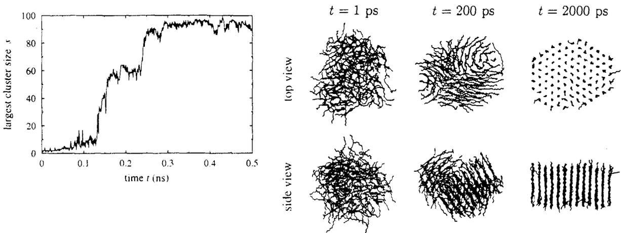
Fig. 1 Stepwise formation of orientational structure in short polymer chains.
