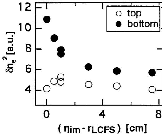
Figure 1. Top and bottom squared density fluctuation level  $\delta n_e^2$  versus the lower modular limiter distance to the LCFS.
