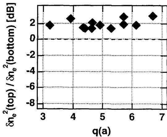
Figure 4. Up-down asymmetry for reversed plasma current versus the edge safety factor  $q(a)$ , with plasmas leaning on the lower limiter located close to the measurement chord.
