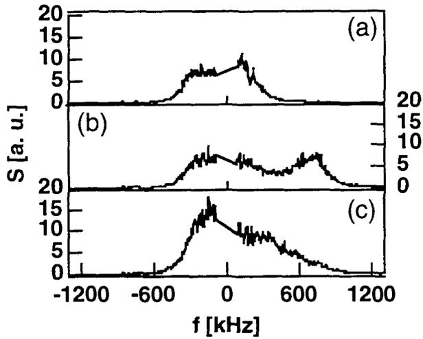
Figure 2. Frequency spectra measured at the bottom of the plasma, for distinct lower limiter positions: (a)  $r_{lim} - r_{LCFS} = 7$  cm, (b)  $r_{lim} - r_{LCFS} = 1$  cm, and (c)  $r_{lim} = r_{LCFS}$ .
