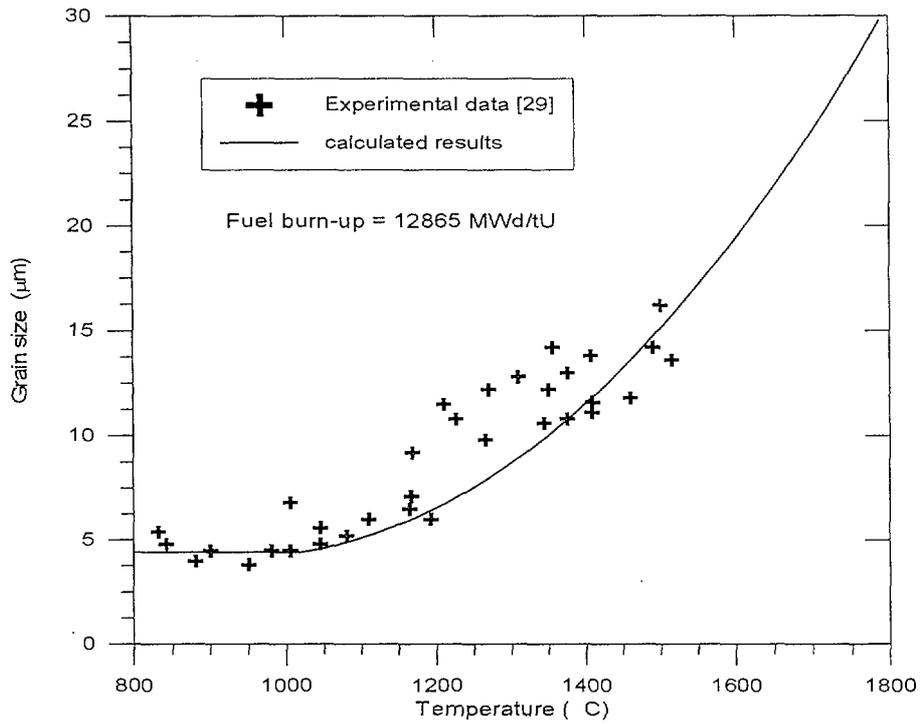
Fig. 2. Comparison of measured and calculated fuel grain growth results
