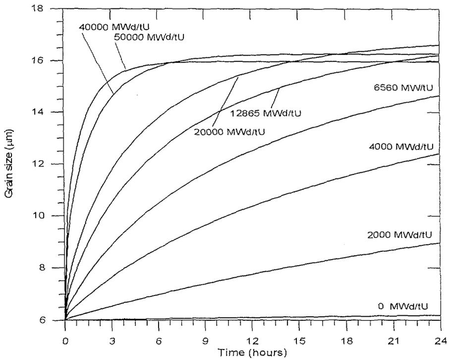
Fig. 5. Grain growth as a function of time for several values of fuel burnups and at the constant temperature of 1300 C.
