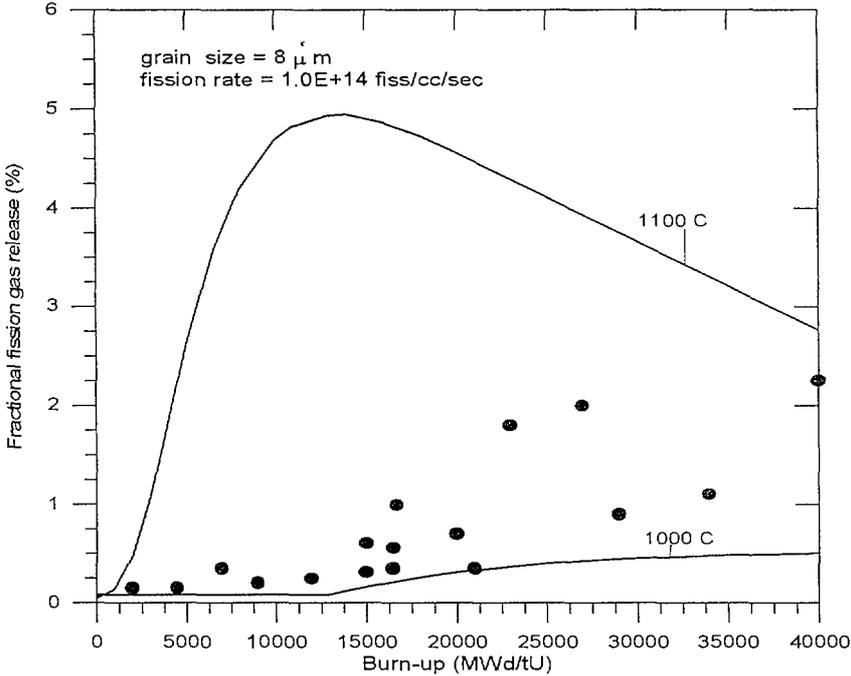
Fig. 7. Comparison of the fractional fission gas release as a function of burn-up with the experimental data copied from Fig. 2. of Ref. [44].
