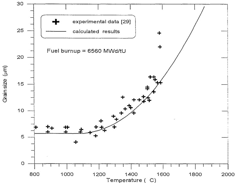
Fig. 1. Comparison of measured and calculated fuel grain growth results.
