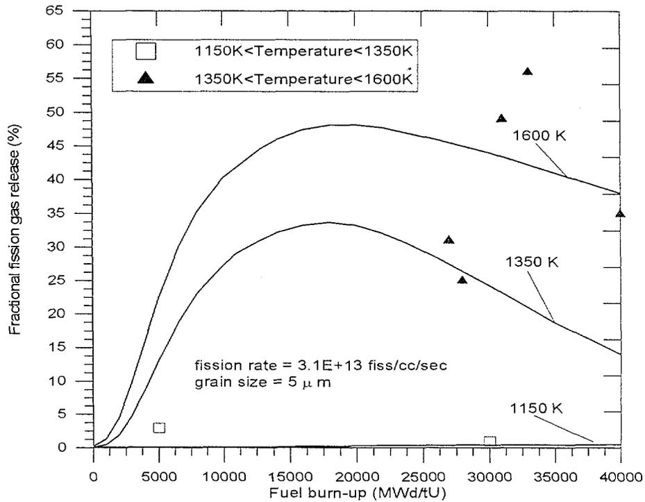
Fig. 9. Comparison of calculated fractional fission gas release as a function of burn-up with the experimental data copied from Fig. 3. of Ref. [37].
