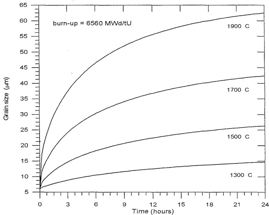
Fig. 6. Grain growth as a function of time for different values of fuel temperature
