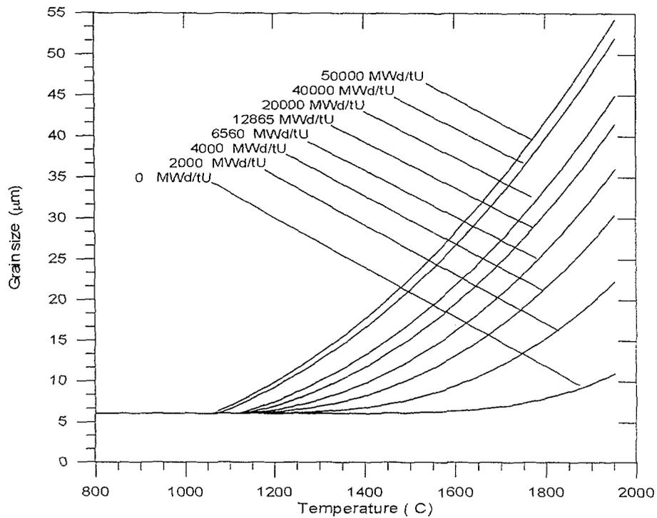
Fig. 4. Fuel grain growth as of fuel temperature for various values of fuel burn-up
