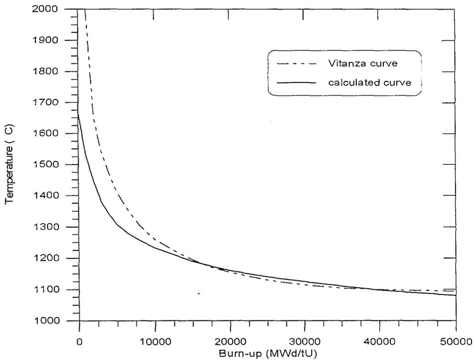
Fig. 3. Comparison between the calculated recrystallization temperature and Vitanza curve [19].
