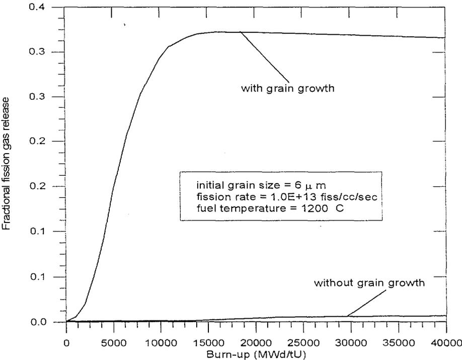
Fig. 8. Comparison between fractional fission gas release with and without grain growth.
