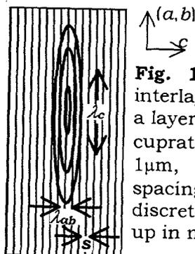
**Fig. 1.** Cross-section of an interlayer Josephson vortex in a layered superconductor. For cuprates,  $\lambda_{ab} \approx 0.1-0.2\mu\text{m}$ ,  $\lambda_c > 1\mu\text{m}$ , and the interlayer spacing  $s \approx 10\text{\AA}$ , so the discrete layers do not show up in magnetic images.
