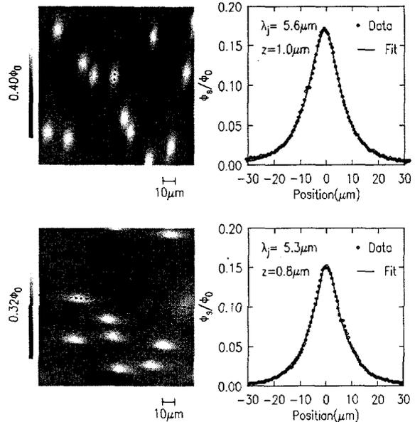
**Fig. 4.** Images of interlayer Josephson vortices in La<sub>1.83</sub>Sr<sub>0.17</sub>CuO<sub>4</sub> taken with two different orientations of the sample and pickup loop, to check for systematic errors induced by the pickup loop shape, and fits to one vortex from each image.
