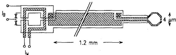
**Fig. 2.** Sketch of a SQUID designed for scanning SQUID microscopy. The  $4 \mu\text{m}$  octagonal pickup loop is separated from the junctions and mod coil ( $l_M$ ).
