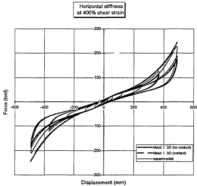
Figure 13. Experimental & numerical horizontal stiffness: results obtained considering the effect of sliding at the rubber-lead interface
