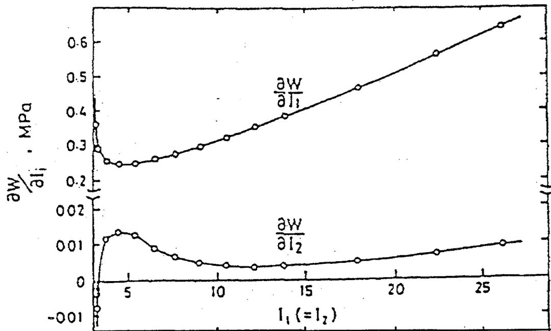
Figure 2. Strain energy density function
