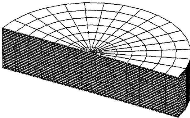
Figure 6. 3D mesh of CRIEPI LRB
