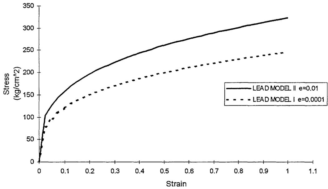
Figure 5. Stress-strain curves of lead plug
