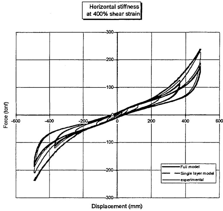
Figure 12. Experimental & numerical horizontal stiffness: results obtained using the single rubber layer model and 3D FEM
