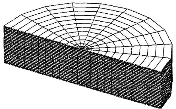
Figure 7. Asisymmetric mesh of CRIEPI LRB
