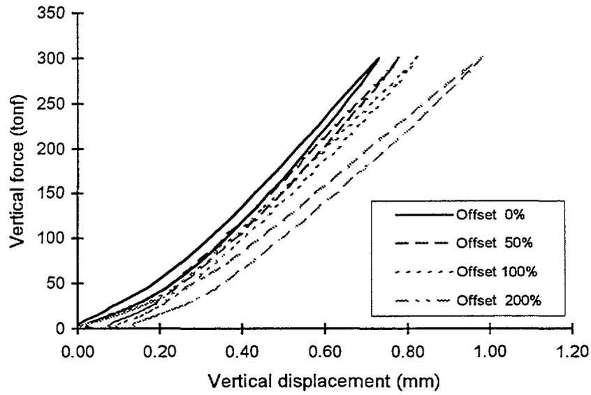
Figure 3. Compression test with different offsets shear strain on CRIEPI LRB
