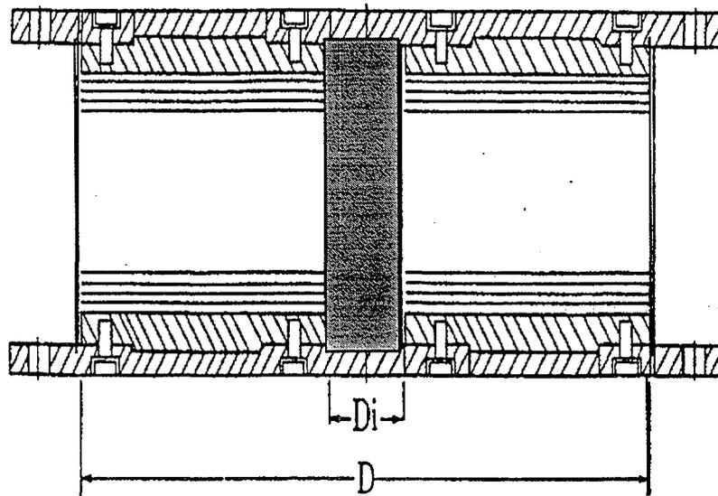
Figure 1. Sketch of the 1:1.83 scale prototype of the CRIEPI LRB
