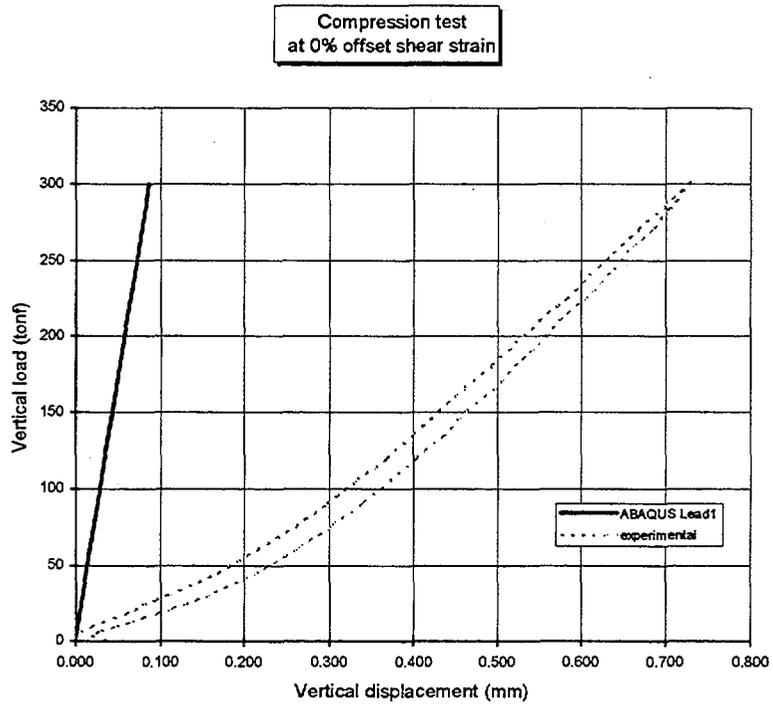
Figure 8. Comparison between experimental and numerical vertical stiffness at 0% offset shear strain
