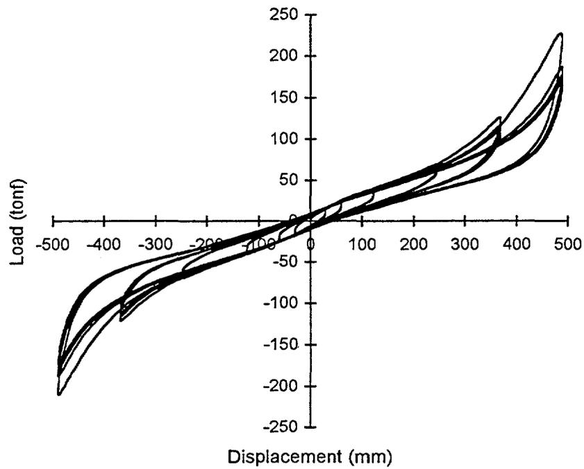
Figure 4. Combined compression & shear strain tests on CRIEPI LRB
