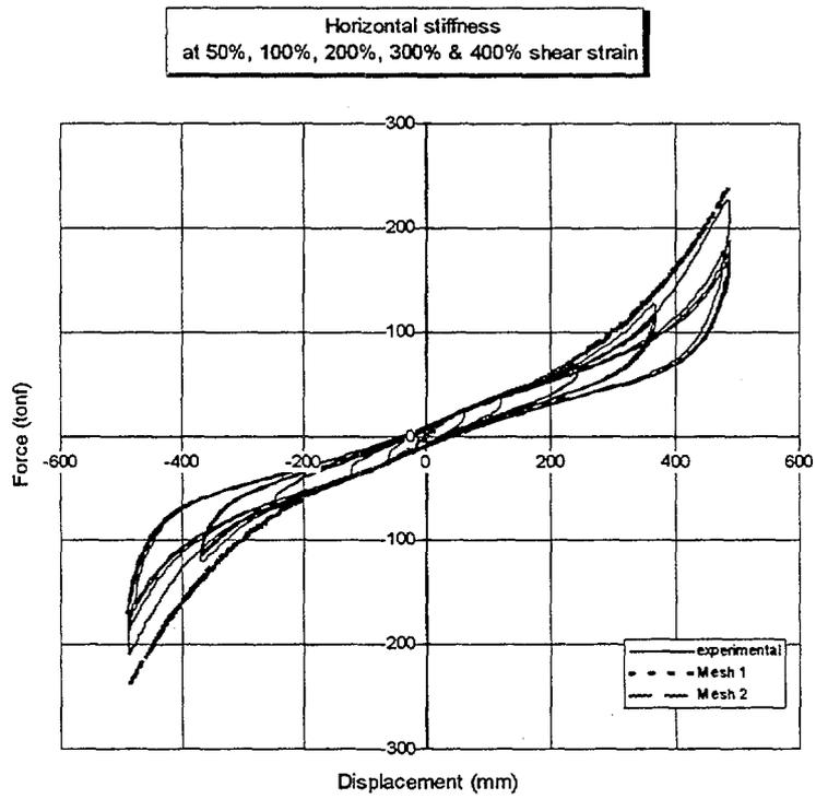
Figure 10. Comparison between experimental & numerical horizontal stiffness: results obtained using two different meshes
