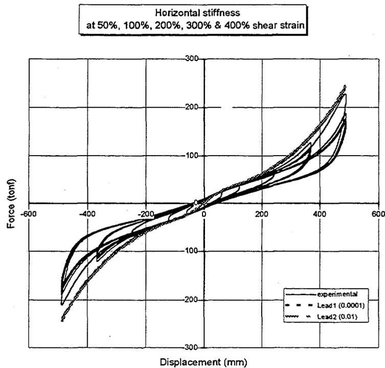
Figure 9. Comparison between experimental & numerical horizontal stiffness: results obtained using the same mesh and two different lead characterisations
