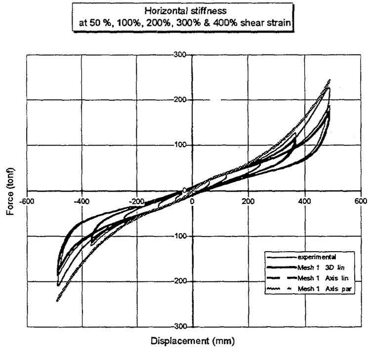
Figure 11. Experimental & numerical horizontal stiffness: results obtained using 3D and axisymmetric elements
