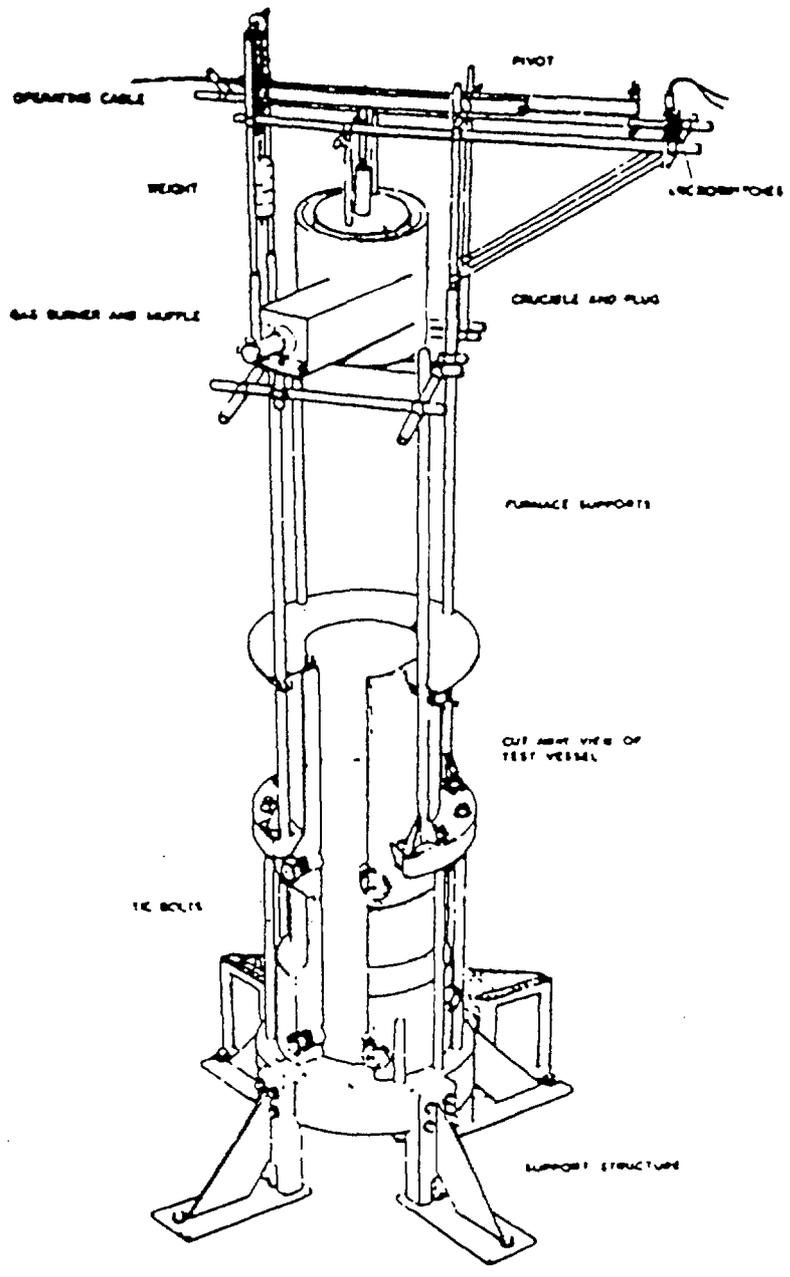
Fig 1. Fig 1. Test Vessel, Furnace, and Release Mechanism. Briggs (1976)
