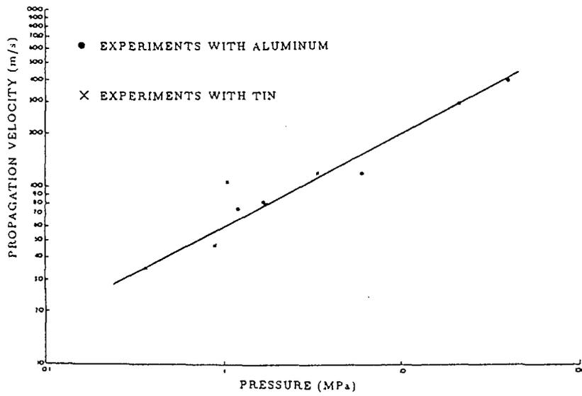
Fig 2. Variation of Propagation Velocity with Peak Pressure, Fry and Robinson
