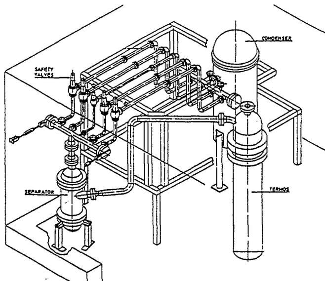
Fig 4. Faro Test Facilities (Test arrangement and venting system)
