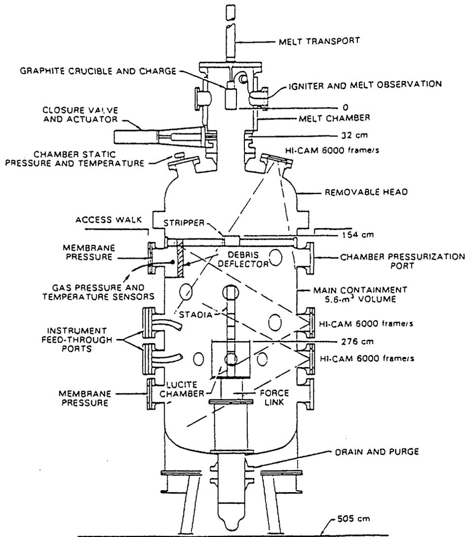
Fig 3. Containment Chamber (Mitchell et al. [29]).
