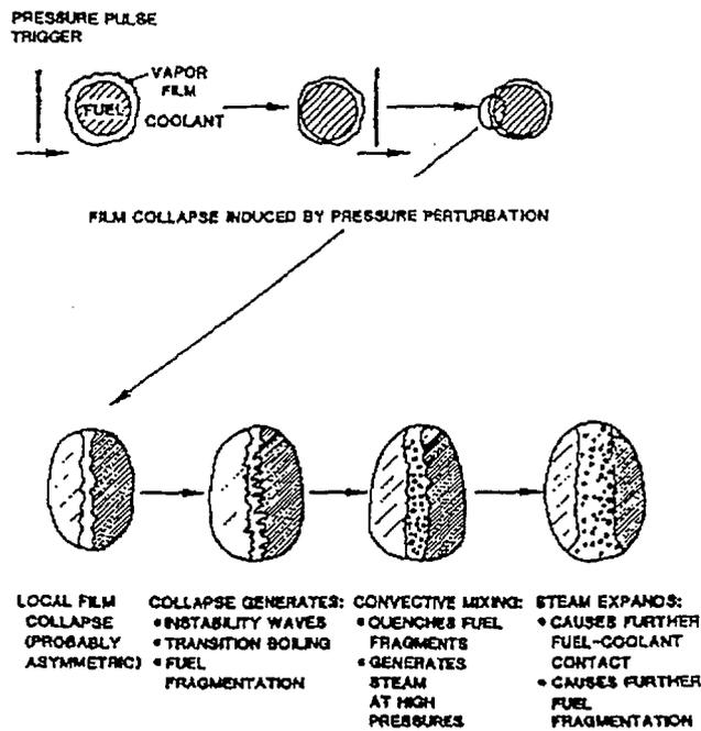
Fig 12. Physical Picture of Thermally Induced Fuel Fragmentation by Taylor Instability
