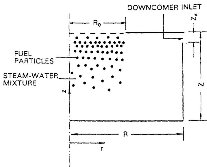
Fig 9. Geometry of Premixing Model, Abolfadl and Theofanous
