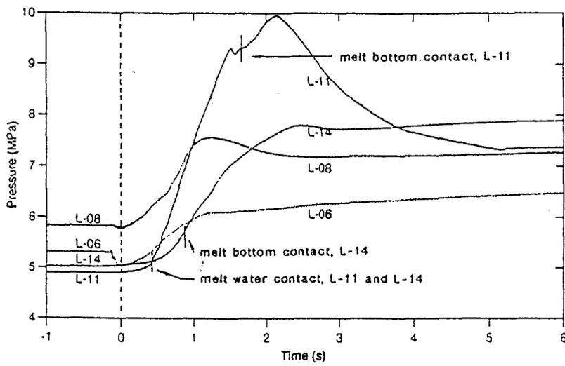
Fig 5. Vessel Pressure History in Test L-06, L-08, L-11, and L-14
