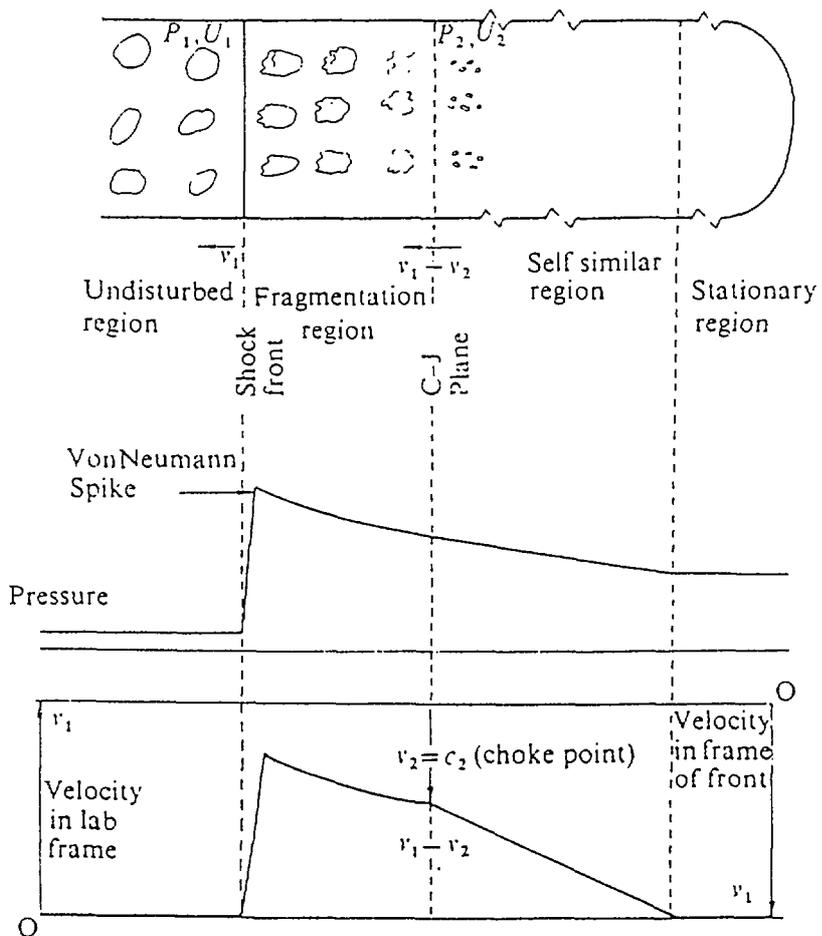
Fig 16. Geometry and Schematic Pressure and Velocity Profiles of a One Dimensional Explosion, Board et al.
