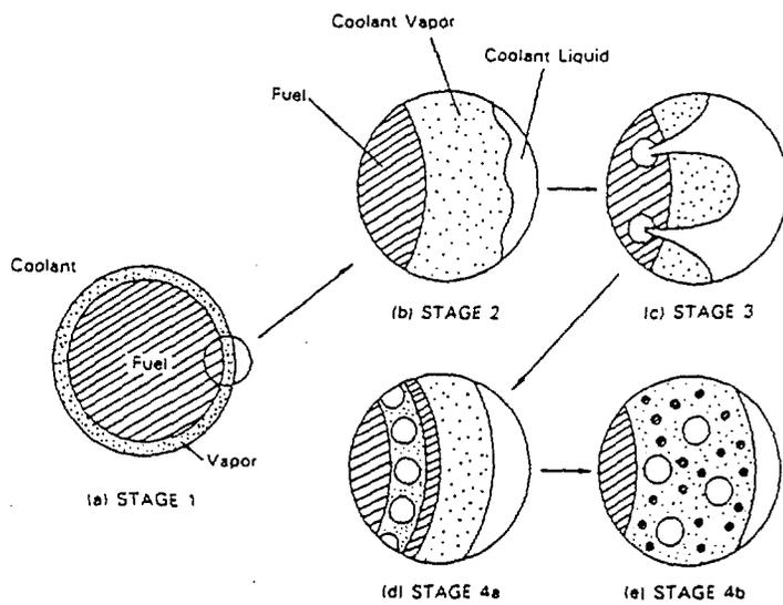
Fig 13. Illustration of Fragmentation by Coolant Entrapment due to Film Collapse and Inward Jet Penetration
