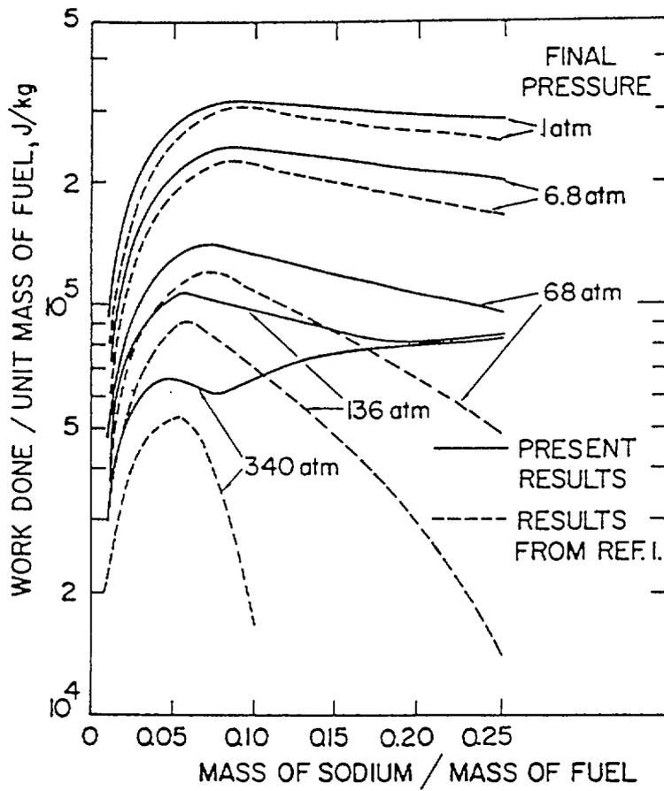
Fig 17. Thermodynamic Work Calculated for  $UO_2$  Fuel and Sodium Coolant Compared to Results of Hicks and Menzies
