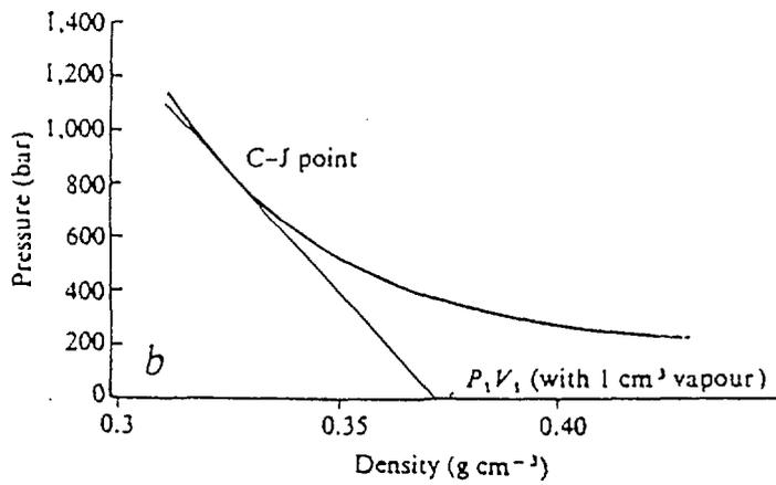
Fig 15. Schematic Shock Adiabatic: Solid Curve for Reacted Material and Dashed Curve for Unreacted Material.
