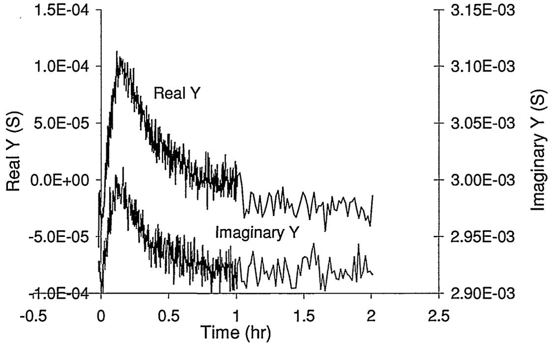
**Figure 15. Real and imaginary parts of admittance at 30 MHz.**
