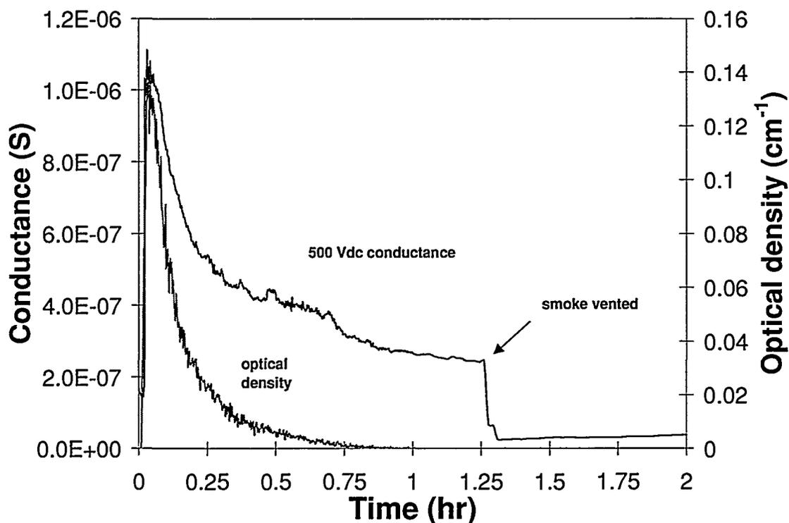
Figure 9. 500 Vdc Conductance and Optical density vs. time.
