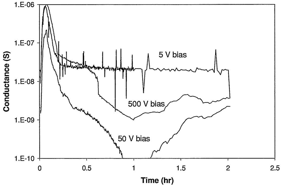
**Figure 20. Comparison of the conductance between boards with different bias voltages.**
