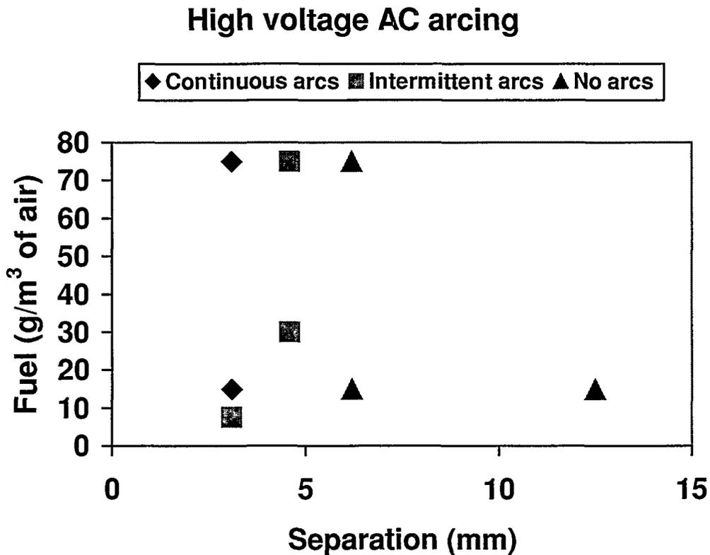
**Figure 16. Results of high voltage ac smoke tests.**
