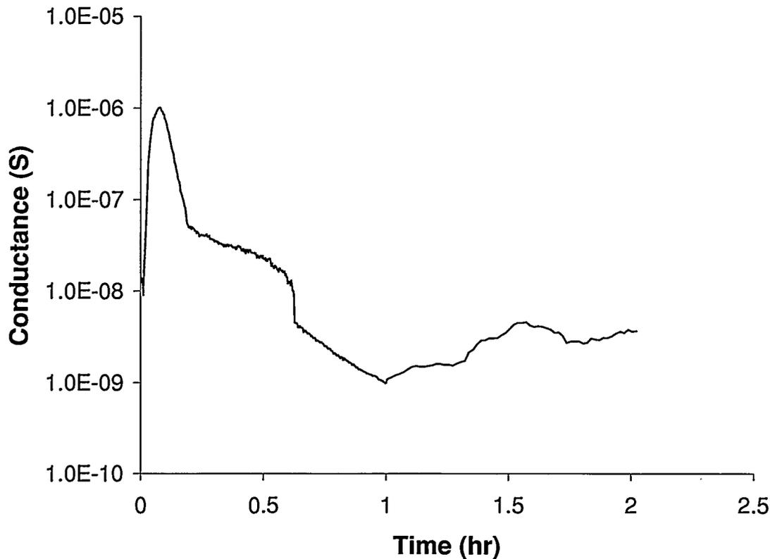
**Figure 25. The conductance of the 500-Vdc biased mass vs. conductivity board.**
