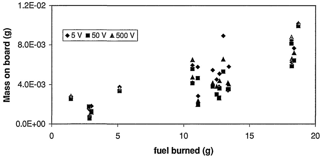
**Figure 21. Smoke collected by conductivity board vs. amount of fuel burned.**
