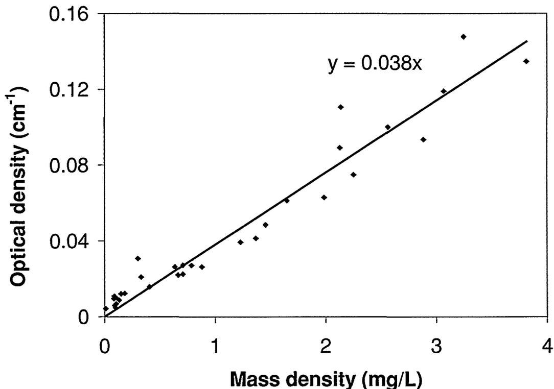
**Figure 8. Optical Density vs Mass density for PVC smoke.**
