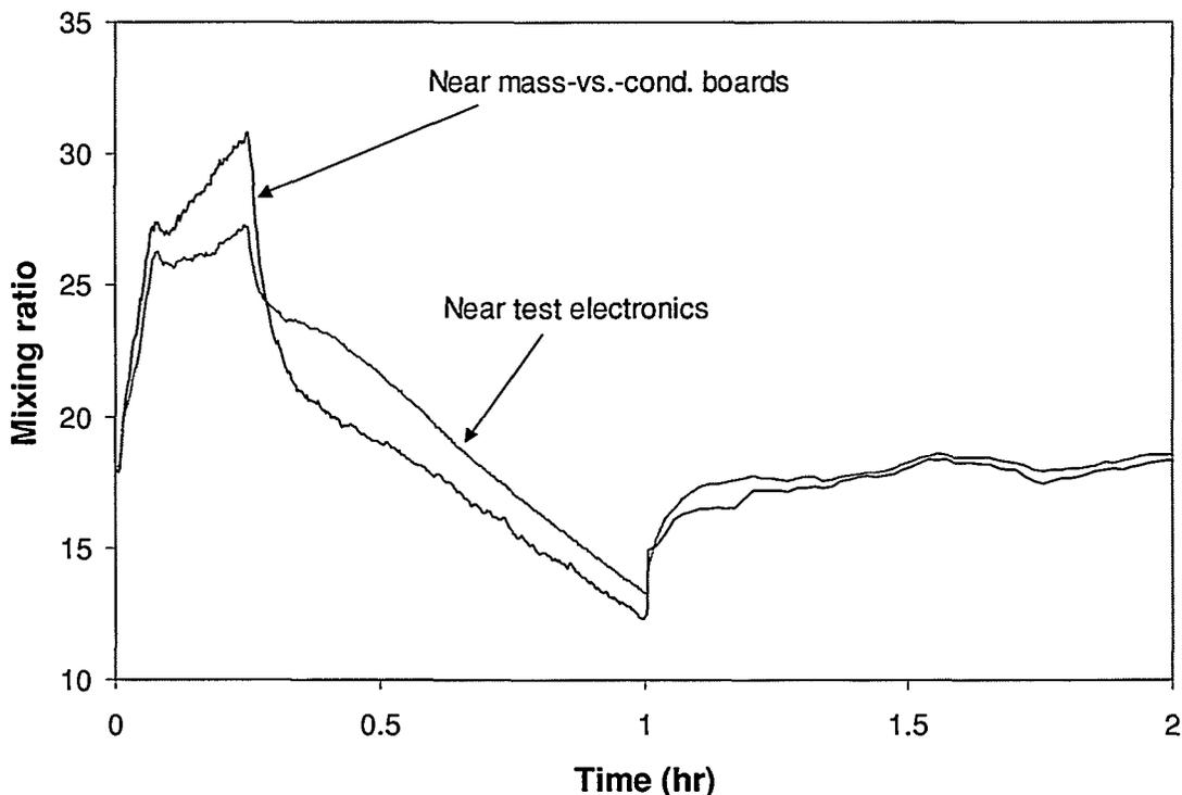
**Figure 24. Mixing ratio (g of H<sub>2</sub>O/kg air) during smoke test.**
