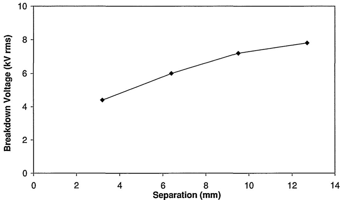
**Figure 17. Breakdown voltage vs. plate separation.**
