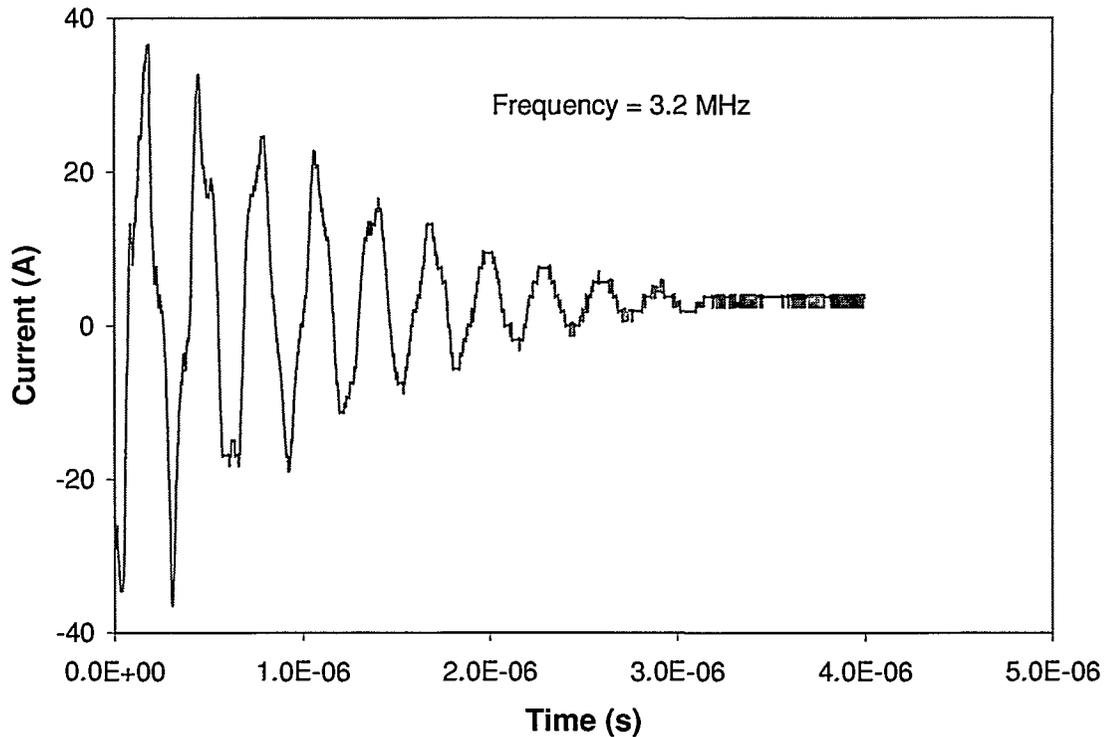
**Figure 18. High voltage AC leakage current.**
