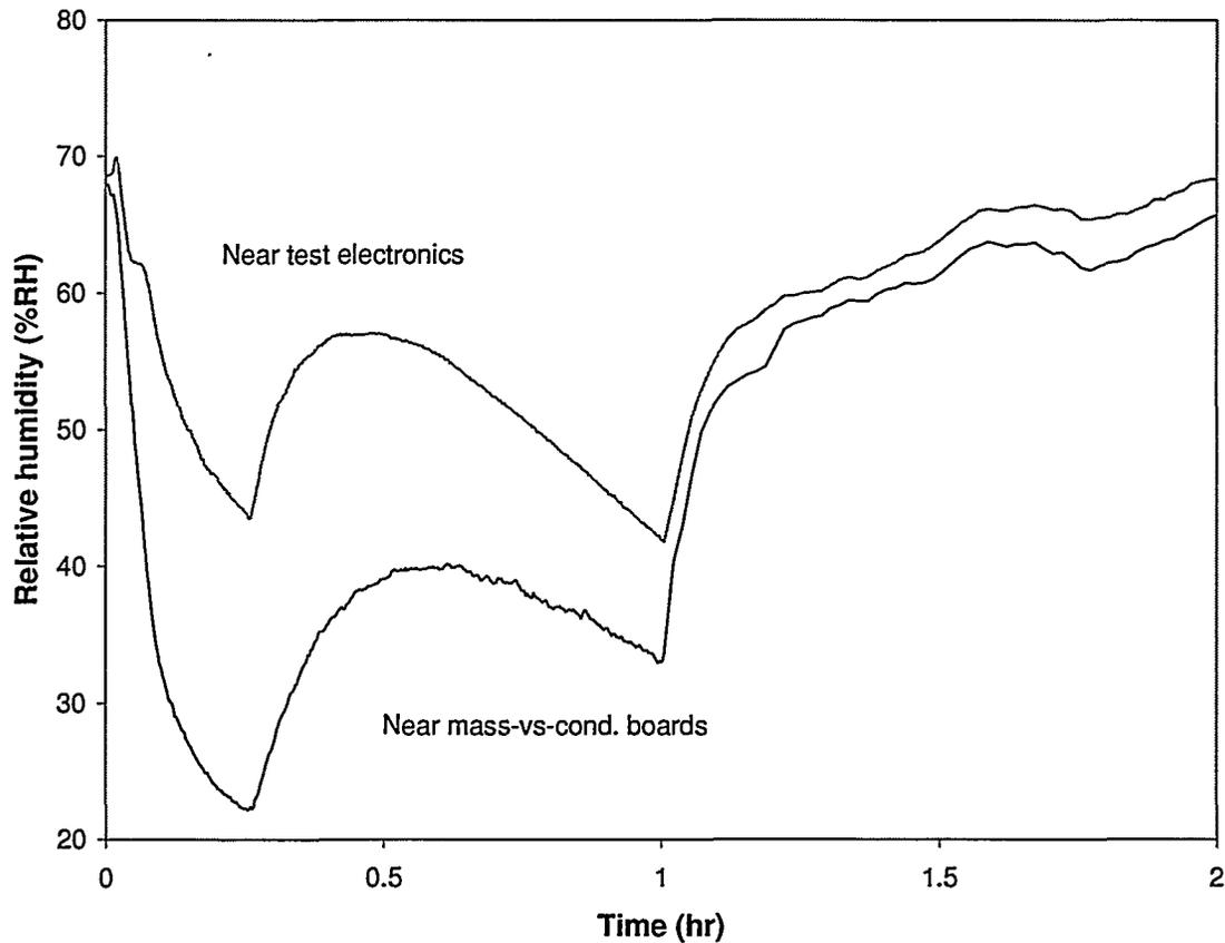
**Figure 23. Relative humidity in two locations in the smoke chamber.**
