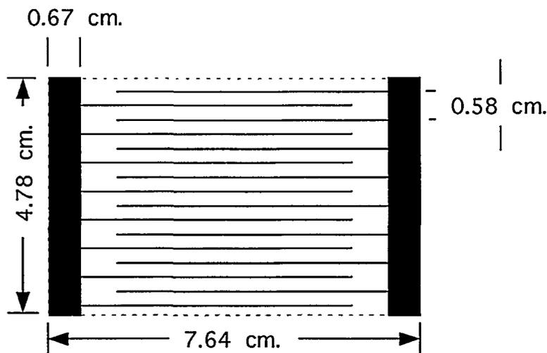
**Figure 5. Mass vs. conductivity board pattern.**
