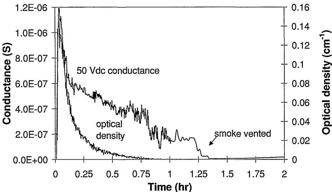
**Figure 14. 50 Vdc parallel plate conductance and optical density vs. time.**
