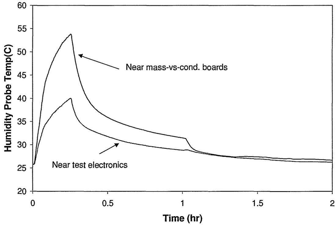
**Figure 22. Temperature of the humidity probes in the smoke exposure chamber.**
