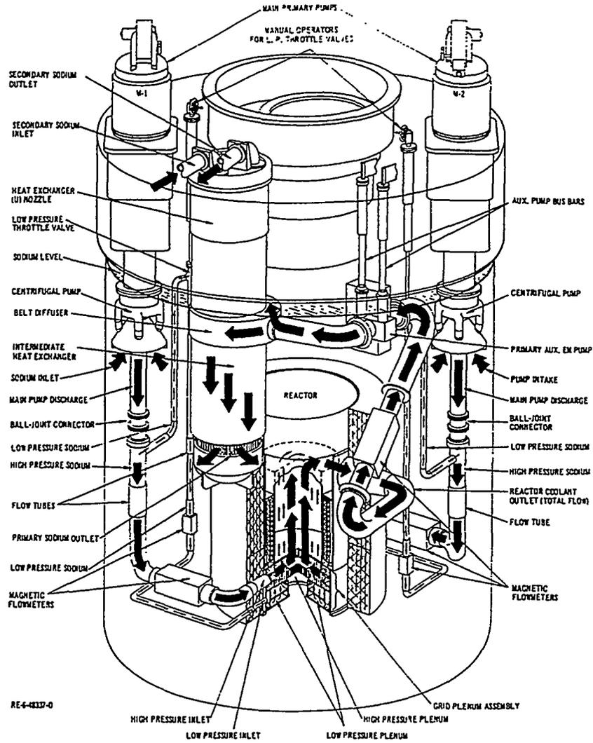
Figure 2. EBR-II Reactor Vessel
