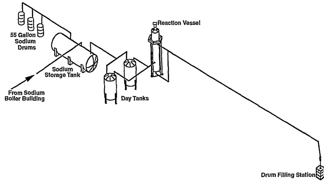
Figure 3. Sodium Process Facility Flow Diagram
