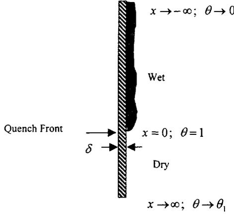
Figure 1 Schematic of top quenching of a single fuel rod
